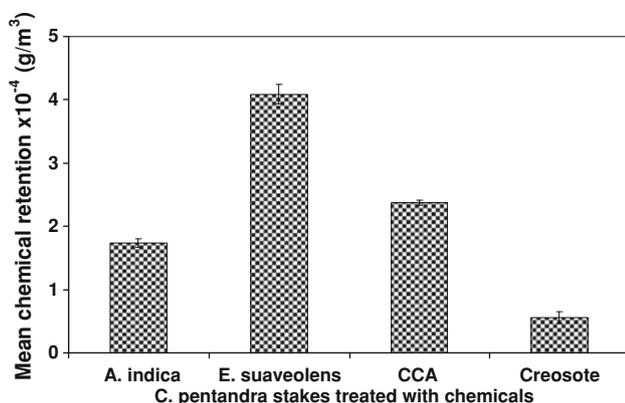
**Fig. 1** Chemical retention for *C. pentandra* treated stakes. Bars  $\pm$  SE ( $n = 10$ )
