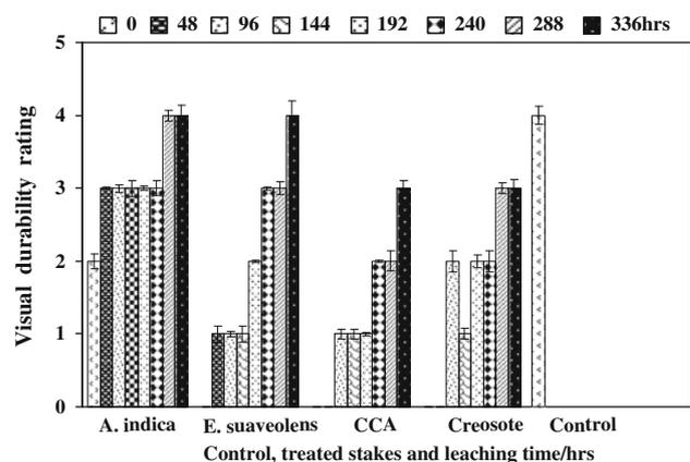
**Fig. 2** Visual durability ratings for *C. pentandra* treated stakes under different leaching periods. Bars  $\pm$  SE ( $n = 10$ )
