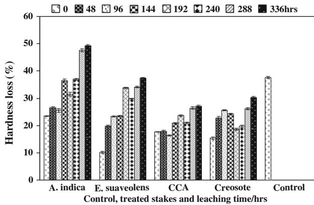
**Fig. 3** Hardness losses for *C. pentandra* treated stakes under different leaching periods. Bars  $\pm$  SE ( $n = 10$ )
