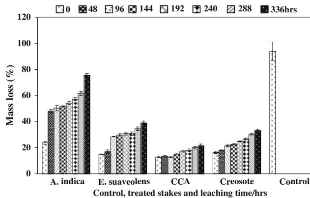
**Fig. 4** Mass losses for treated stakes under different leaching periods Science of the Total Environment Bars  $\pm$  SE ( $n = 10$ )
