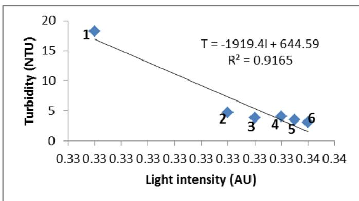
Fig.- 6: A graph of turbidity (NTU) as a function of transmitted light intensity (AU) for sample well water, (1) raw water, (2) filtrate (3) treated raw sample with 0.5g Zx, (4) treated raw sample with 0.2g Zx, (5)treated raw sample with 0.2g Zx, and (6) treated filtrate with 0.5g Zx.
