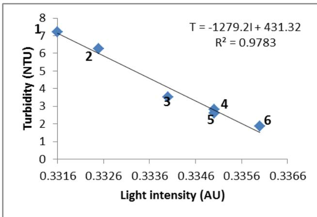
Fig-5: A graph of turbidity (NTU) as a function of transmitted light intensity (AU) for sample stream 2, (1) raw water, (2) filtrate, (3) treated raw sample with 0.5g ZX, (4) treated raw with 0.2g ZX, (5) treated filtrate with 0.5g ZX (5) treated raw sample with 0.2g ZX, and (6) treated filtrate with 0.2g ZX
