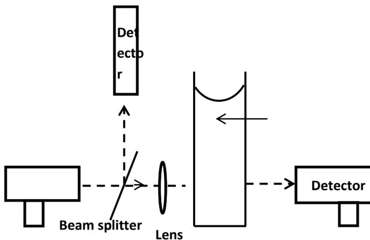
Fig -1: Experimental set up for the light transmission experiment
