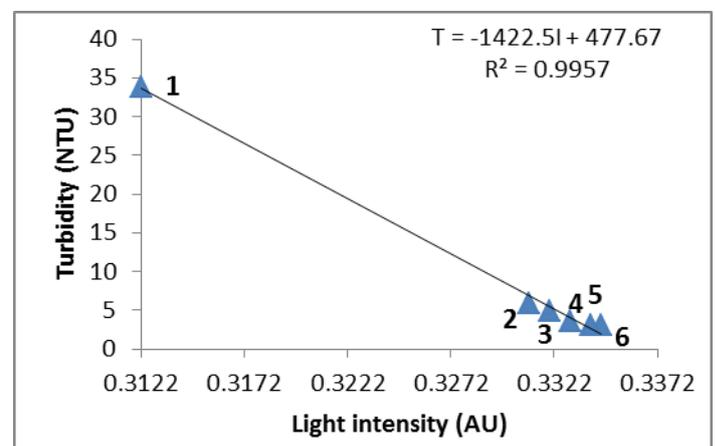
Fig.- 4: A graph of turbidity (NTU) as a function of transmitted light intensity (AU) for sample stream 1, (1) raw sample (2) filtrate, (3) treated raw sample with 0.5gZX, (4) treated raw sample with 0.2g ZX, (5) treated raw sample with 0.2g ZX, and (6) treated filtrate with 0.5g ZX.
