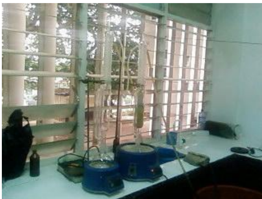
Fig. 3.2: A picture of Soxhlet apparatus during an extraction
