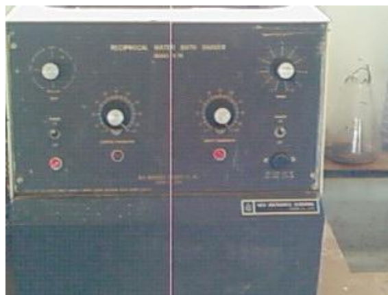
Fig. 3.5: A picture of New Brunswick Scientific (Edison N.J. USA) reciprocal water bath shaker model R76
