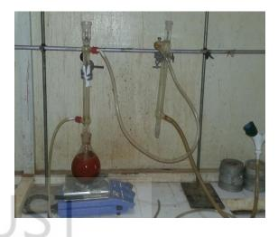
Plate 6 Bauxite waste in a refluxing set up before digestion
