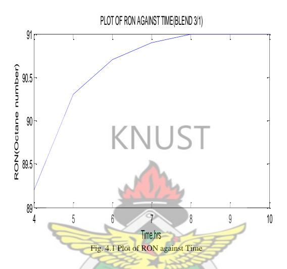
The fig. 4.1 above is a blend of tank 3 against 1 and it displays a plot of RON against time in hours. The RON is 89.2 after 4hours of mixing. At 5 hours of mixing the RON is 90.3, at 6hours 90.7 and 7hours 90.9. After 8hours of mixing the RON is 91 and stays constant at 91 till 10hours of mixing.
