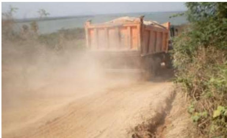
***Figure 2.7 Dust generated on a haul road (source: Personal Collection)***
