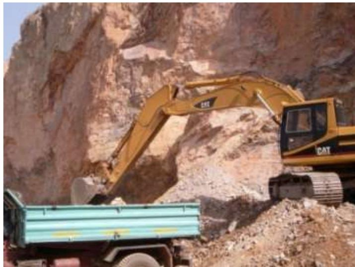
*Figure2.5 A dry pit gravel extraction operation (source: Personal Collection)*
