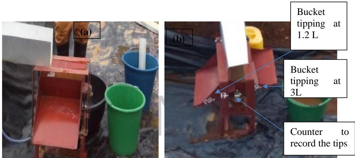
**Plate 4.3 (a). Seasonal calibration to determine the tipping volume of each bucket. (b)Tipping bucket devices installed at the end of a runoff plot with the counter and the tipping volume of each bucket: 1.20 L and 3 L**
