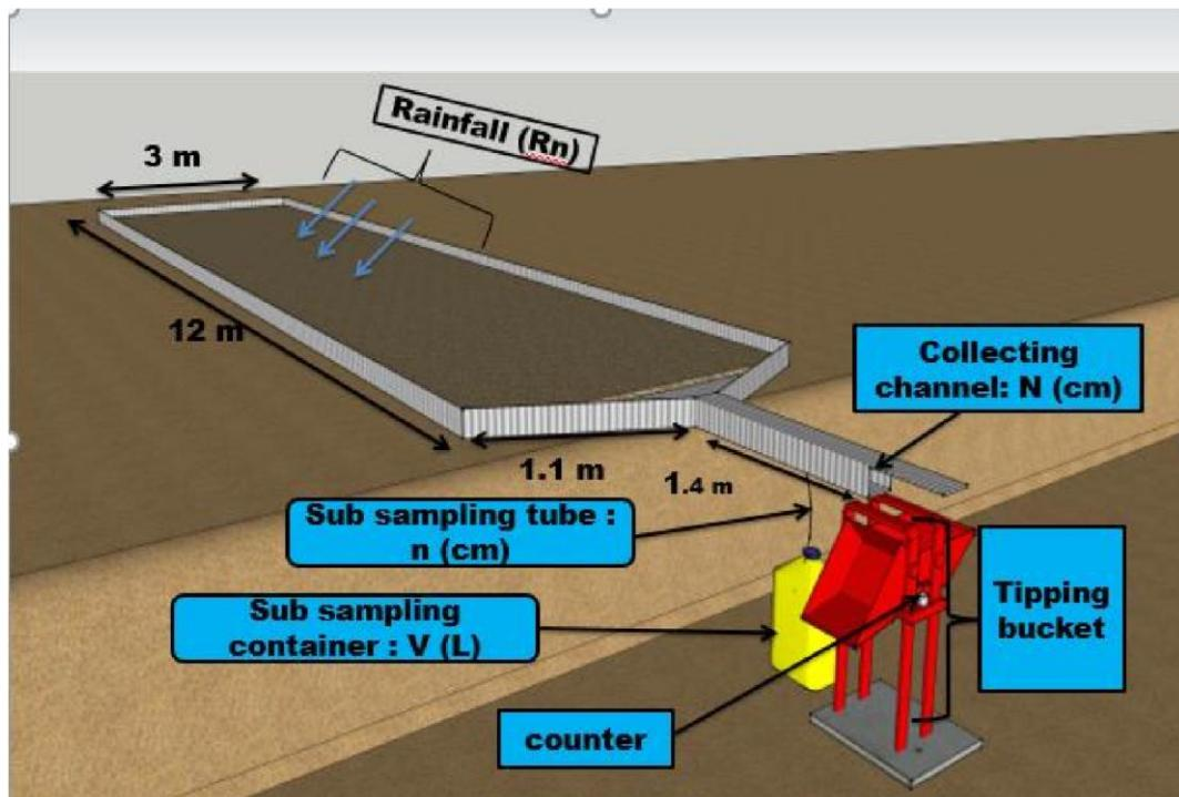
**Plate 4.1. Layout of runoff plot with the tipping bucket device for runoff and soil erosion assessment**
