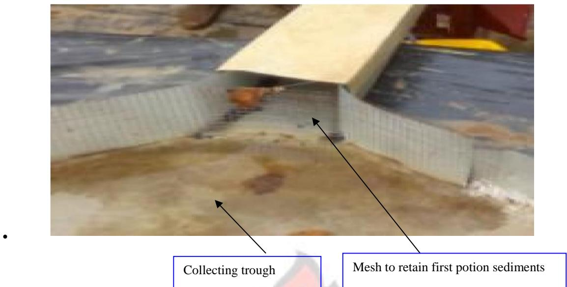
**Plate 4.2. Collecting trough with aluzinc sheet at the end of each runoff plot and the mesh fixed between the channel and the collecting trough to retain the first portion of the runoff loads**
