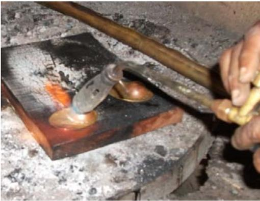
Plate 3.19 – soldering the dome and oval
