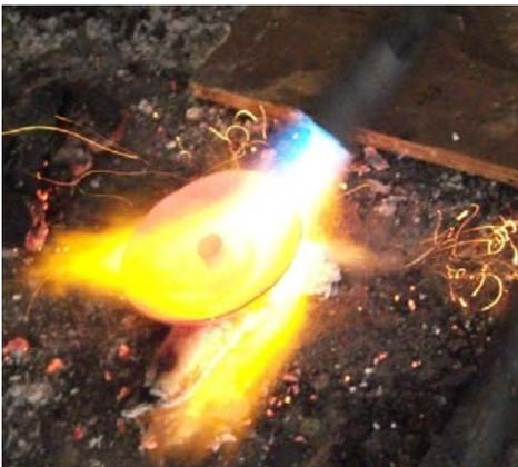
Plate 3.14 – soldering the seat into bowl
