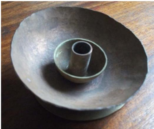
Plate 3.18- all parts of the base soldered together
