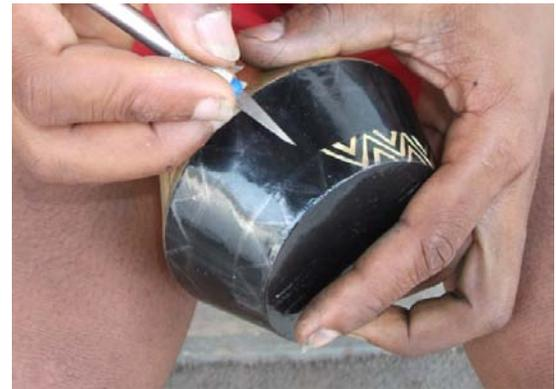
Plate 3.67 – Cutting out the design with a knife
