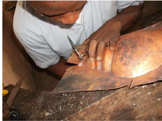
Plate 3.51 – Piercing off excess metal
