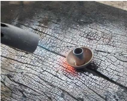
Plate – 3.13- soldering the copper tube into the dome.
