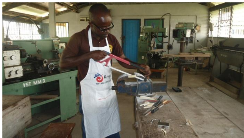
Plate 3.13: Cutting the bone with hacksaw tightly held with a vise
