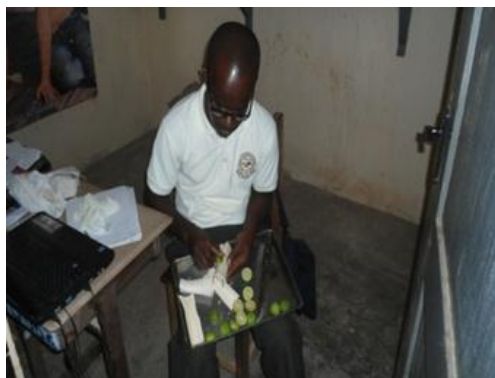
Plate 3.7: Deflecting and degreasing the bone. Plate 3.8: Application of lime to bone for removal of unpleasant smell and bleaching of bone.
