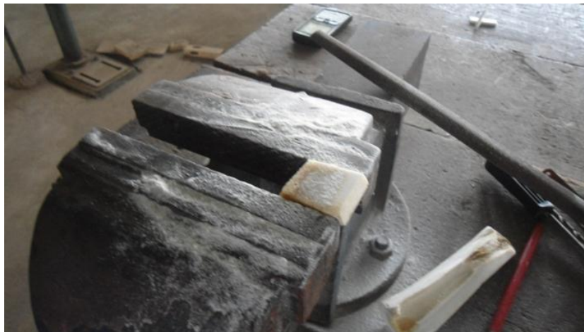
Plate 3.12: the bone held tightly with vise and filed into desired shape
