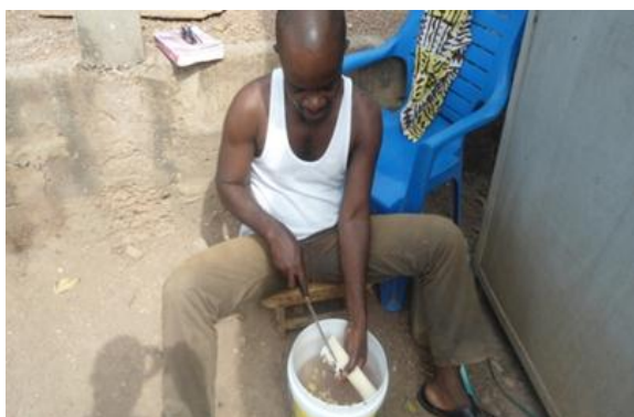
Plate 3.7: Deflecting and degreasing the bone. Plate 3.8: Application of lime to bone for removal of unpleasant smell and bleaching of bone.
