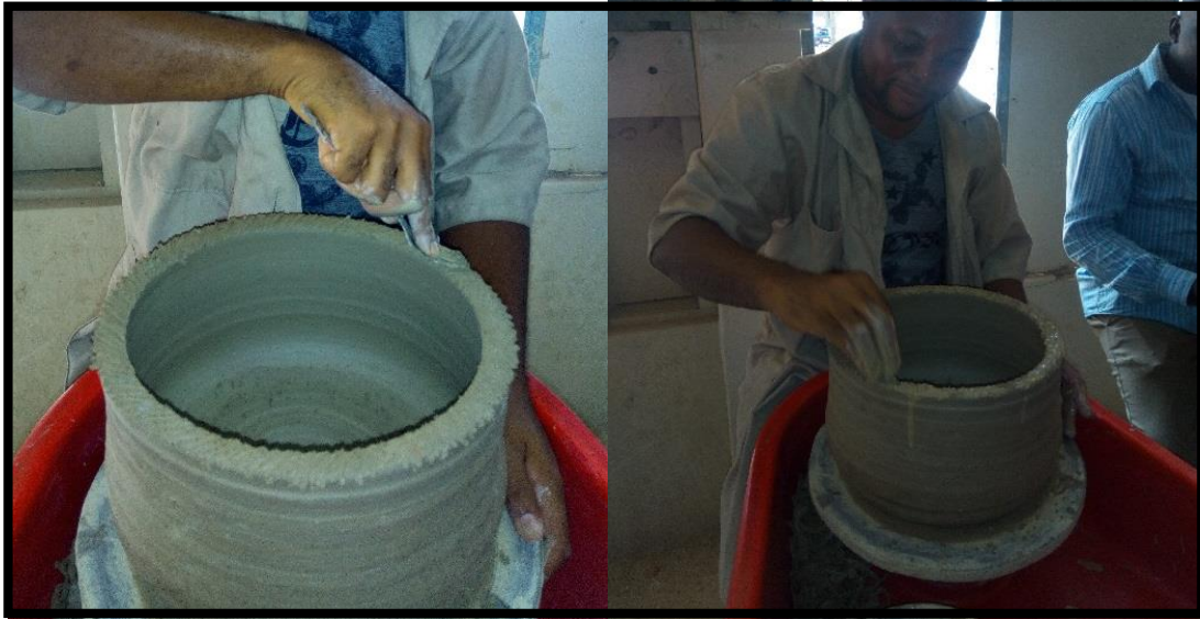
plate 3.16: application of slip prior to joining
