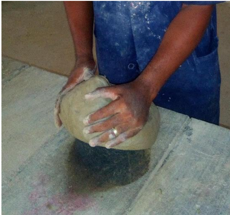
Plate 3.11: proper opening to remove air pockets and impurities
