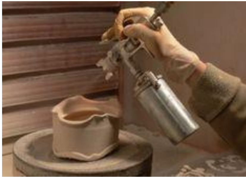
Plate 2.17: glaze application by spraying (Source: www.pinterest.com )
