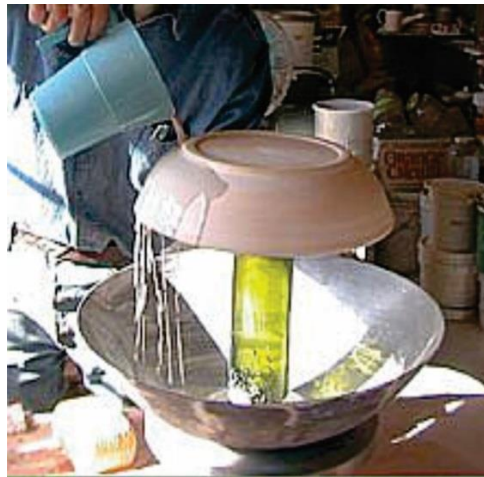
Plate 2.15: pouring technique of glaze application (Source: www.pinterest.com )
