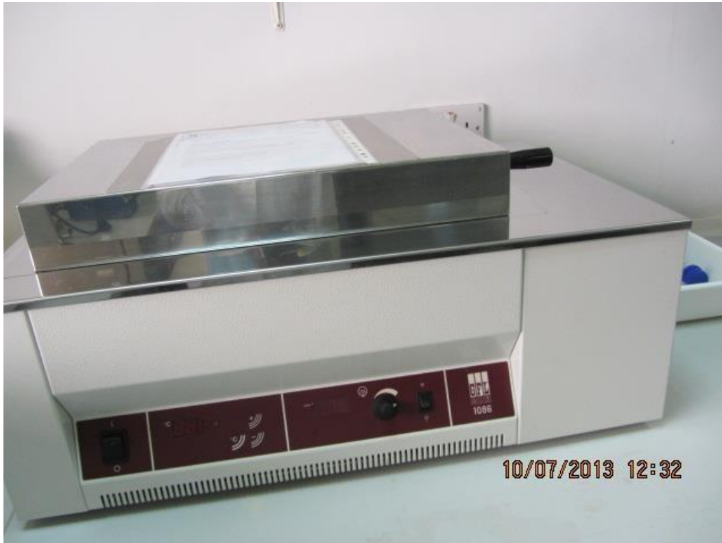
Water bath used to keep prepared agar at constant temperature
