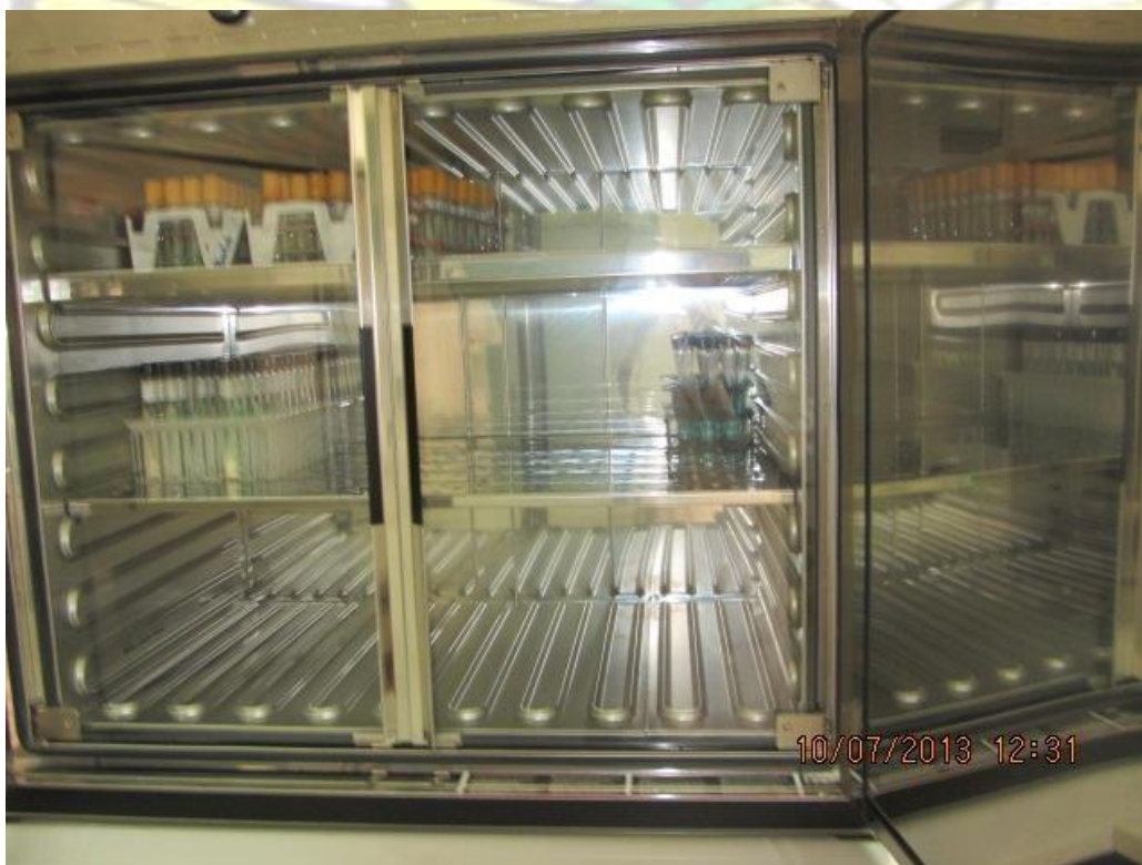
Incubator used in the study to dry agar plates
