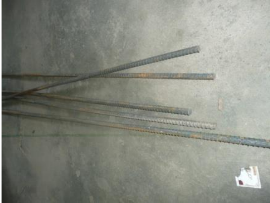
Fig. 3.10:steel (or iron) rods (12mm)
