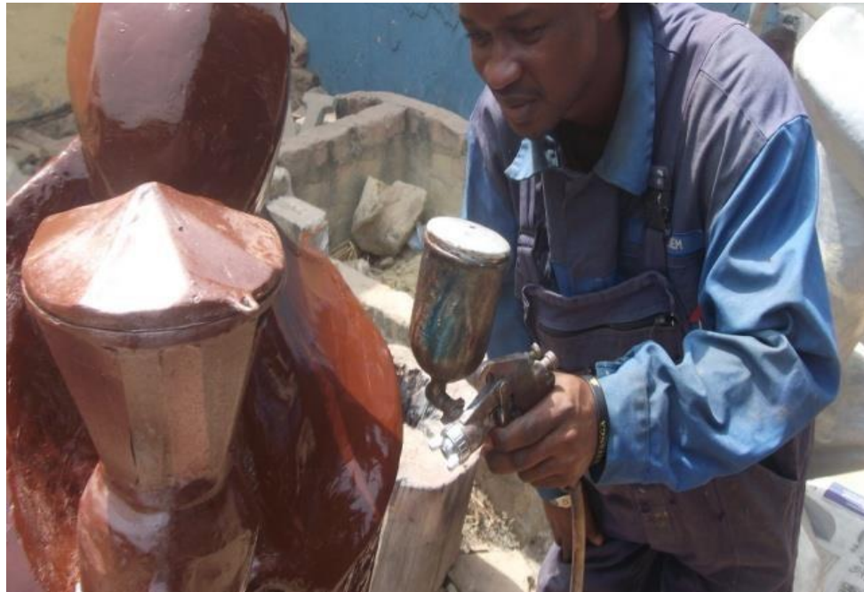
Fig. 3.87: spraying the body
