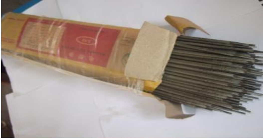
Fig. 3.15: A packet of 2.5mm electrodes
