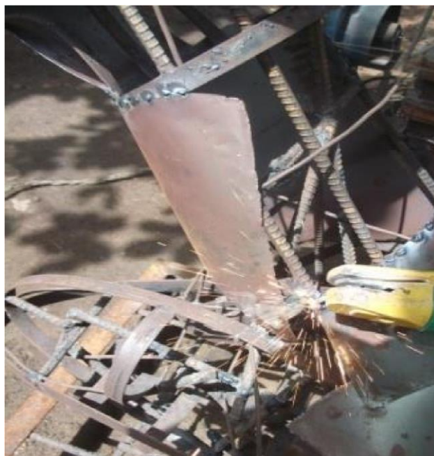
Fig. 3.95: welding the lower part of the stomach
