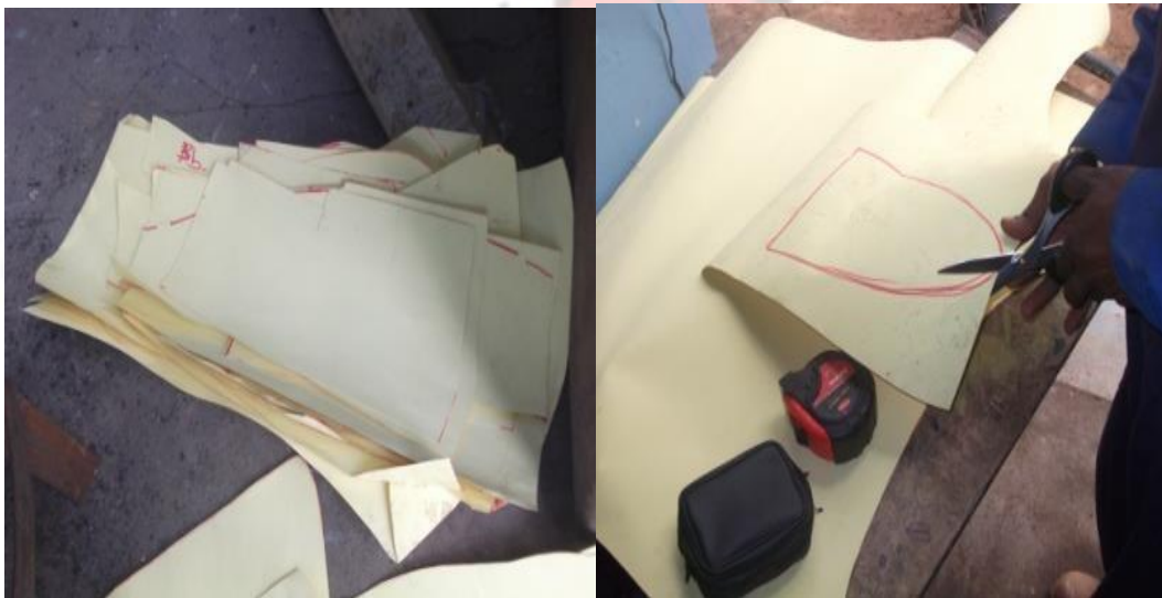
Fig. 3.61: some manila card patterns Fig. 3.62: using a pair of scissors to cut out a pattern
