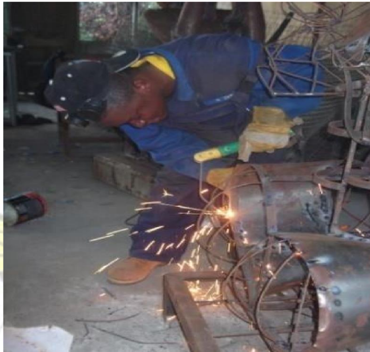
Fig. 3.69: Tack-welding the thighs
