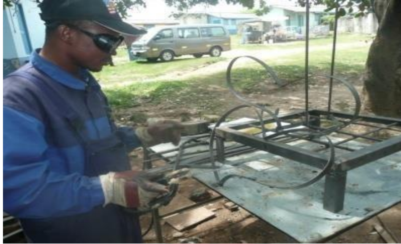
Fig 3.52 shows the welding of the fabricated heart shapes being welded onto the base of the armature.
