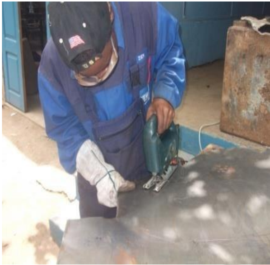
Fig. 3.63: cutting a template with a Jigsaw
