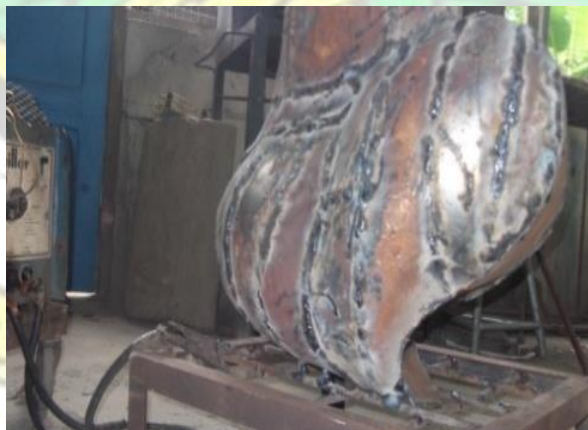
Fig. 3.71: the complete back part of the heart shape which also serves as the buttocks of the statue.
