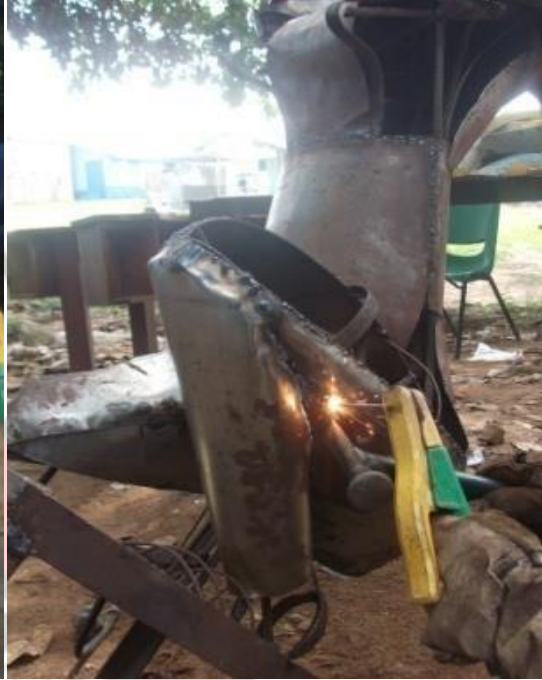
Fig. 3.100: forming and joining the thigh.
