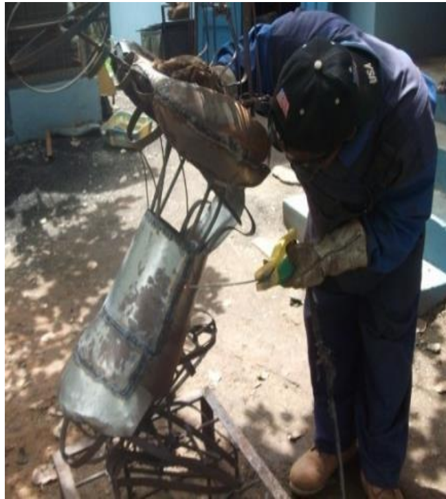
Fig.3.96: welding the back of the figure with overlapped the templates.
