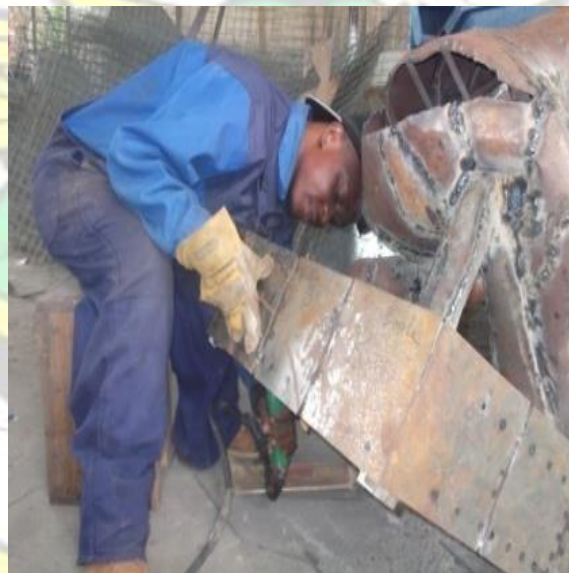
Fig. 3.108: welding the metal tiles from the outside
