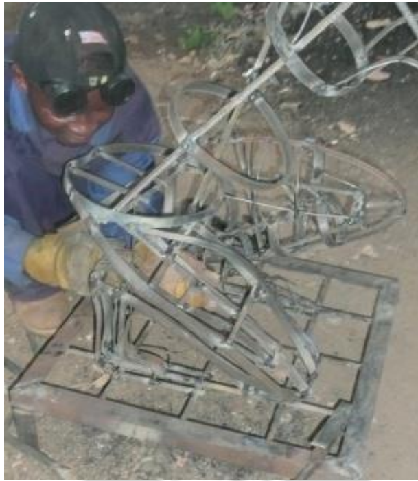
Fig. 3.91: Joining rings to the attachment
