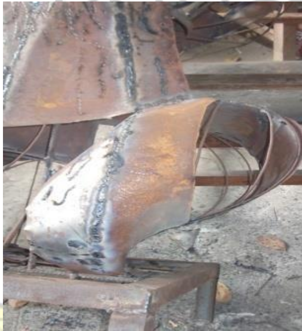
Fig. 3.70: Fabrication and welding of the heart shape
