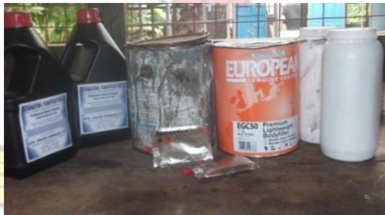
Fig. 3.110: from left to right are turpentine, primer, hardeners, filler and paints in the white plastic containers.
