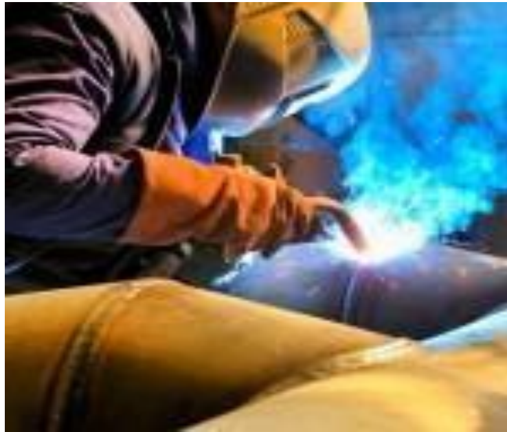
Fig 2.1: GMAW or Gas Metal Arc Welding process
