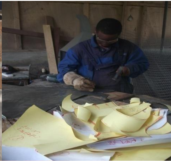
Fig. 3.64: cutting a template with chisel and hammer
