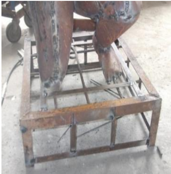
Fig. 3.107: Creating attachments for the welding of metal tiles
