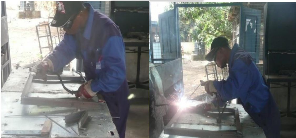
Fig. 3.48: shows the tack-welding of the angle bars to form the top square component of the platform
