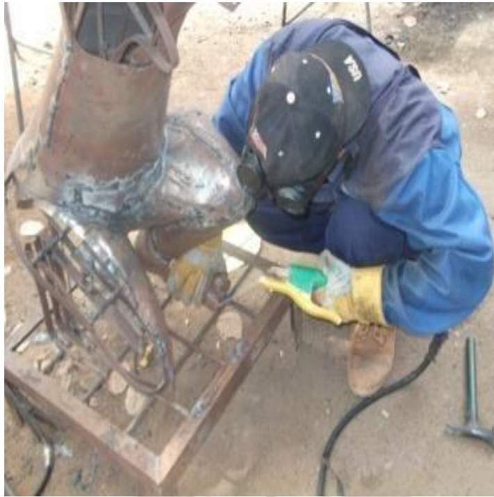
Fig. 3.101: Attaching the feet to the platform, or the base.
