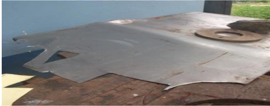
Fig. 3.13: a section of 1mm steel sheet and another 1mm sheet from which templates were being cut.
