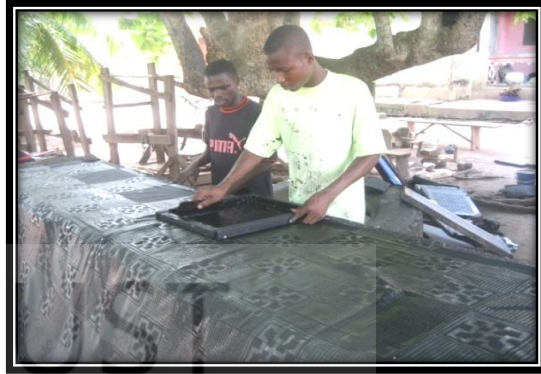
Plate. 4.9. Screen printing (modern) method of adinkra printing
