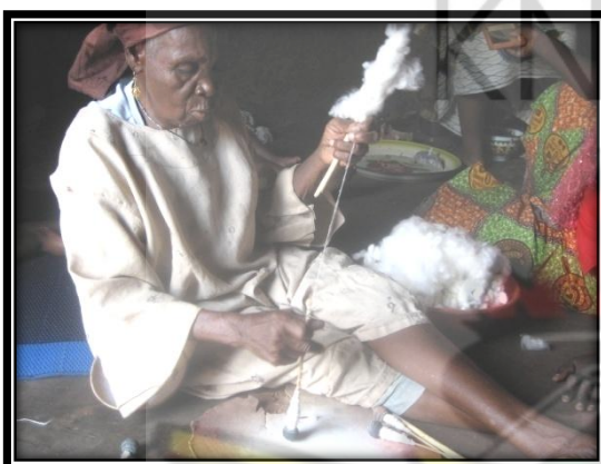
Plate. 4.36. Spinning of cotton aided by the revolving spindle and the right hand.
