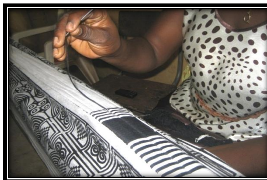
Plate. 4.12. Faggoting technique in the production of “nwomu” cloth
