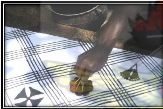
Plate. 4.10. Hand stamping (traditional) method of adinkra printing
