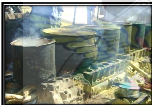
Plate. 4.18. Initial boiling of dye liquor in series of chambers
