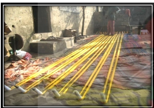
Plate. 4. 81. Warp laying round pegs on the ground
