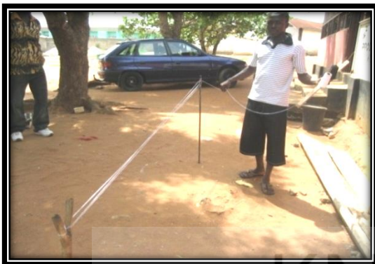
Plate. 4.79. Laying warp between two upright posts (“ntomatene”)
