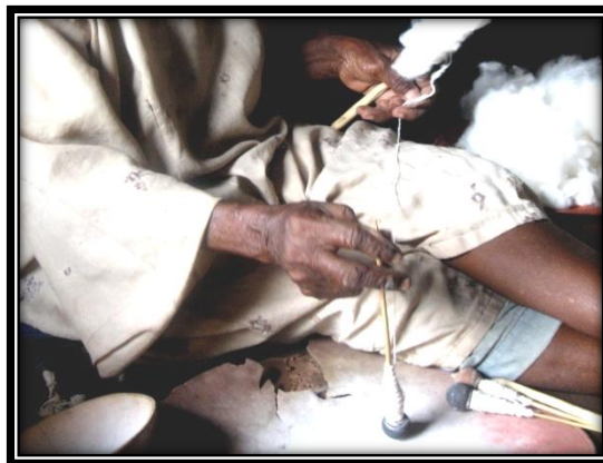
Plate. 4.35. Setting the spindle revolving
