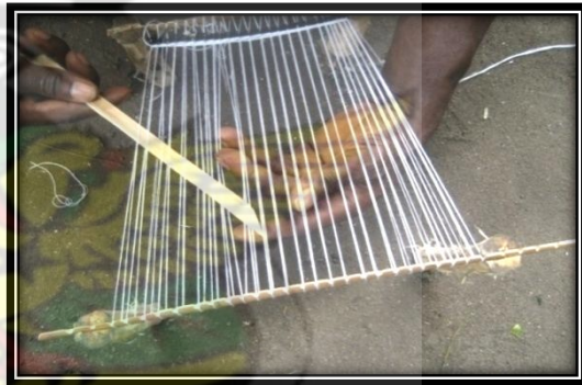
Plate. 4.67. Opening up the warps in alternating order using a palm leaf accessory
