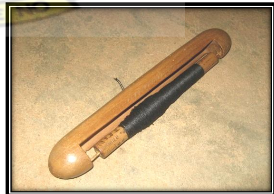
Plate. 4.89. Shuttle loaded with weft for weaving
