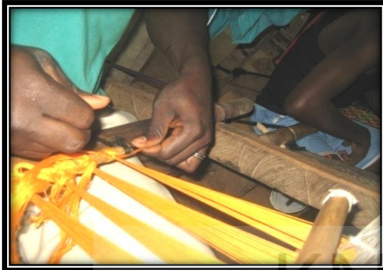
Plate. 4.86. Tying warp yarns to cloth roller.
