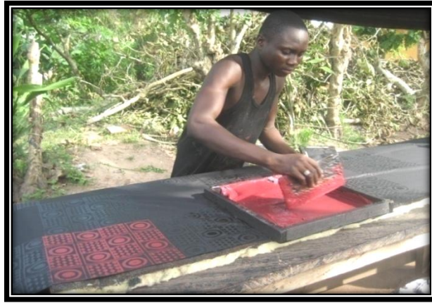
Plate. 4.24. Screen printing adinkra patterns unto cloth
