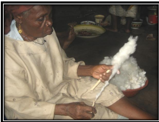
Plate. 4.34. Attaching a strand of cotton onto the spindle
