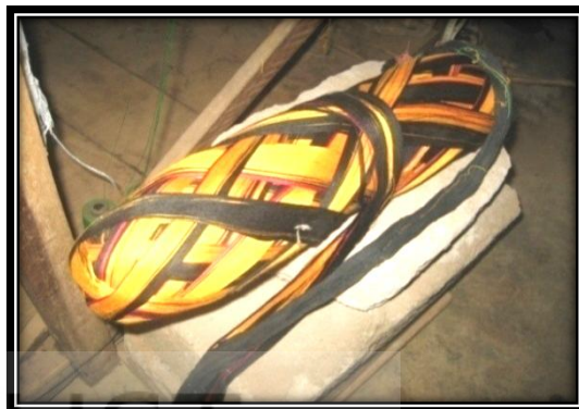
Plate.4.80. Wound warp after warping (Ashanti “bobo”)
