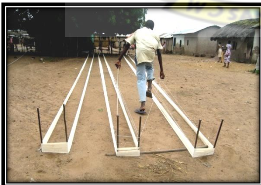
Plate. 4.44. Warping yarns prior to dyeing
