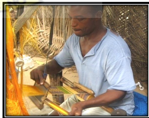
Plate. 4.93. Beating-up the newly inserted wefts together (beating –up)
