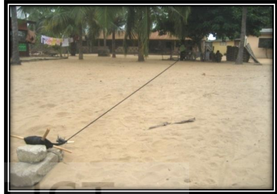
Plate. 4.87. Stretched warp yarns to ensure even tension in warp during weaving
