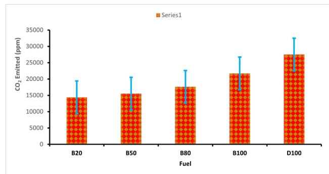
Figure 6. Carbon (IV) oxide emission of different blends
