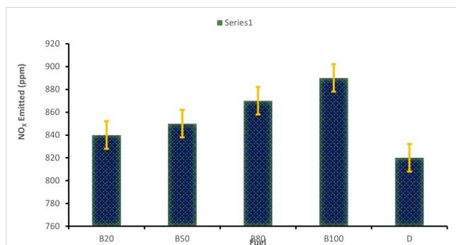
Figure 7. NO<sub>x</sub> emission of different blends
