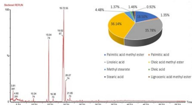
**Figure 1.** The GC-MS Chromatogram of WCO-derived biodiesel
