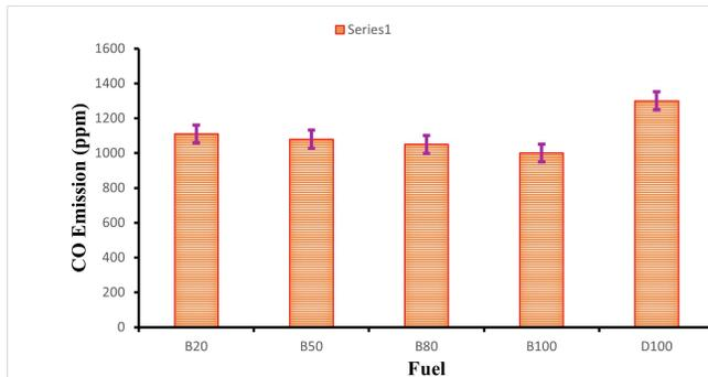
Figure 3. Carbon (II) oxide emission of different blend
