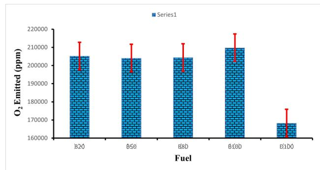
Figure 5. Oxygen emission of different blends
