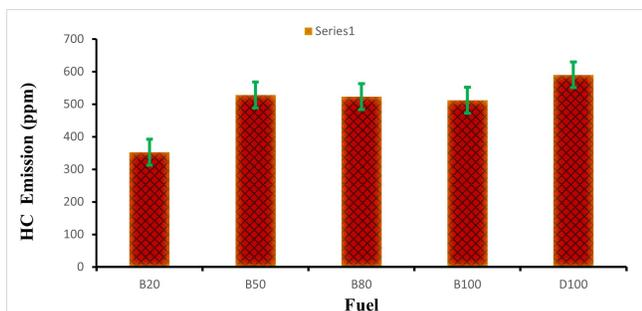
Figure 4. UHC emission of different blends
