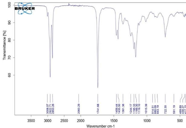
**Figure 2.** FTIR Spectra of WCO-derived biodiesel
