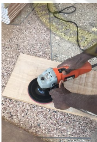
Plate 3.11d: The support was sanded, glued and fixed with nail to the Map frame
