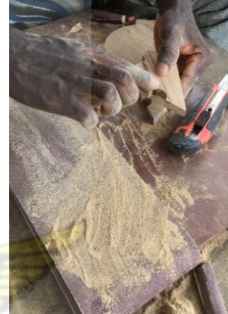
Plate 3.8d: Sawdust and Superglue were mixed to fill the cracks in the wood
