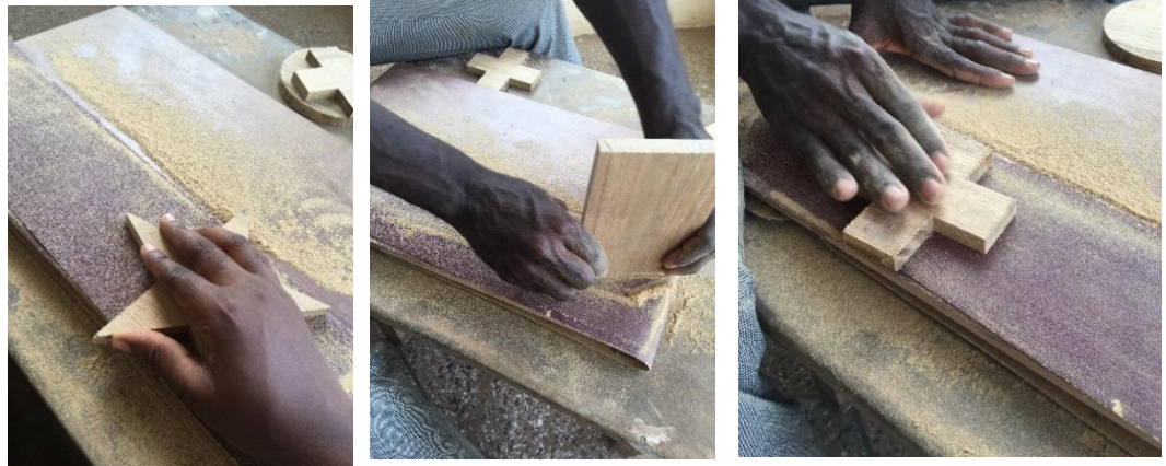
Plate 3.9c: Sanding the cut-out shapes to make them smooth
