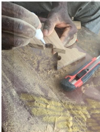
Plate 3.8d: Sawdust and Superglue were mixed to fill the cracks in the wood
