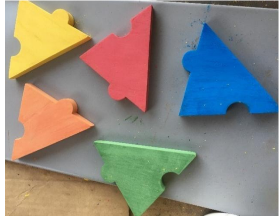
Plate 3.8f: The work was sanded, painted and left to dry three times before lacquer was applied on them
