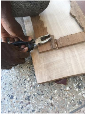
Plate 3.11e: Nail heads clipped, concealed with punch and edges trimmed
