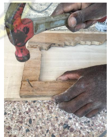
Plate 3.11d: The support was sanded, glued and fixed with nail to the Map frame
