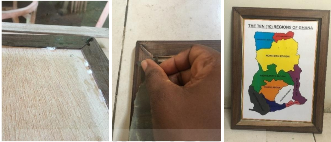
Plate 3.11o: Chamfered wood glued to plywood and sanded to complete work
