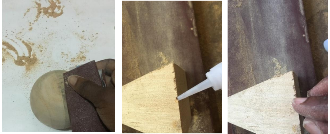
Plate3.10e: Wood sanded, holes sealed with sawdust and superglue
