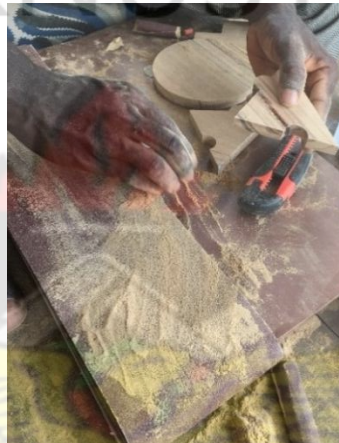
Plate 3.8d: Sawdust and Superglue were mixed to fill the cracks in the wood
