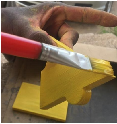
Plate 3.8f: The work was sanded, painted and left to dry three times before lacquer was applied on them
