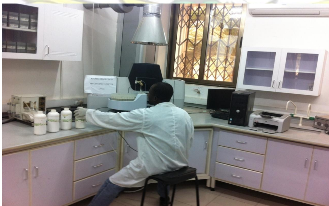
Plate K: Analysis of Heavy metal by AAS
