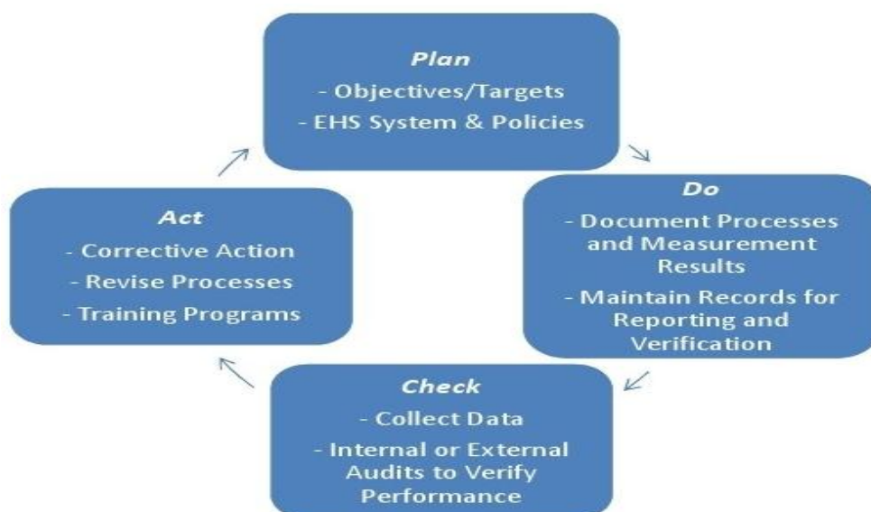
Figure 2.5: A Generic Plan-do-check-act Model Applied to record-keeping
