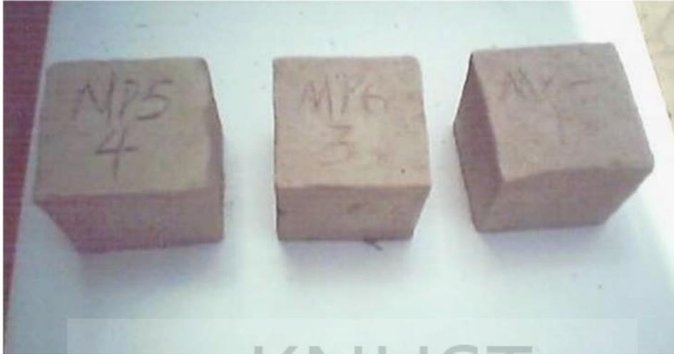
Figure 5.43 Test pieces made with Mfensi clay with 5% lime plus 5%, 10% and 15% PBA after two years exposure for two years. (Maintained shape)
