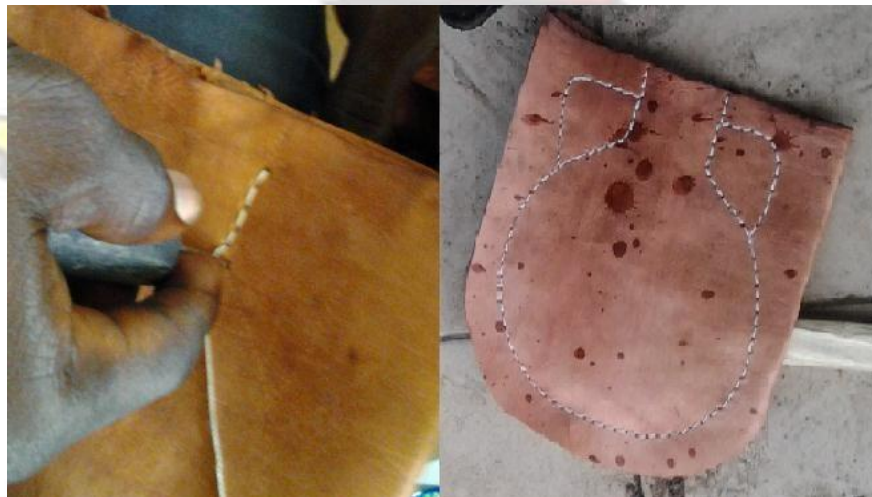
Plate 3. 4: With the Help of an Awl Stitching on the Drawn Pattern
