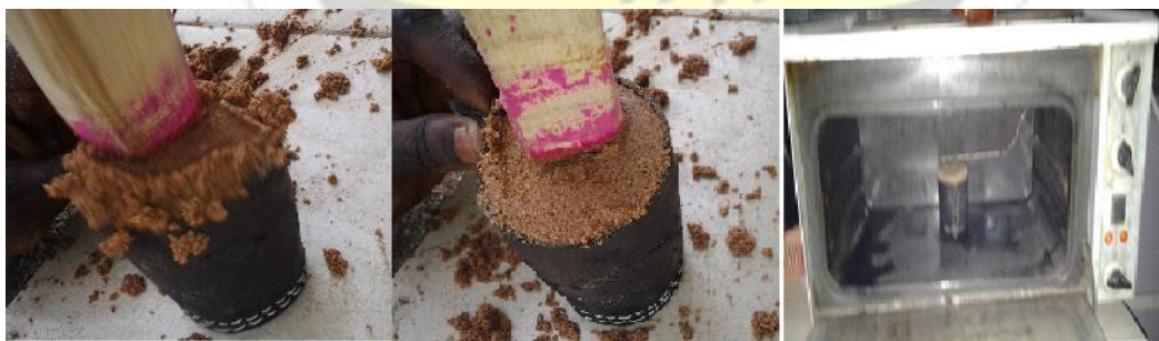
Plate 3.11: Sand is packed in the stitched vessel and baked in an electric oven
