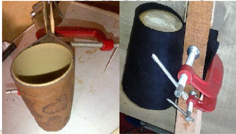
Plate 3.7: Leather wrapped around a carved wooden log with a G-clamp
