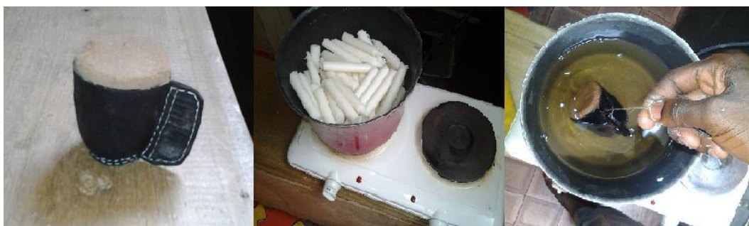
Plate 3.12: After baking the vessel, put the baked vessel in a melting wax
