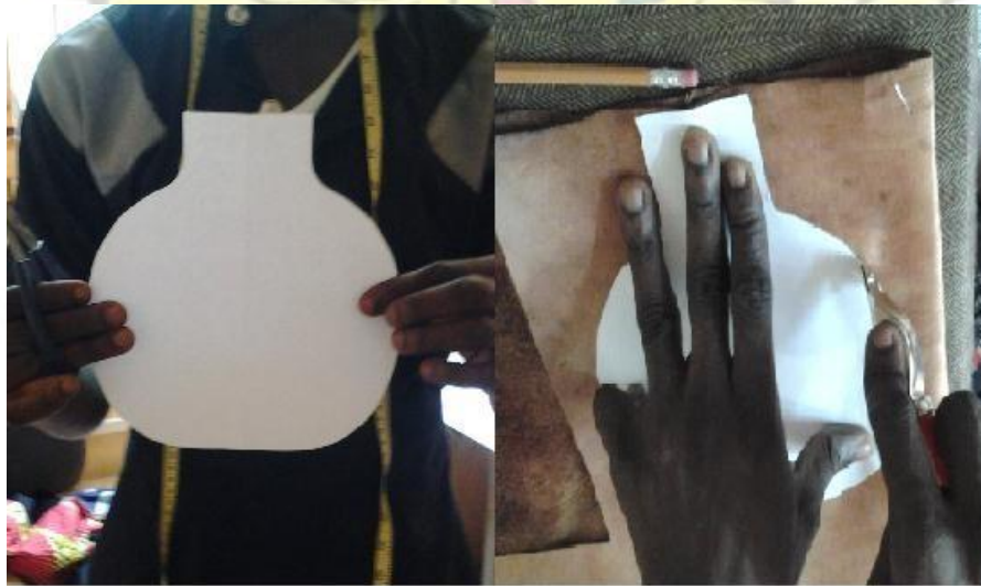
Plate 3.3: Making and transferring the pattern of the leather bottle
