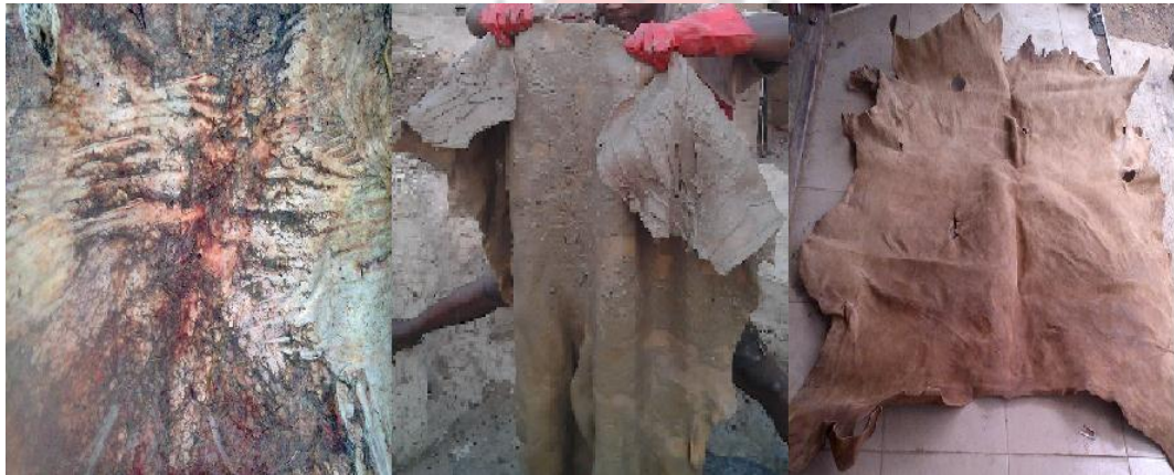
Plate 3.1: Pelt put in a pit with some small degree of acidity and salinity to obtain the leather (hide)
