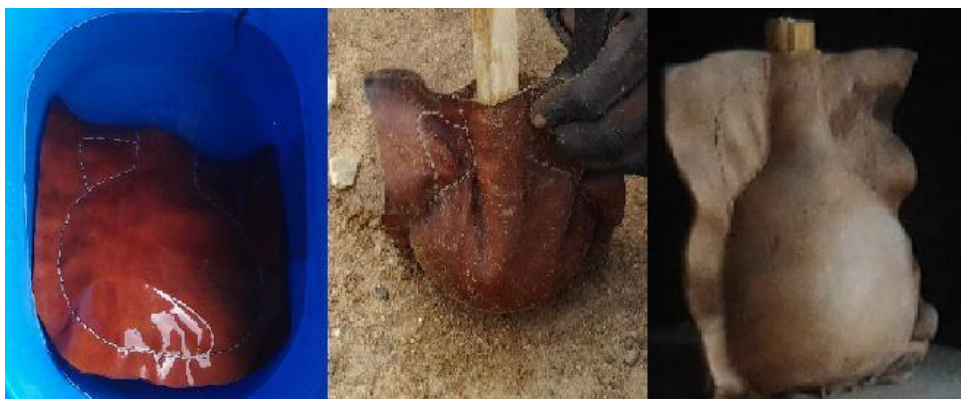
Plate 3. 5: The sawn leather soaked in warm water and sand being filled with it to bring the shape
