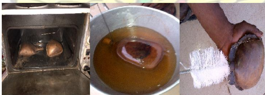
Plate 3.6: Baking the vessel; immersing the baked vessel in melting wax and washing the interior of the waxed vessel
