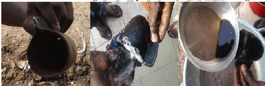
Plate 3.12: After baking the vessel, put the baked vessel in a melting wax
