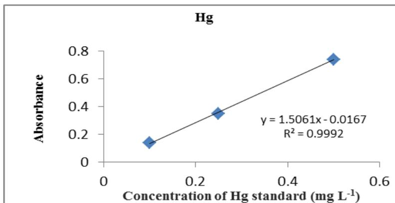
**Fig 3.3** Linear regression line for the calibration of the CV-AAS method for Hg determination
