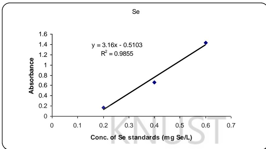
**Fig 3.2** Linear regression line for the calibration of the HG-AAS method for Se determination
