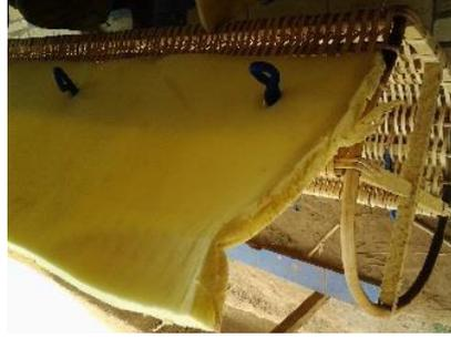
Plate 5.3h and 5.3i: Application of foam to the woven palanquin
