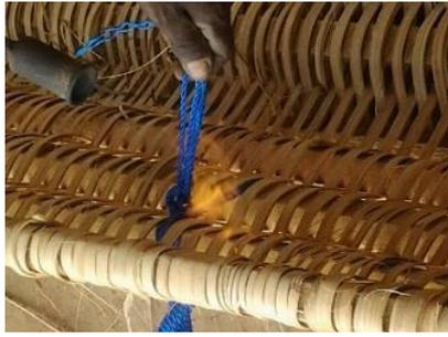
Plate 5.3g: Fixing of the handles
