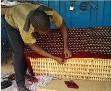
Plate 5.3j and 5.3k: Application of printed fabric
