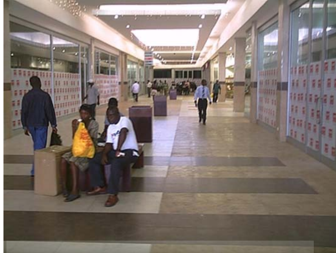
Fig.4.16. Dull floor tiles to camouflage stains in ASM space
