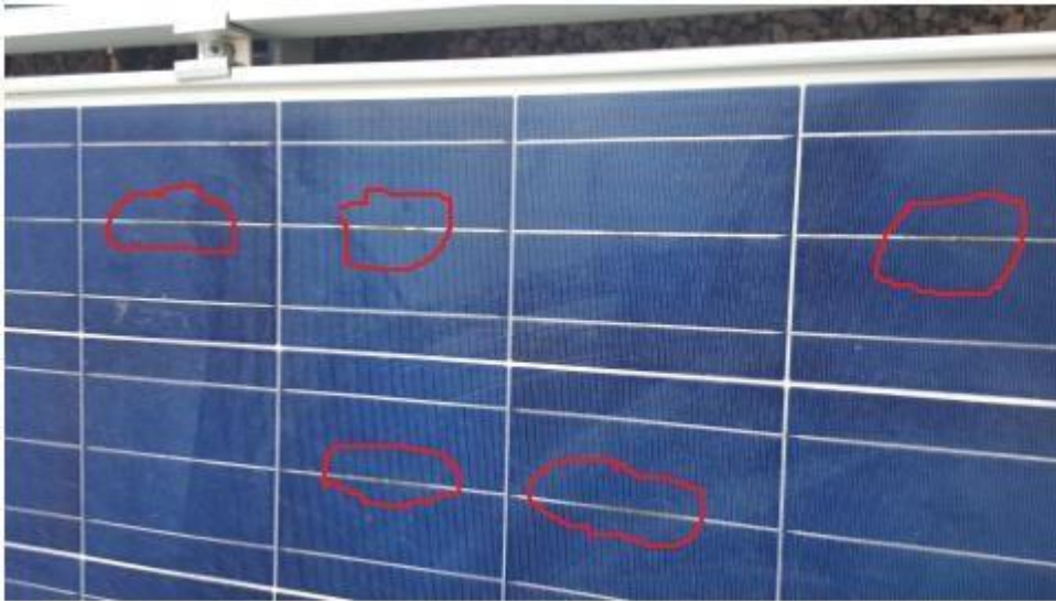
Snail crack propagating on module
