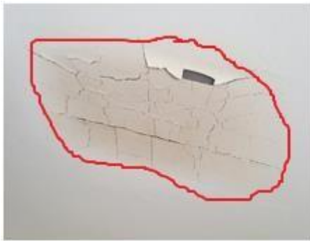
Back sheet delamination leading to cracks
