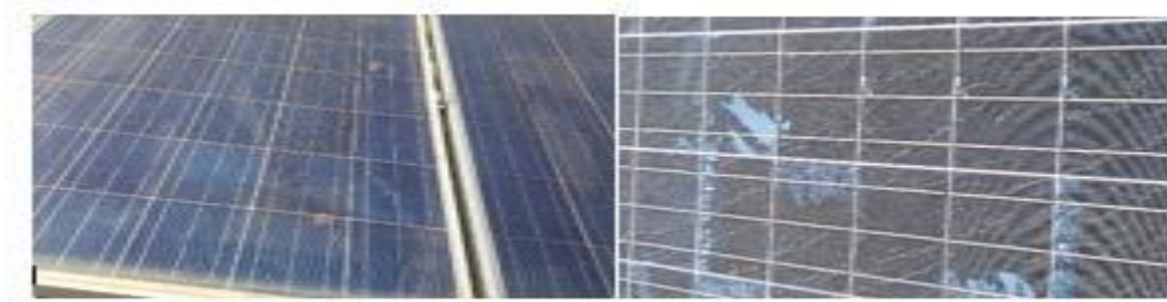
Plate 4- 4: front glass slightly soiled
