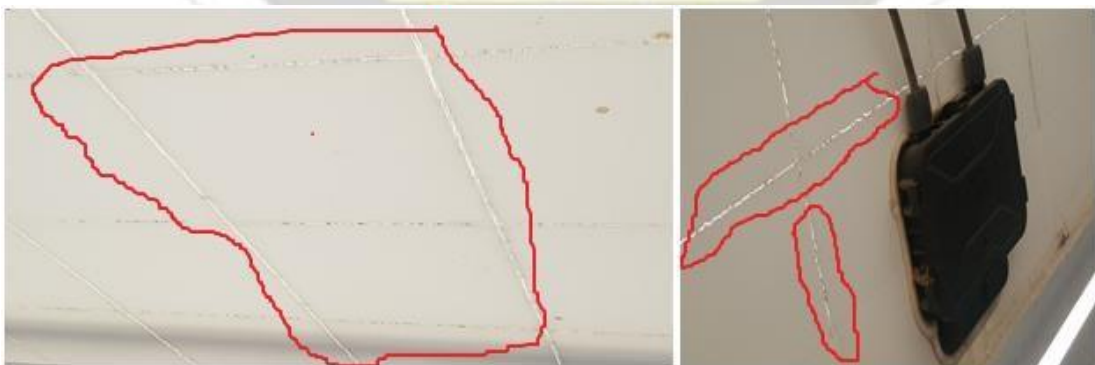
Plate 4- 2: cell cracks/ cell snail tracks
