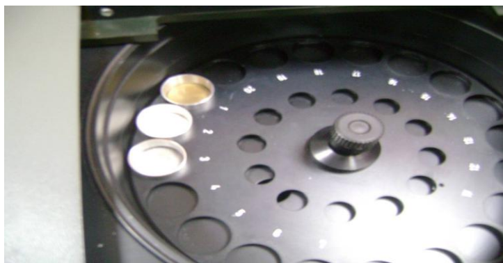
Figure 3.2: Placing the Pellets into the X-ray Fluorescence machine
