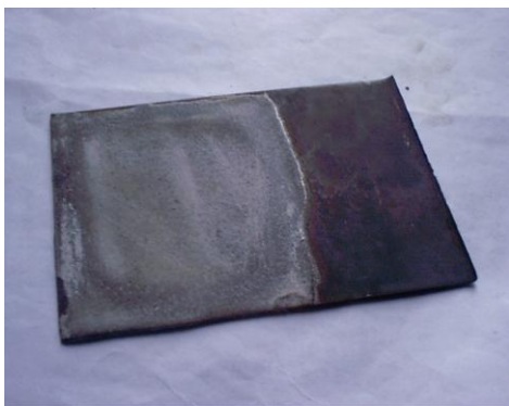
Figure 4.9: A picture of test piece prepared with FMB 10:1:5 fired at 800°C
