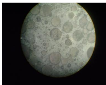
Figure 4.4: Micrograph of FMB 8:1:5 fired at 900°C
