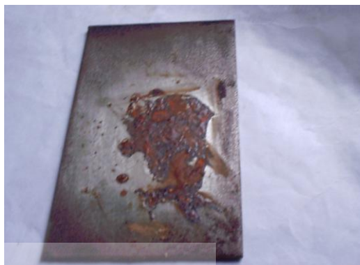
Figure 4.24: An uncoated surface two weeks after being treated with 10% salt solution
