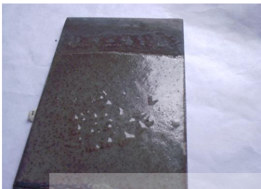
Figure 4.23: FAB 10:1:5 coated surface two weeks after being treated with 10% salt solution
