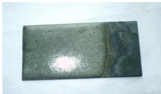
Figure 4.14: A picture of a test piece prepared with FAB 10:1:5 fired at 850°C
