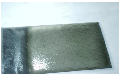
Figure 4.13: A picture of test piece prepared with FMB 12:1:5 fired at 850°C
