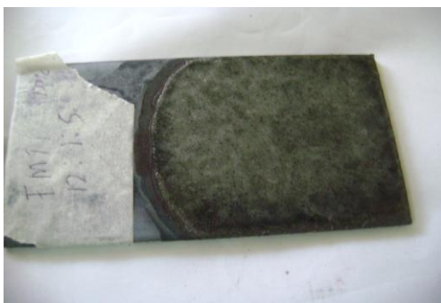
Figure 4.17: A picture of test piece prepared with FMB 12:1:5 fired at 900°C
