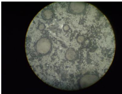
Figure 4.7: Micrograph of FAB 10:1:5 fired at 850°C
