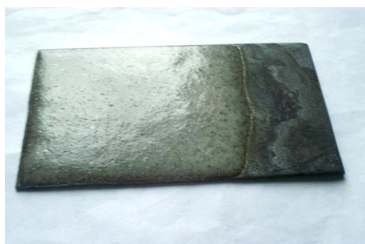
Figure 4.18: A picture of test piece prepared with the FAB 10:1:5 fired at 900°C
