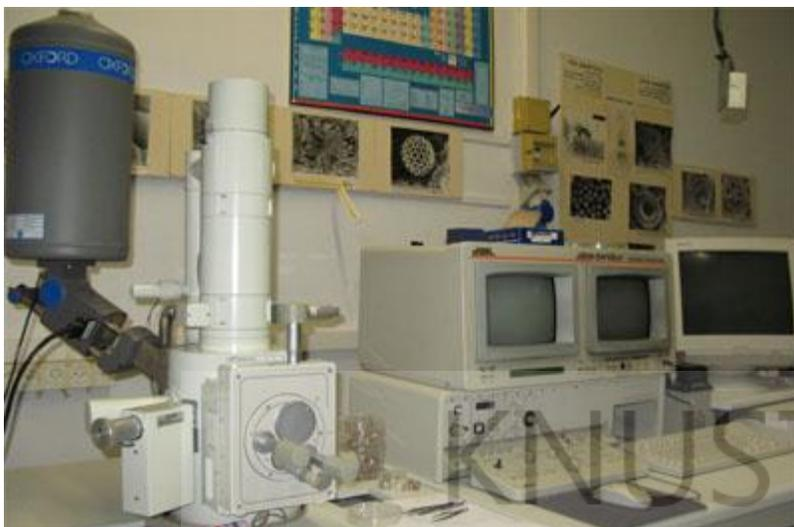
**Plate 4 Energy Dispersive X Ray Apparatus**
