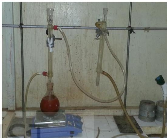
Plate 6 Bauxite waste in a refluxing set up before digestion
