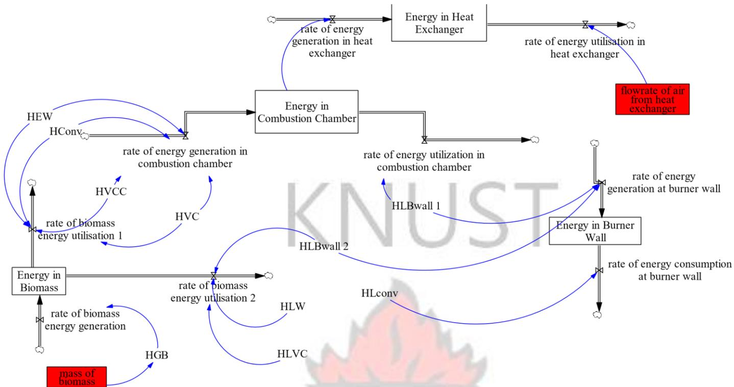
Figure 3.0.7: Stock-and-flow diagram of the burner system
