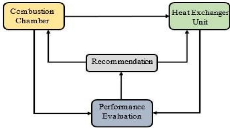
Figure 3.0.4: Inter-relations between various subsystems of the biomass burner
