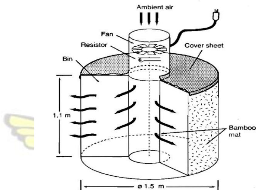
Figure 2.3: Components of the SRR-1 dryer (Source: Ban *et al.*, 1996)
