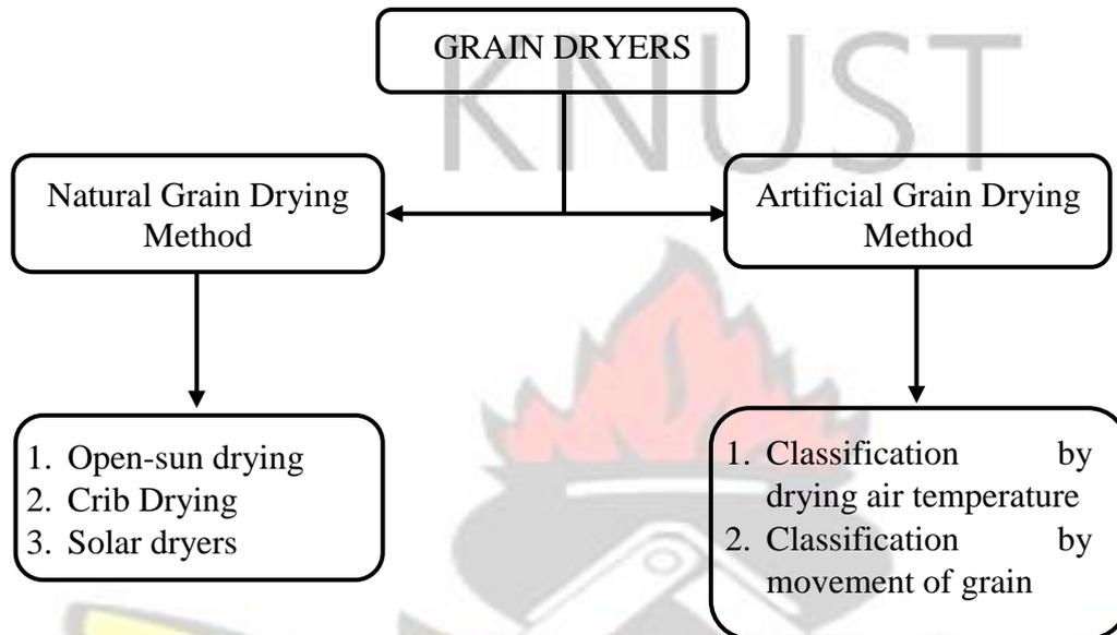
Figure 2.2: Classification of grain dryers (Meas *et al.*, 1998)
