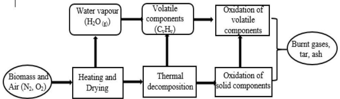
Figure 3.0.8: Biomass combustion process (Žecová and Terpák, 2010)
