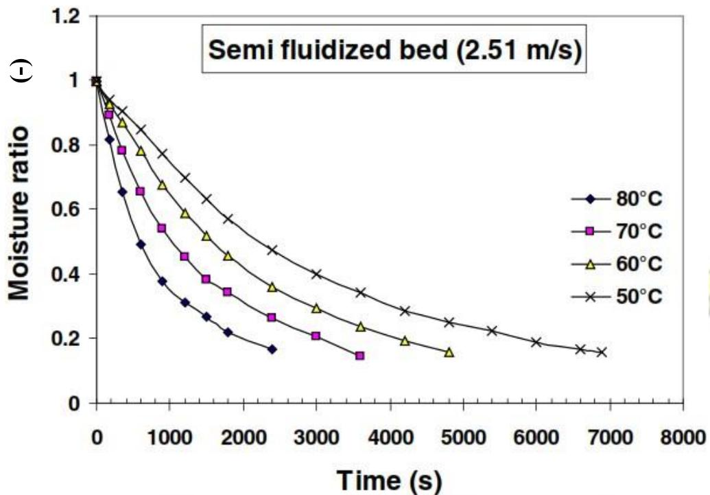
Figure 2.1: Effect of temperature on drying rate (Chayjan *et al.*, 2013)
