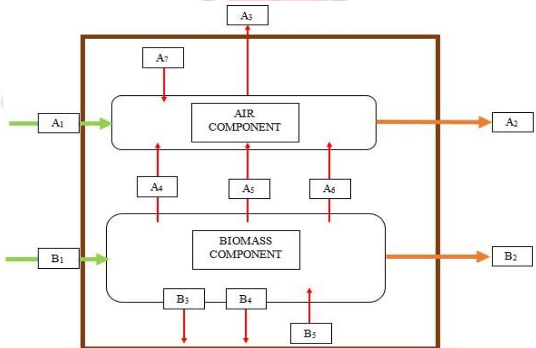
Figure 3.0.9: Energy dynamics during biomass combustion (modified from Žecová and Terpák, 2010)
