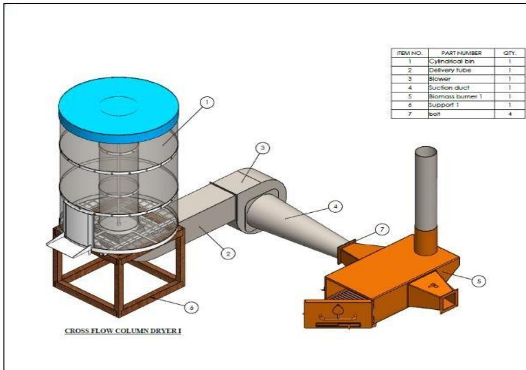
Figure 3.0.11: A CAD model of the crossflow column dryer showing all of its parts
