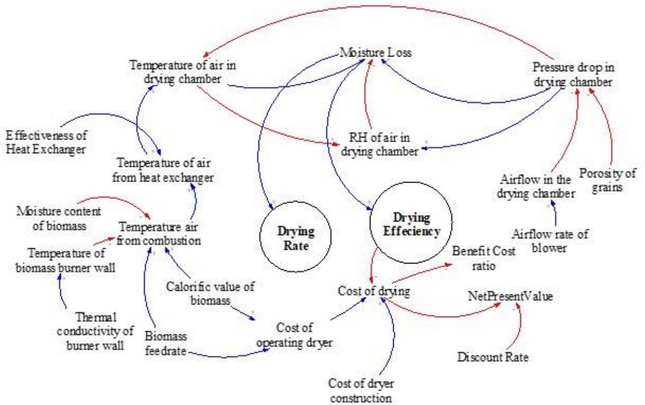
Figure 3.0.6: Causal loop diagram for the column drying system
