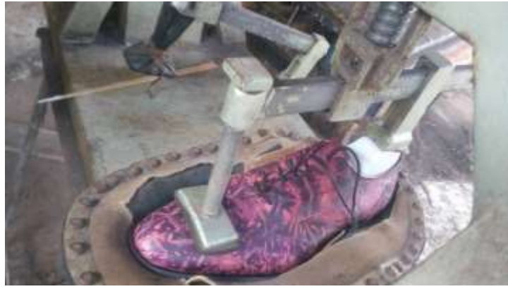
Plate 3.29: shoe placed under pressing machine
