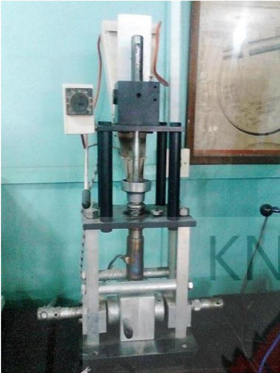
**Figure 3.5: A table top injection molder**
