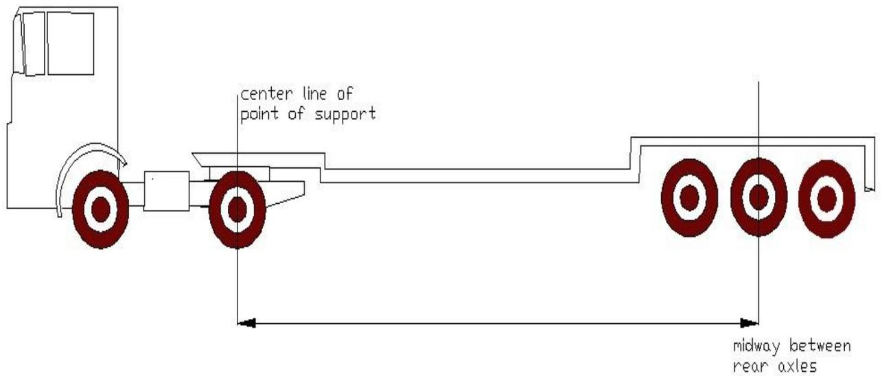
**Figure 2.6 (b)** Measurement of axle interspace on a triple-axle trailer (Source: Lowe, 2002)
