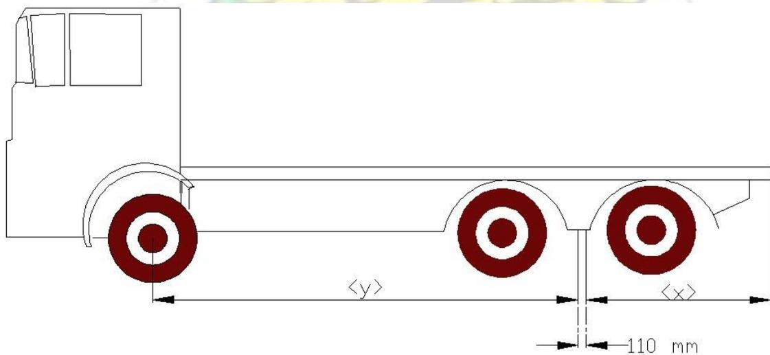
**Figure 2.4 (b)** Vehicles with three or more axles: Overhang „x“ measured from 110 mm behind the center line of the two rear axles must not exceed 60% of the
