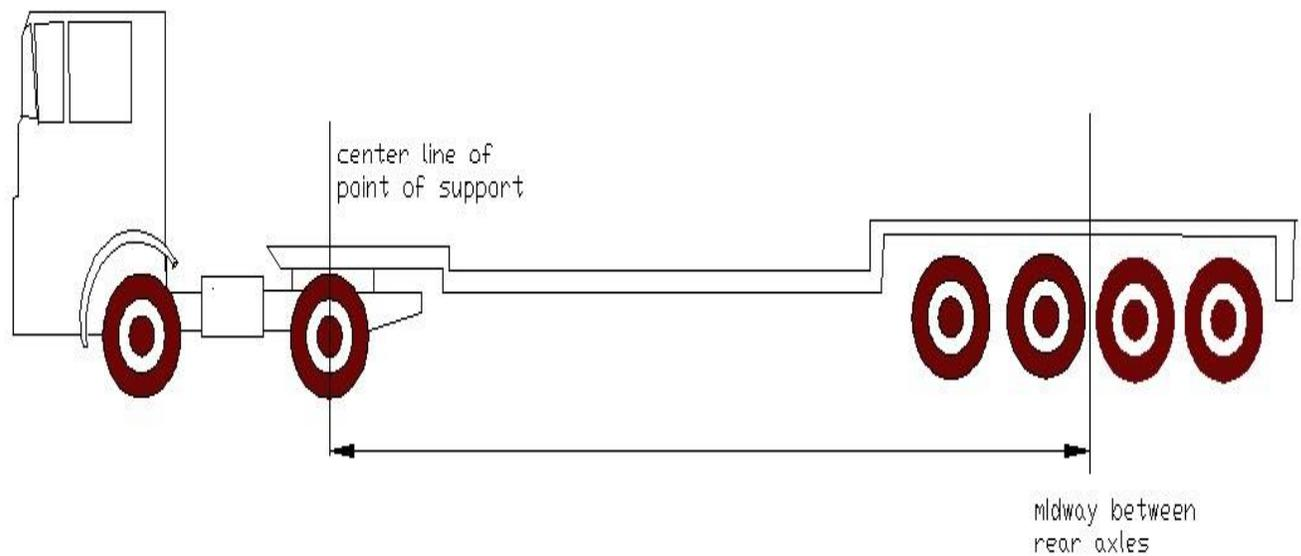
**Figure 2.6 (c)** Measurement of axle interspace on a quadruple-axle trailer
