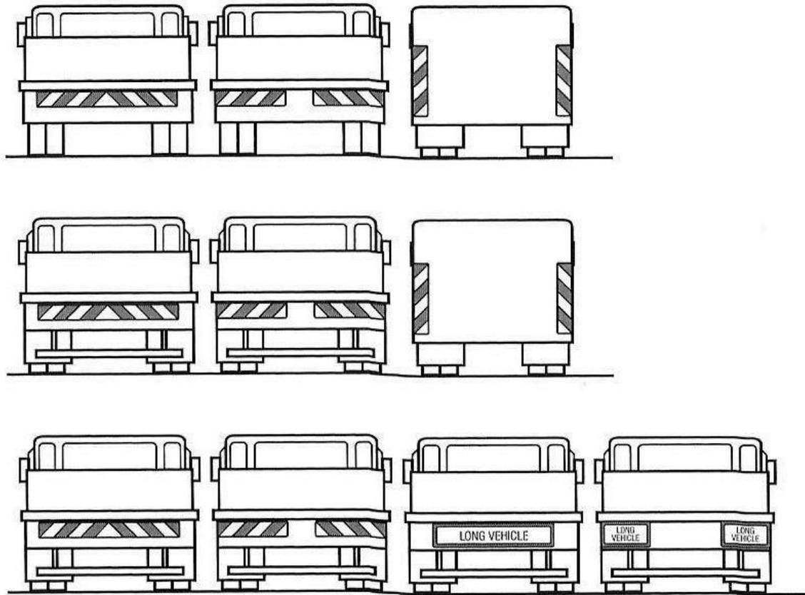
**Figure 2.7 (b)** How reflective markings are fitted to the vehicles (Source: Lowe, 2002)
