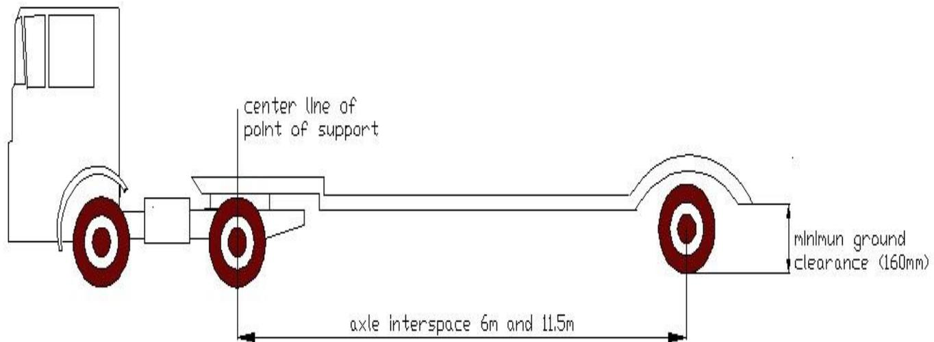
**Figure 2.5 (a)** Ground clearance for trailers with axle interspace between 6 meters and 11.5 meters
