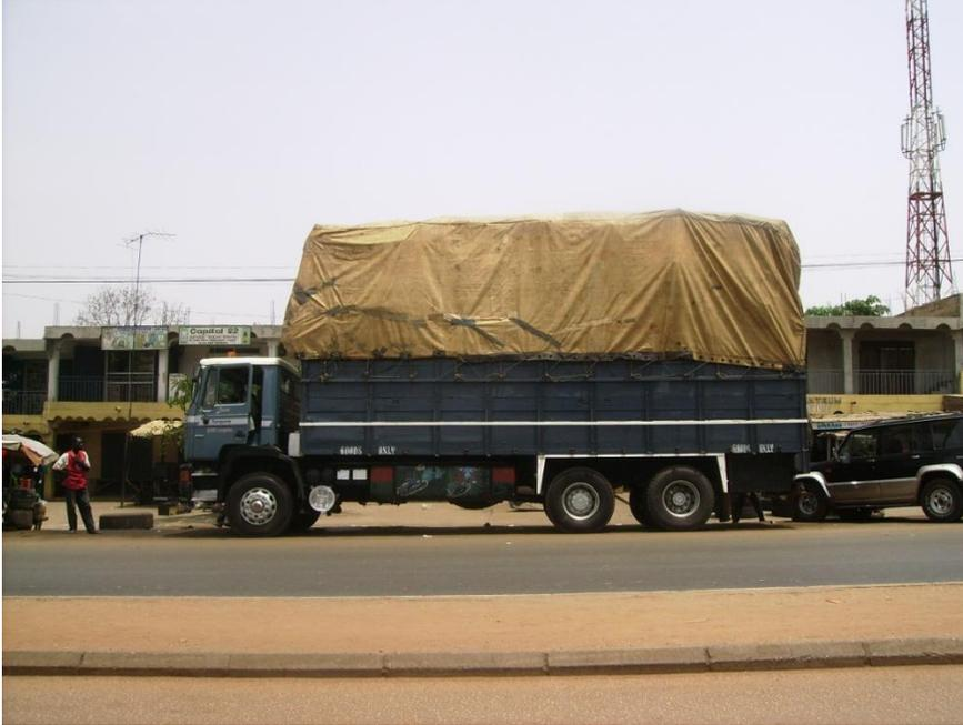
**Figure 4.1** An overloaded cargo truck exceeding permitted load height
