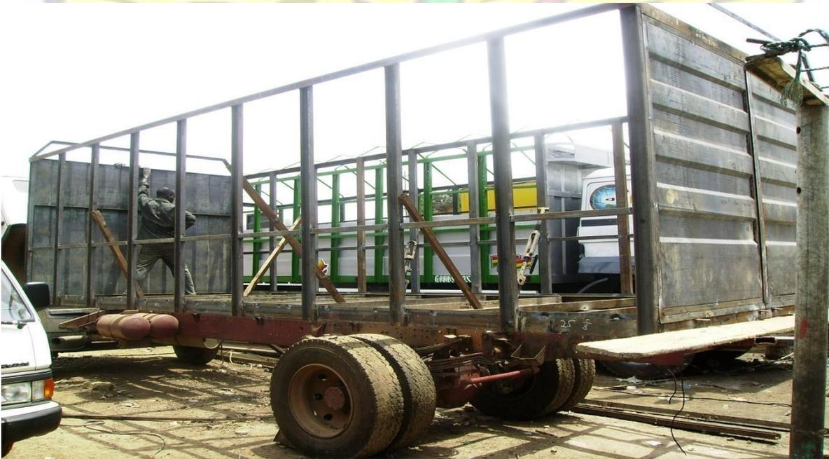
**Figure 3.1 (b)** Modification in progress (Increasing cargo truck capacity)
