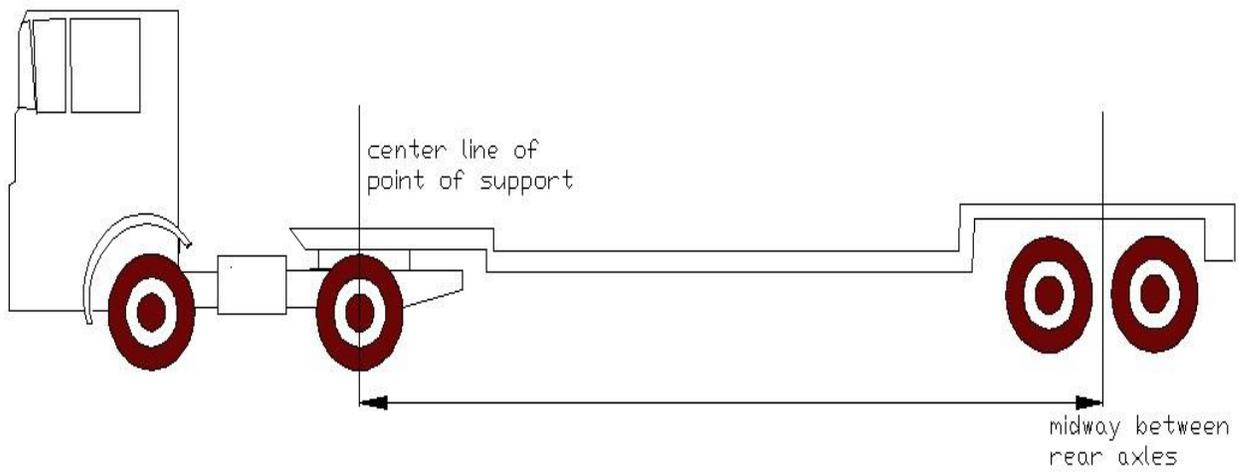
**Figure 2.6 (a)** Measurement of axle interspace on a double-axle trailer. (Source: Lowe, 2002)
