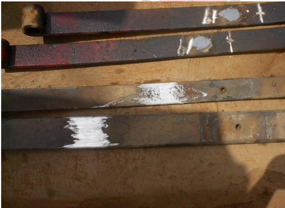
**Figure 3.2** Grinded springs after welding
