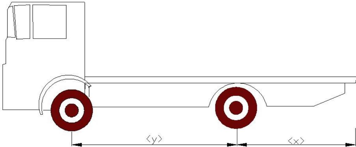
**Figure 2.4 (a)** Two-axled vehicles: Overhang „x“ must not exceed 60% of length „y“ (Source: Lowe, 2002)
