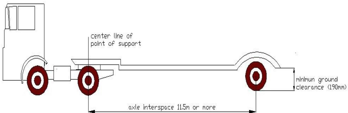
**Figure 2.5 (b)** Ground clearance for trailers with axle interspace of 11.5 meters or more (Source: Lowe, 2002)
