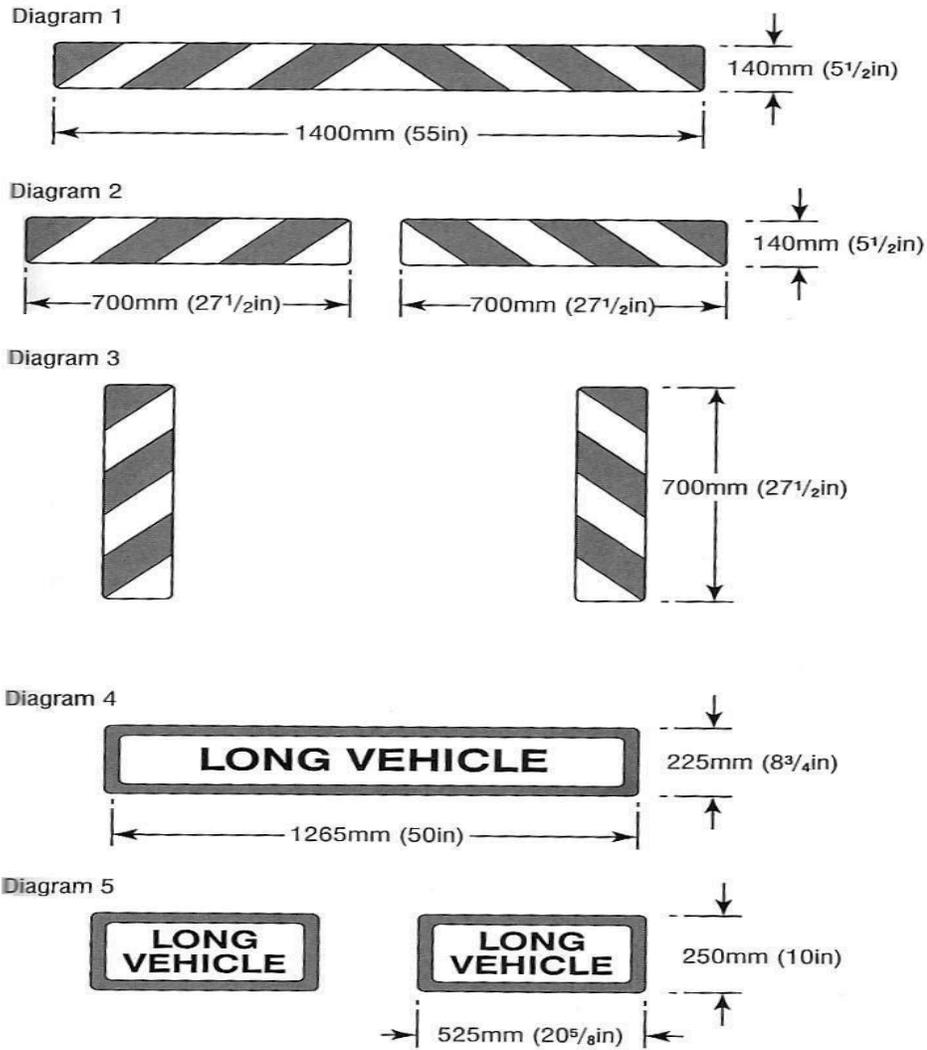
**Figure 2.7 (a)** The various types of reflective markings and their dimensions
