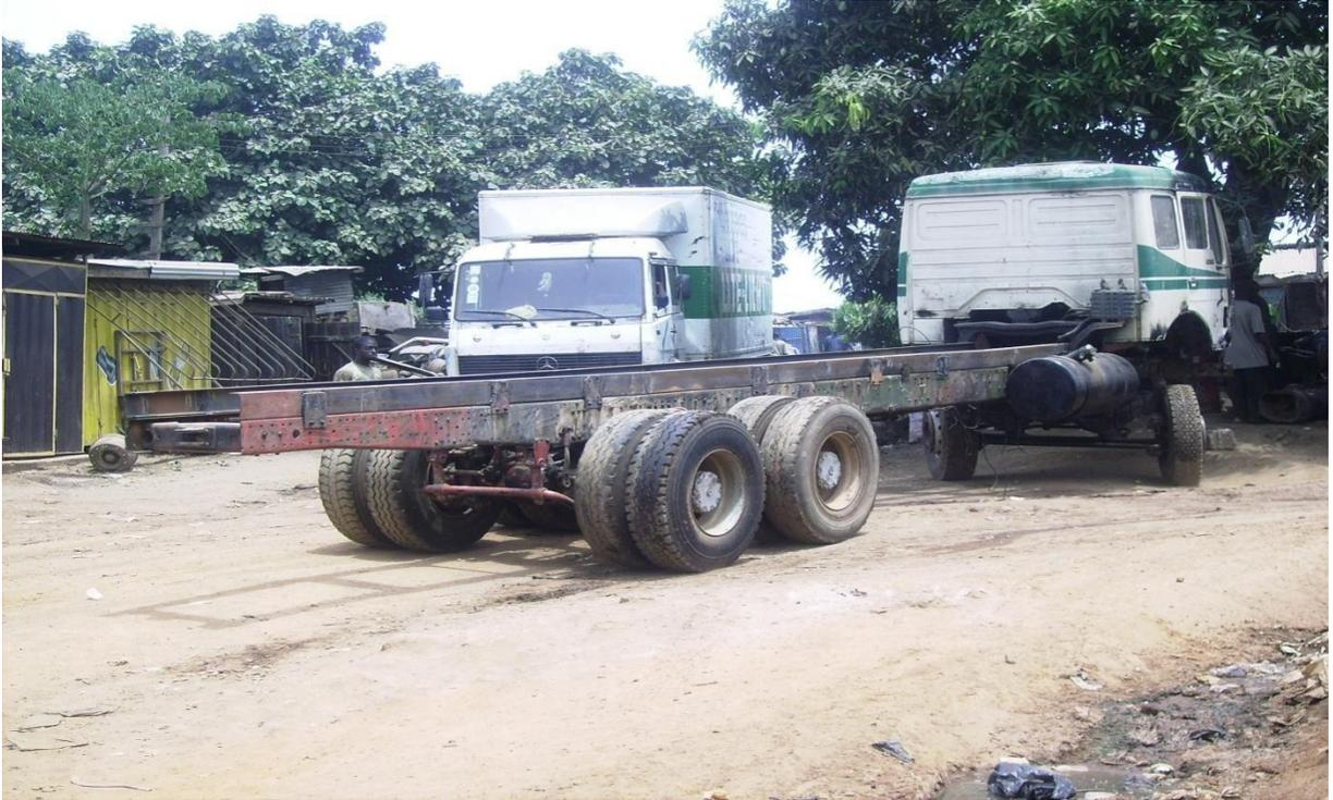
**Figure 3.1 (a)** A lengthened trailer frame
