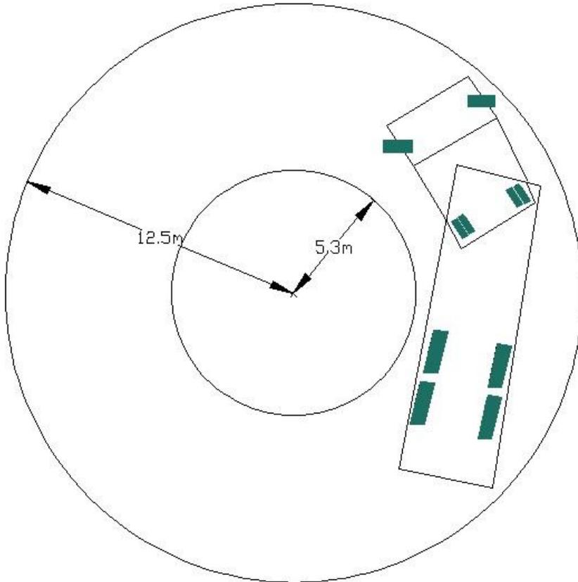
**Figure 2.1** The maximum and minimum outer and inner swept circles within which a 16.5 meter long articulated vehicle must be able to turn.
