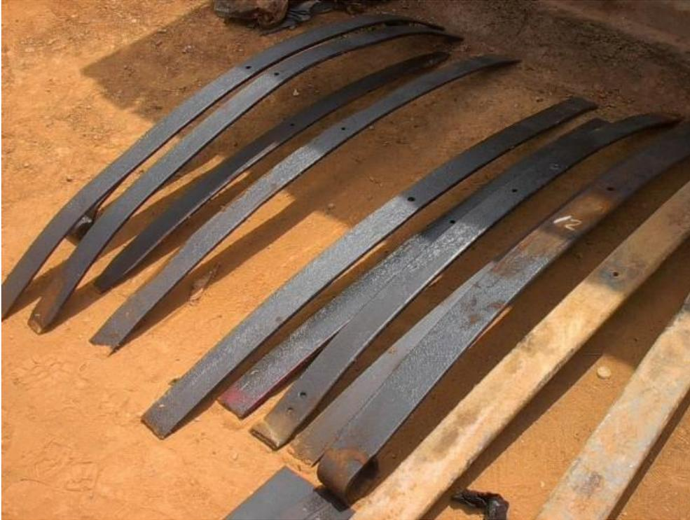
**Figure 3.3** Finished products (leaves painted black to conceal welded spot)
