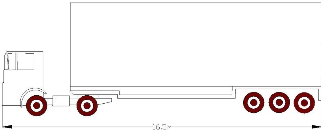
**Figure 2.2** The maximum permitted length for articulated vehicles and semi-trailers (Source: Lowe, 2002)
