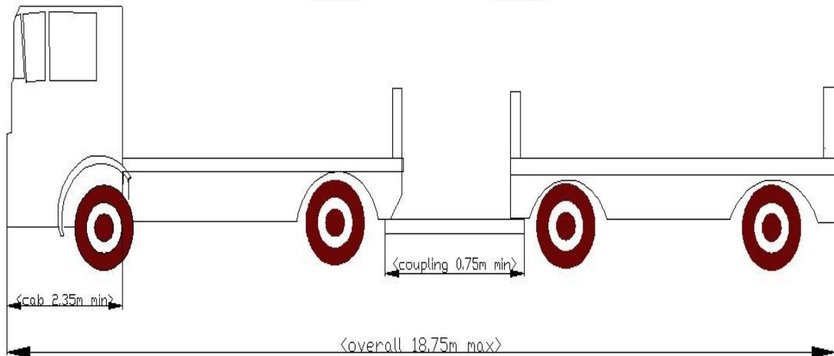
**Figure 2.3** The maximum length for drawbar vehicle combination.
