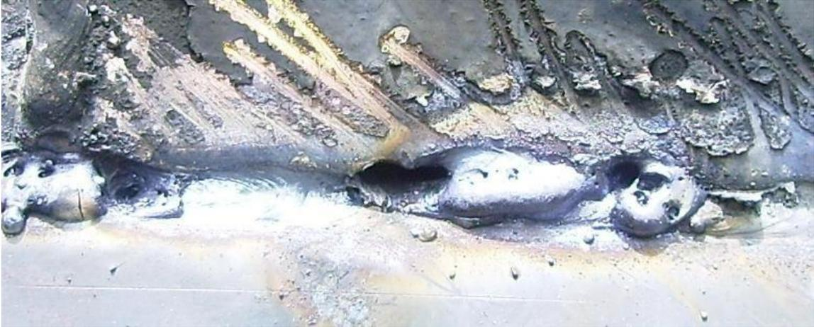
**Figure 3.7** Cavity and inclusion defects in a weld produced at Suame Magazine
