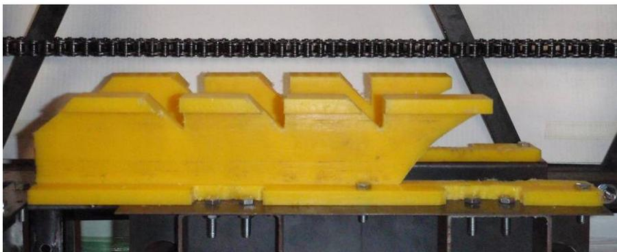
**Fig. 4** Plastic rail used to open the containers; the diagonal notches allowed the nymph predators remaining inside the container to be shaken out.
