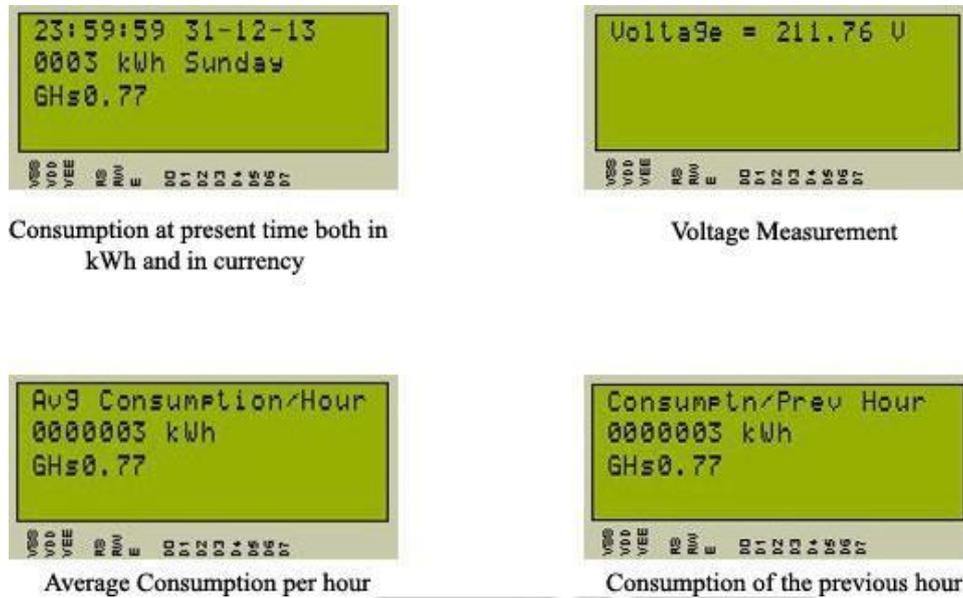
**Figure 5.4 LCD displaying consumption data and power measurements**
