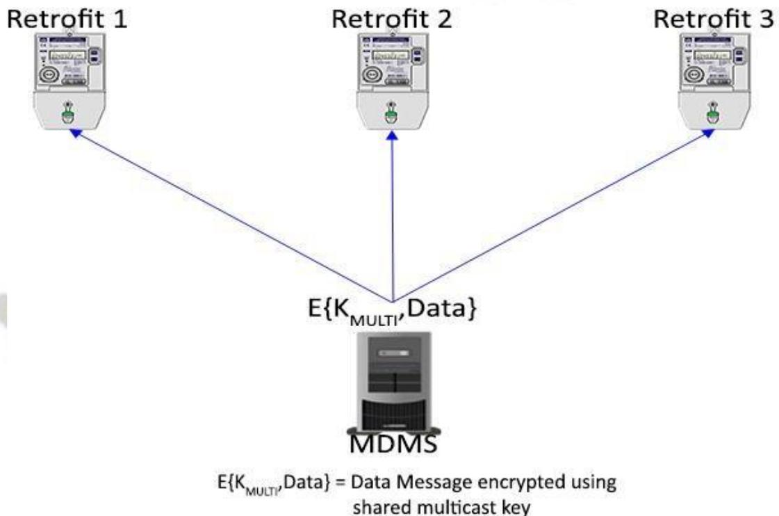
**Figure 6.19 Transmission of an encrypted multicast message**
