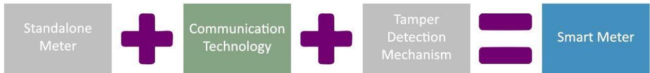
**Figure 4.1 Basic Constituents of a Smart Meter**
