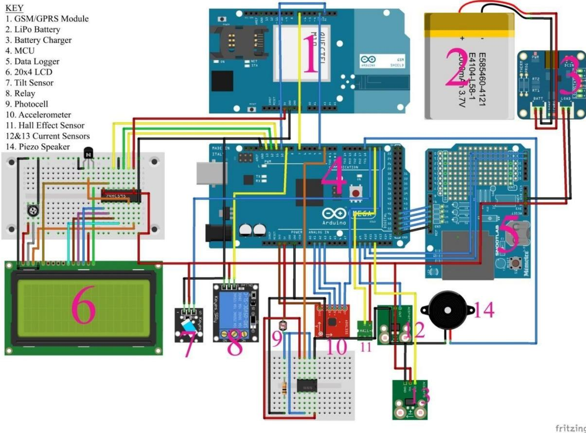
**Figure 5.6 Breadboard Schematic Diagram of Smart Retrofit Design**
