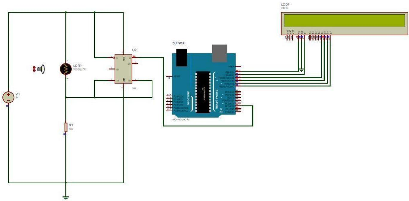
**Figure 4.12 Simulation Schematic of LED Pulse Detection**
