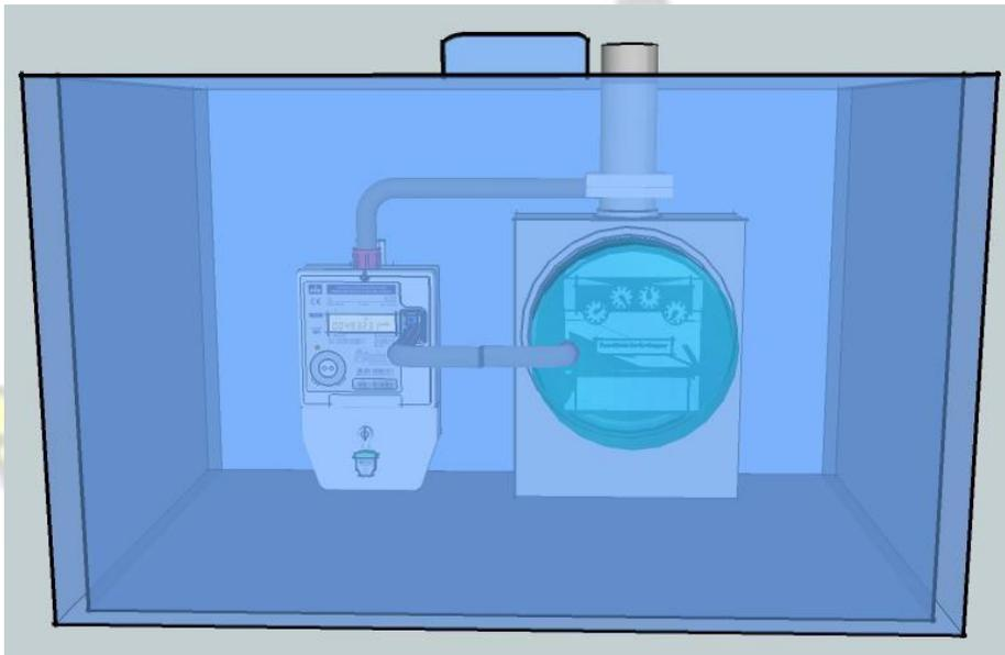
**Figure 5.11 Front view of Retrofit and Meter's 3D Model in Transparent Casing**
