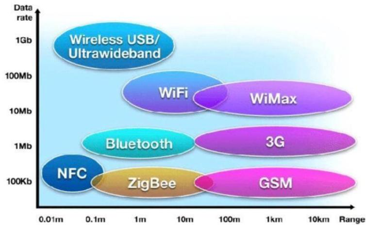
**Figure 2.9 Comparisons of Wireless Communication Technologies [2.56]**
