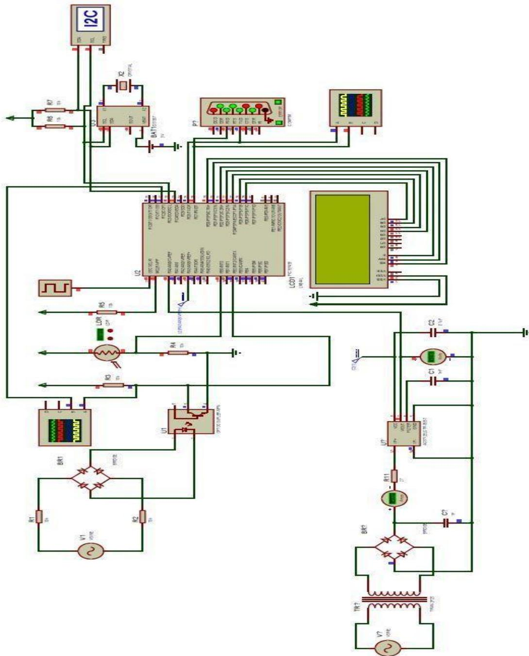
**Figure 5.3 Schematic of Smart Retrofit Circuit Simulation**
