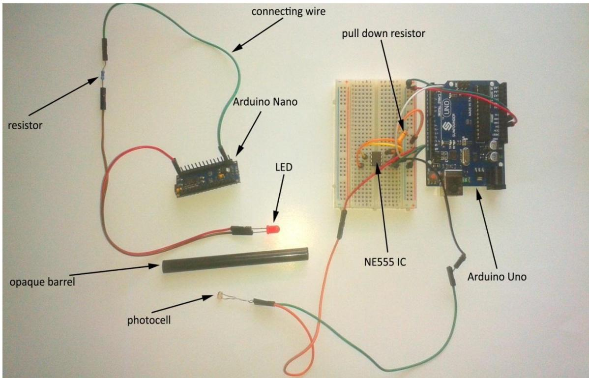
**Figure 4.14 Experimental Setup for Photocell Response Test**
