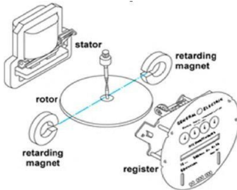
**Figure 2.12 Basic parts of an electromechanical meter [2.68]**
