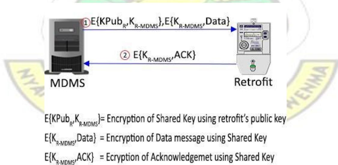
**Figure 6.18 Transmission of unicast data messages from MDMS to Retrofit**
