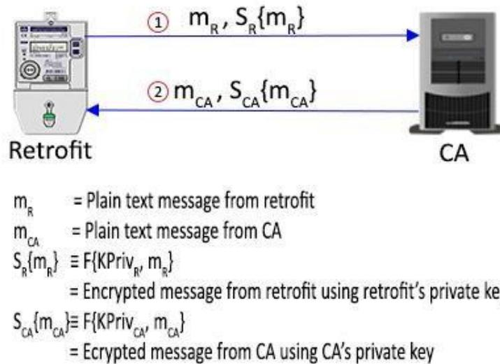
**Figure 6.15 Authentication Process between Smart Retrofit and CA**
