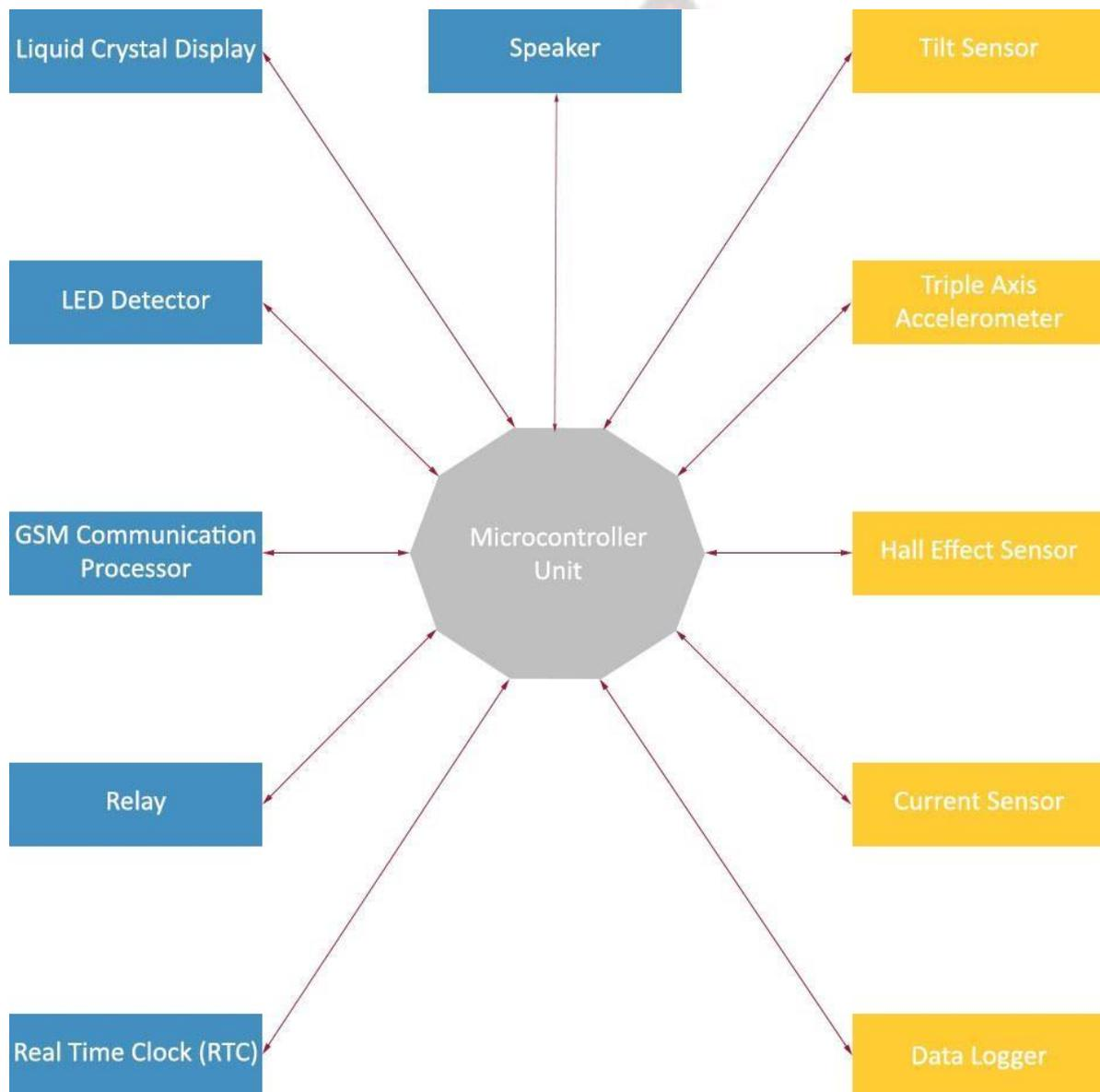
**Figure 4.15 A Basic Block Diagram of Interconnecting Components**
