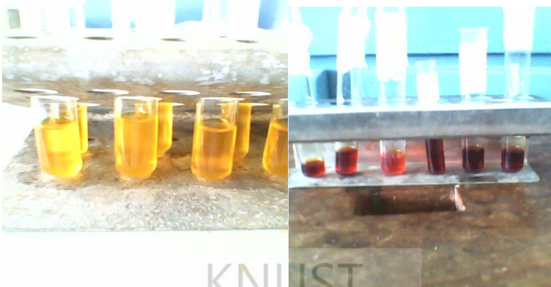
Plate 5; Enzymes, starch, buffer after DNSA is added. Plate 7; culture after incubation
