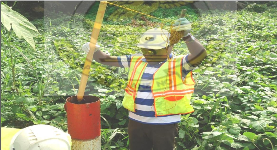
**Plate 2: Sampling from monitoring boreholes**
