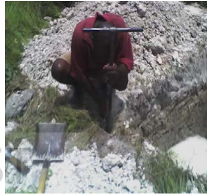
Figure 3.6 Sampler driven deep into the earth
