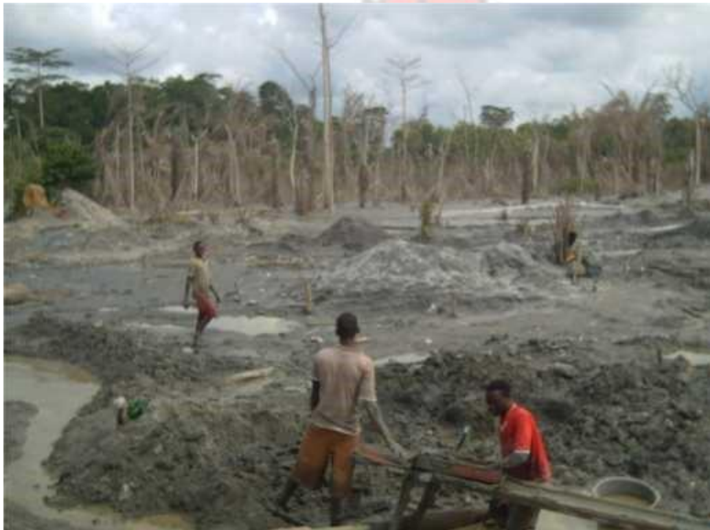
Plate 2.1: Shallow Alluvial Mining Technique
