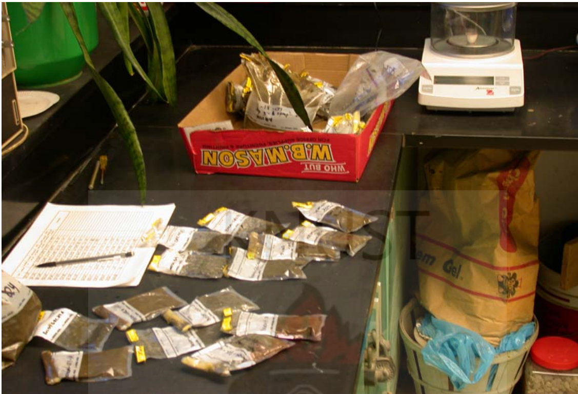
Figure 3.23 Picture of the sample preparation process showing samples in labeled bags, data sheet and a measuring balance.
