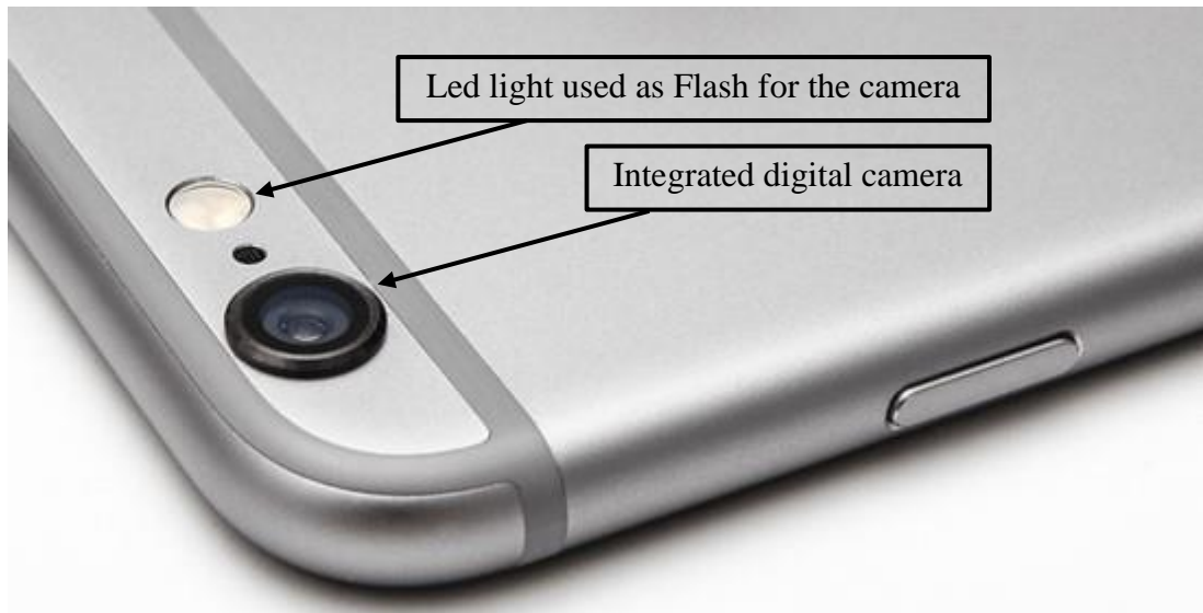
Plate 2.2: The integrated digital camera and Flash on an iPhone
