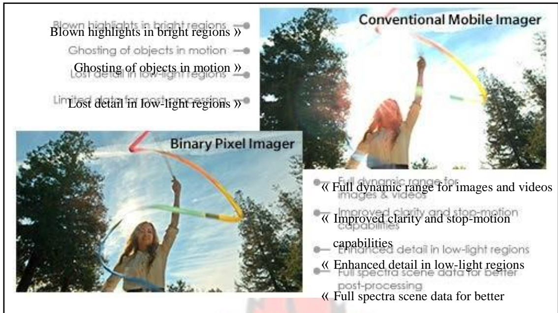
Plate 2.4: shows Binary Pixel Imager verses Conventional Mobile Imager (Rambus, 2015).
