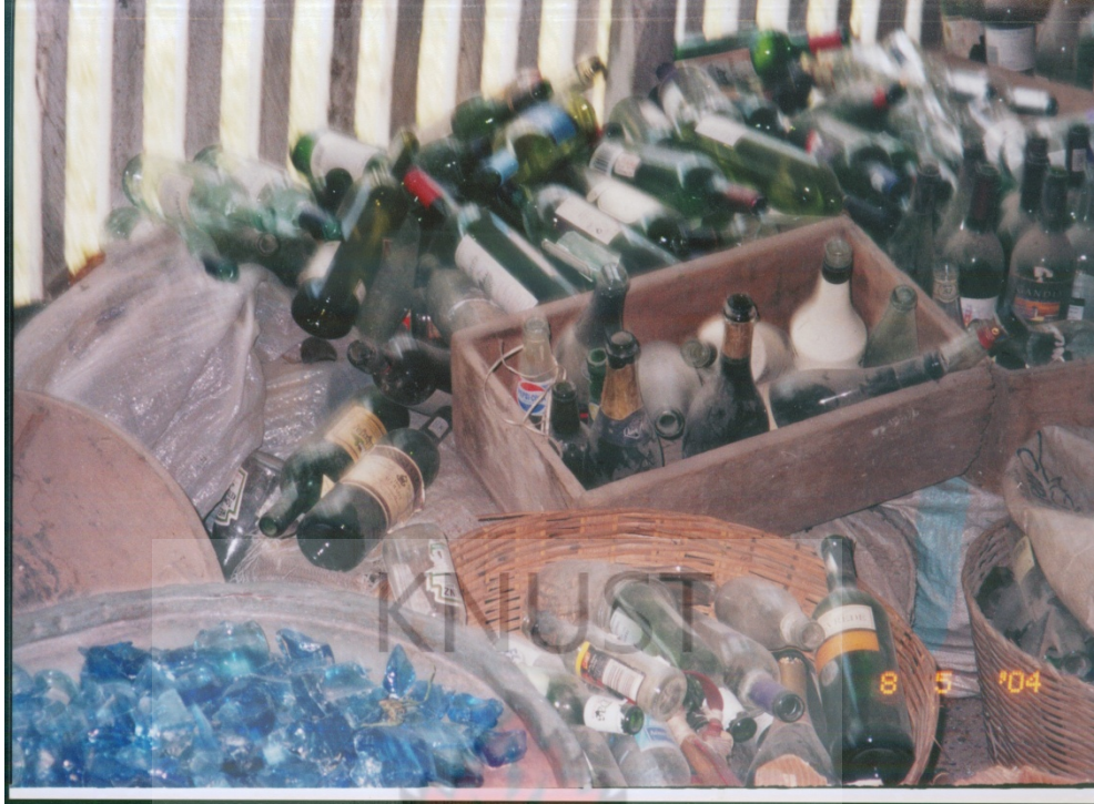
Plate 4.3 Glass bottles as raw materials for making beads. (Source: Cedi Beads, Odumase Krobo, picture by researcher)
