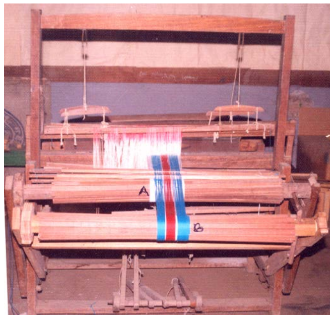
Plate 9 – Back Of Adapted Loom Showing Pile Warp and Ground Warp.
