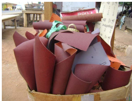
Plate 4.27 Sand paper Sand paper: Is used for sanding the finished carvings to make the surface smooth. The reason is that smooth carvings when polished will reflect the light of intelligence that went into the carvings.
