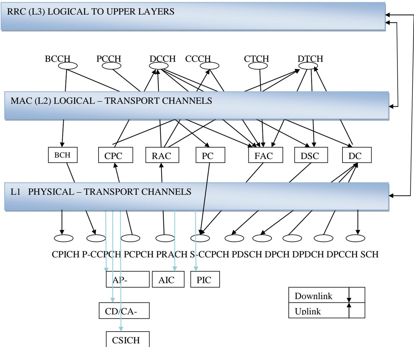
Figure 3-3 3G Logical ->Transport -> Physical Channel Mapping [32]
