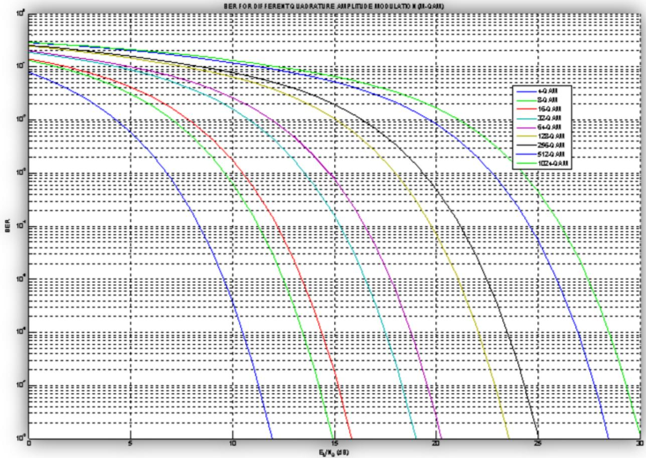
Figure 5-6 Comparison of various M-QAM modulation techniques
