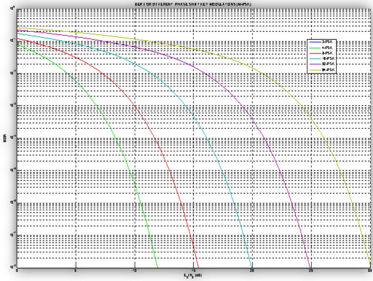
Figure 5-7 Comparison of M- PSK modulation techniques
