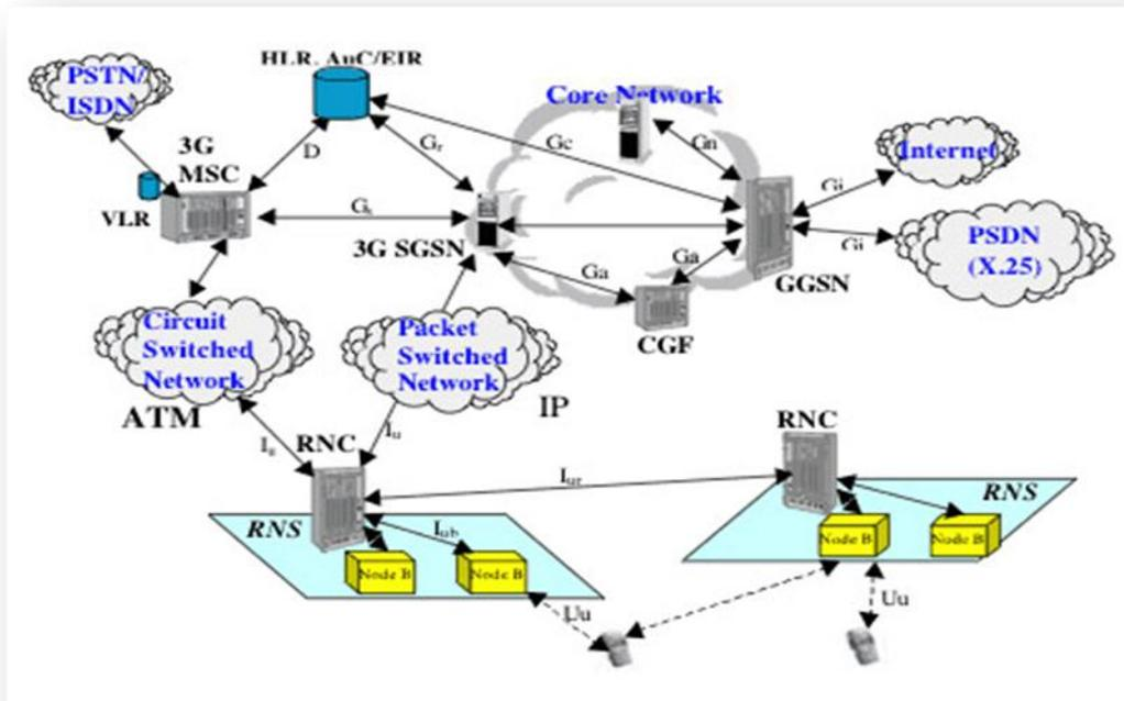
Figure 3-1 UMTS 3G Network Architecture
