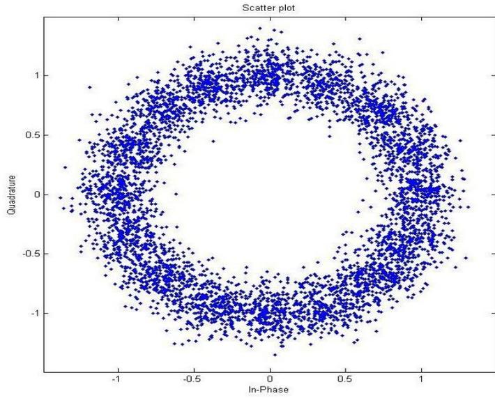
**Figure 5-8** Signal Constellation Diagram showing 16-PSK using MATLAB
