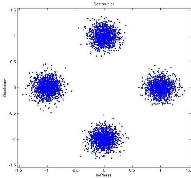
Figure 5-6 Signal Constellation Diagram showing 4-PSK using MATLAB
