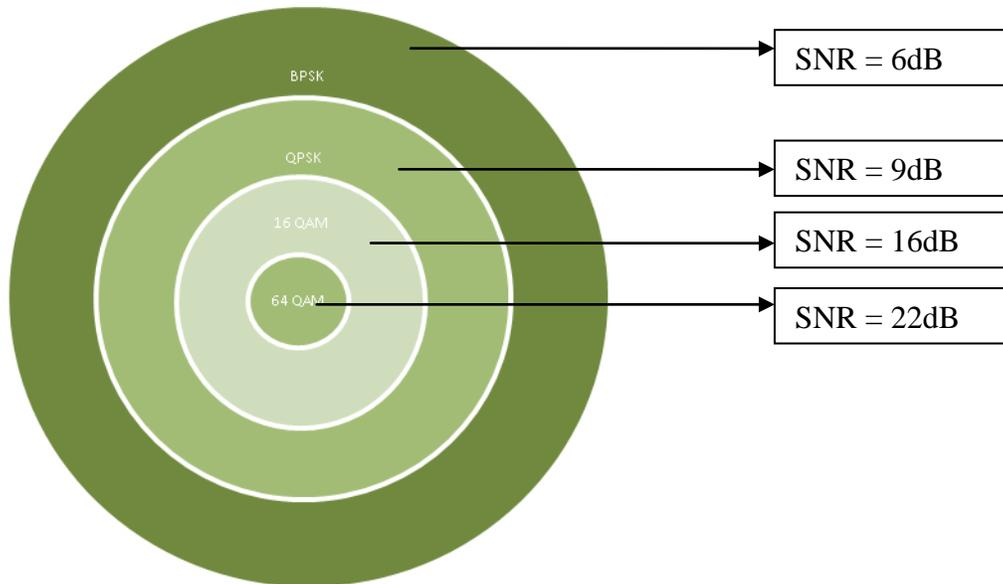
Figure 5-5 Comparison the range of various modulation techniques [33]
