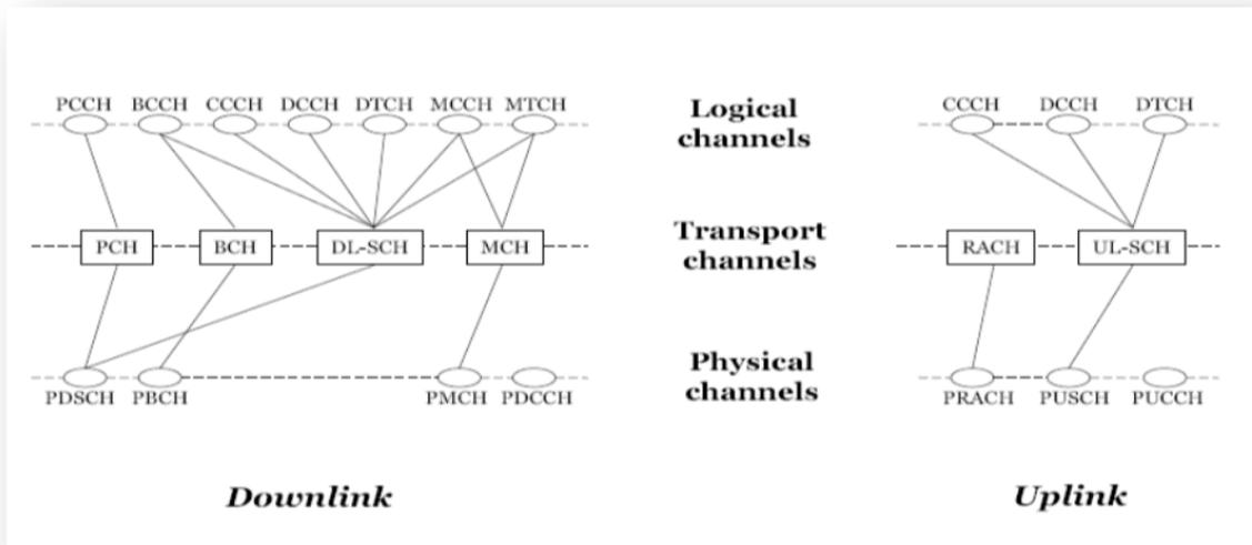
**Figure 3-5 LTE Logical Transport and Physical Channel Mapping [4][23][42]**
