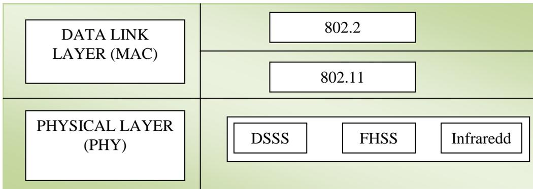
**Figure 2-4 Wi-Fi physical and data link layer architecture [12]**
