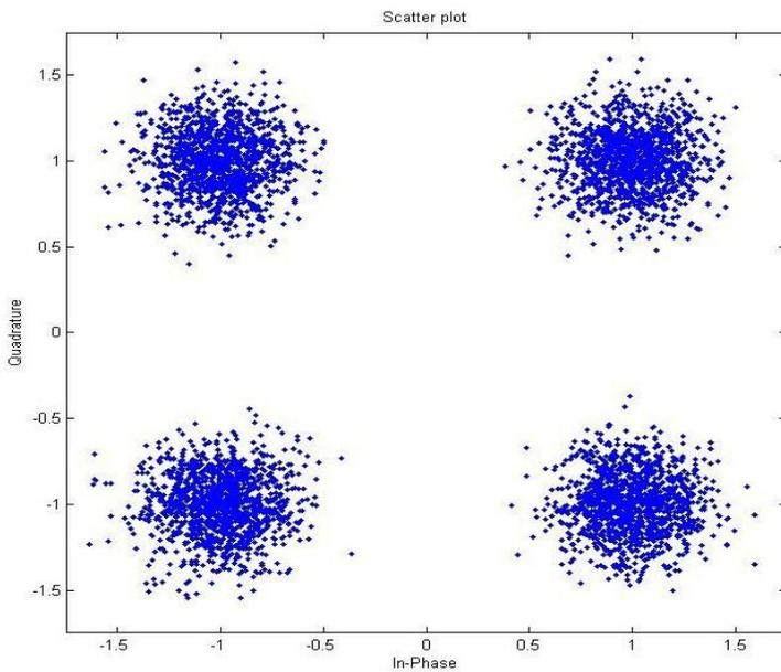
Figure 5-7 Signal Constellation Diagram showing 4-QAM using MATLAB
