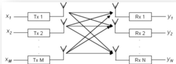
Figure 2-2 Multiple Input Multiple Outputs - MIMO
