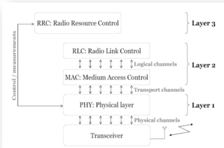
Figure 3-2 Physical layer in the UTRA protocol stack [4]
