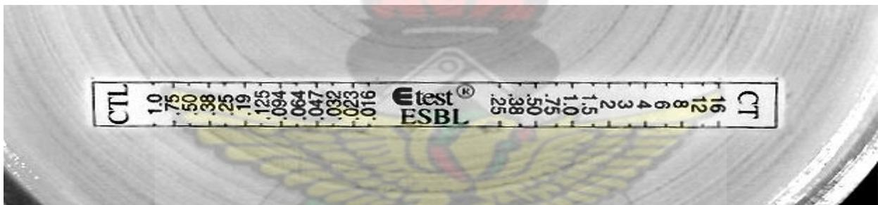
Figure 8d. The E-test strip method: When MIC values are above the test ranges, result is Non-Determinable (ND) (AB BIODISK, Dalvägen 10; 169 56 Solna, Sweden).
