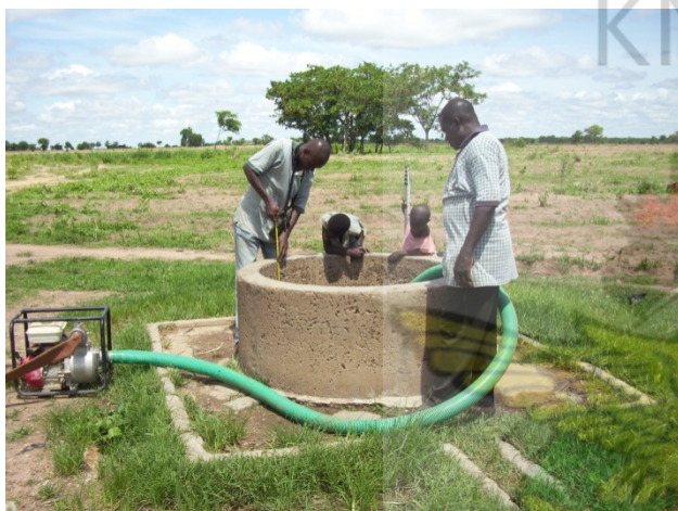
Fig.XXV: Measuring yield of a HDW
