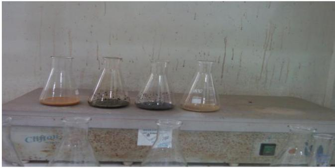
**Plate 3- 4:** Boiling of media in nitric acid for the extraction of Al from AOCM
