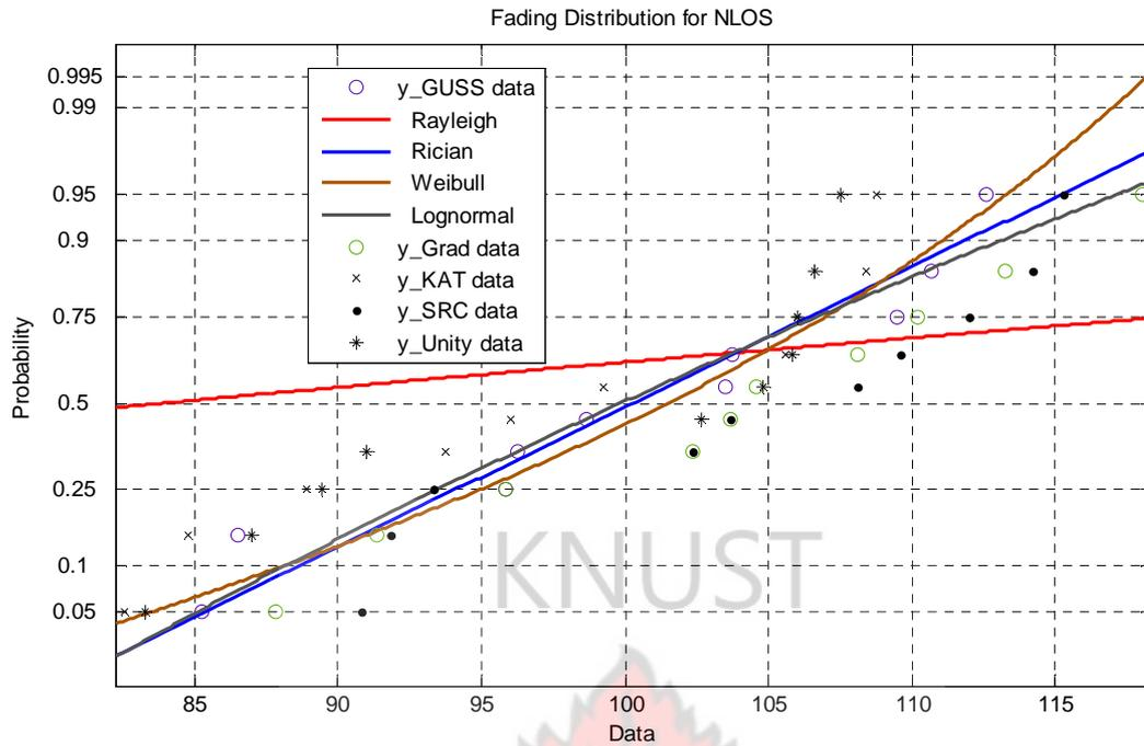
**Figure 4-2:** A comparison of fits to Log-normal, Rician, Weibull and Rayleigh Probability in NLOS environment
