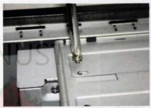
Fig 2.8: Installing optical drive.
