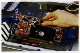
Fig 2.5: Installing the video card.
