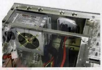
Fig 2.4: Installing the power supply
