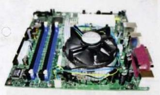
Fig 2.2: Installing the heat sink
