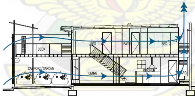
Figure 2.17 Typical section showing air flow. (Source: Townsville City Council Planning and Development Services 2007)
