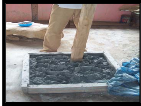
Plate 4.29 Clay being pounded for mould Making
