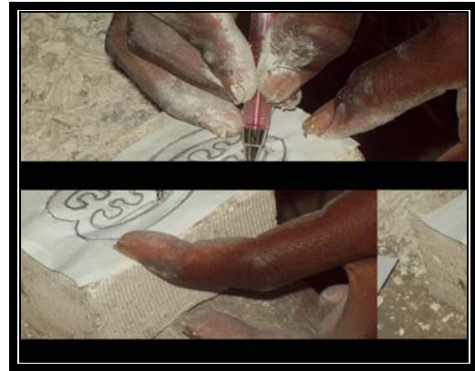
Plate 4.36 Tracing of design onto plaster
