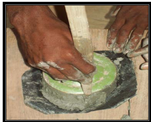
Plate 4.31 Defining the shape of the mould
