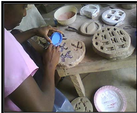
Plate 4.40 Filling of the moulds with a mixture of colouring oxides and glass
