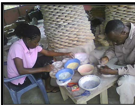
Plate 4. 39 Dry mixing of colouring oxides and powdered glass
