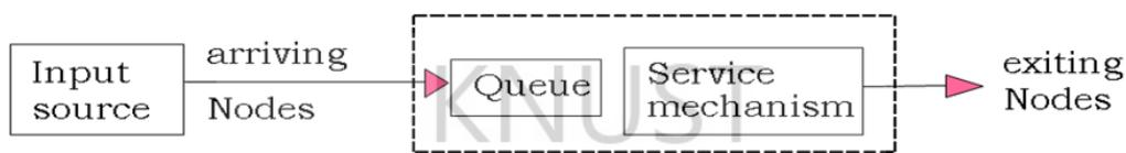
**Figure 3 1: M/M/1 Queueing System Model**
