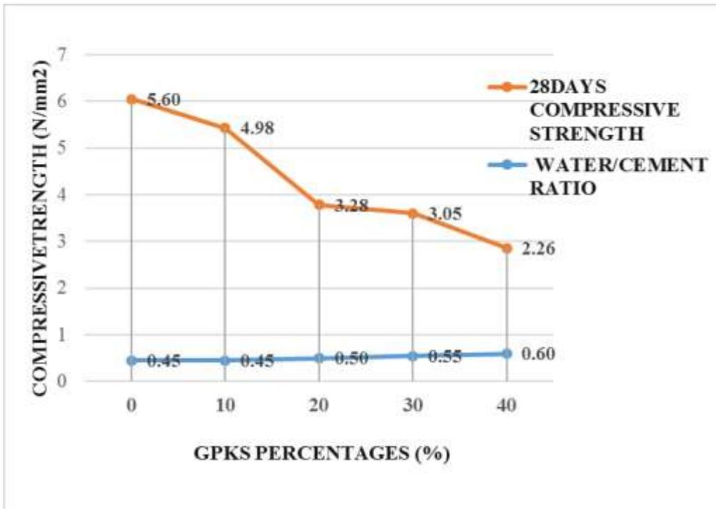
Figure 4.25a, Effect of Water on Strength (125mm solid block with GPKS aggregate Type A)
