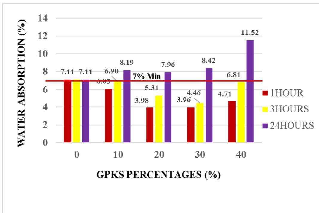
Figure 4.7b Water absorption of cubes produced with GPKS (Type B)
