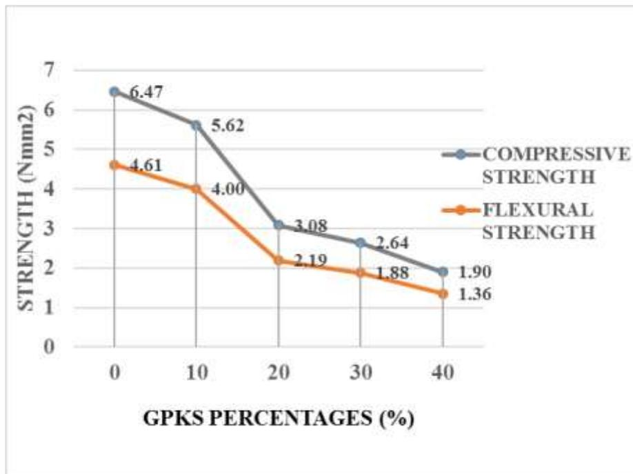
Figure 4.28a, Compressive versus Flexural Strengths (with GPKS aggregate Type A)
