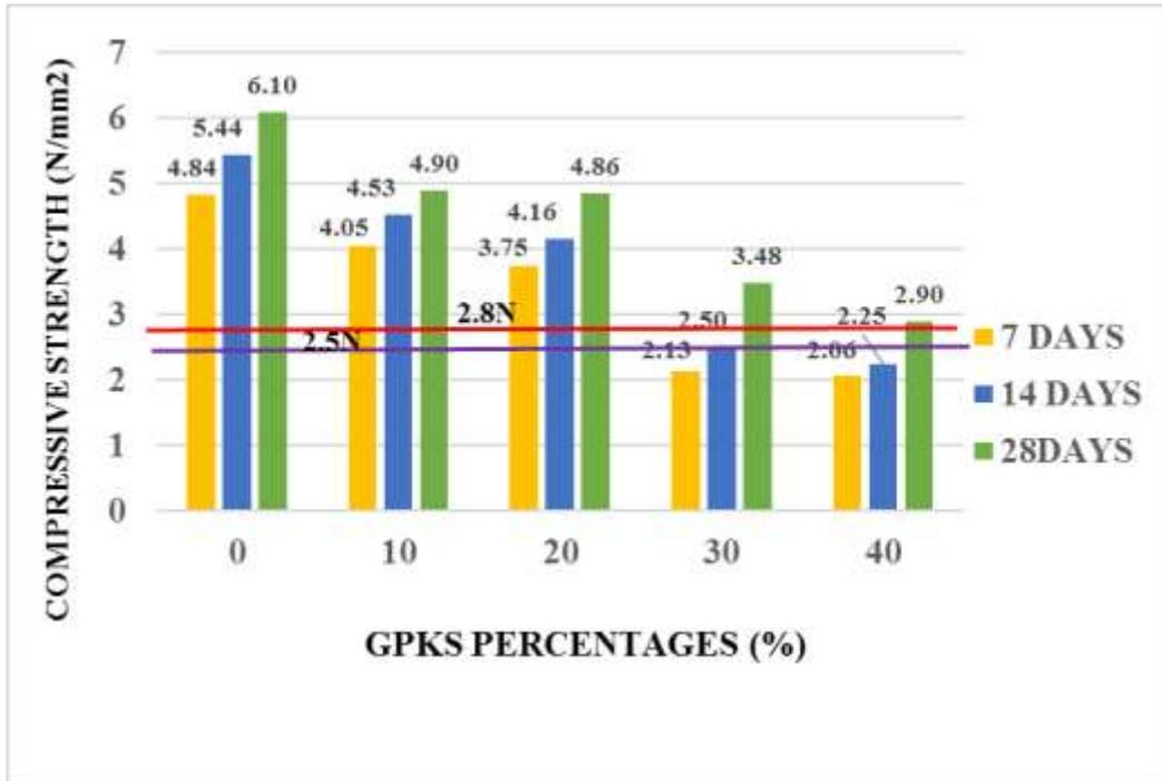
**Figure 4.11b, Compressive strength of 125mm cellular block with (GPKS Type B)**
