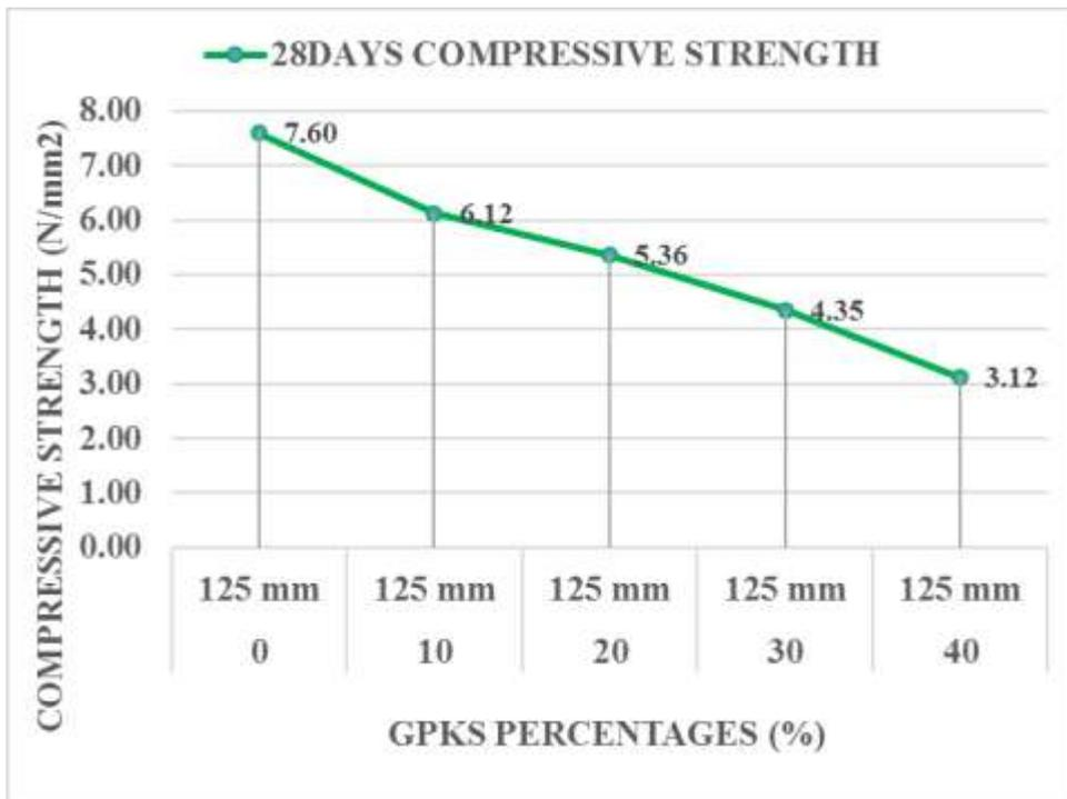
Figure 4.21b, Strength Verses Size of 125mm solid block with GPKS aggregate Type B
