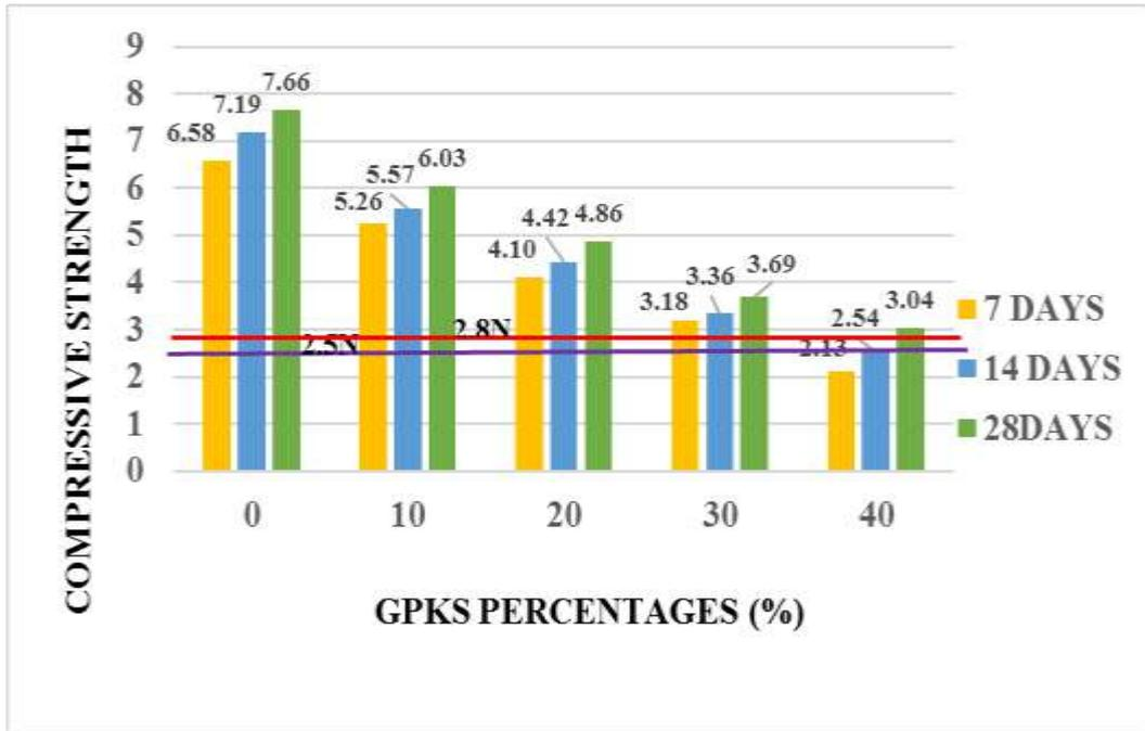
Figure 4.8b, Compressive strength of 150mm solid block with (GPKS Type B)
