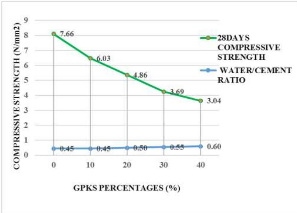
Figure 4.24b, Effect of Water on Strength (150mm solid block with GPKS aggregate Type B)
