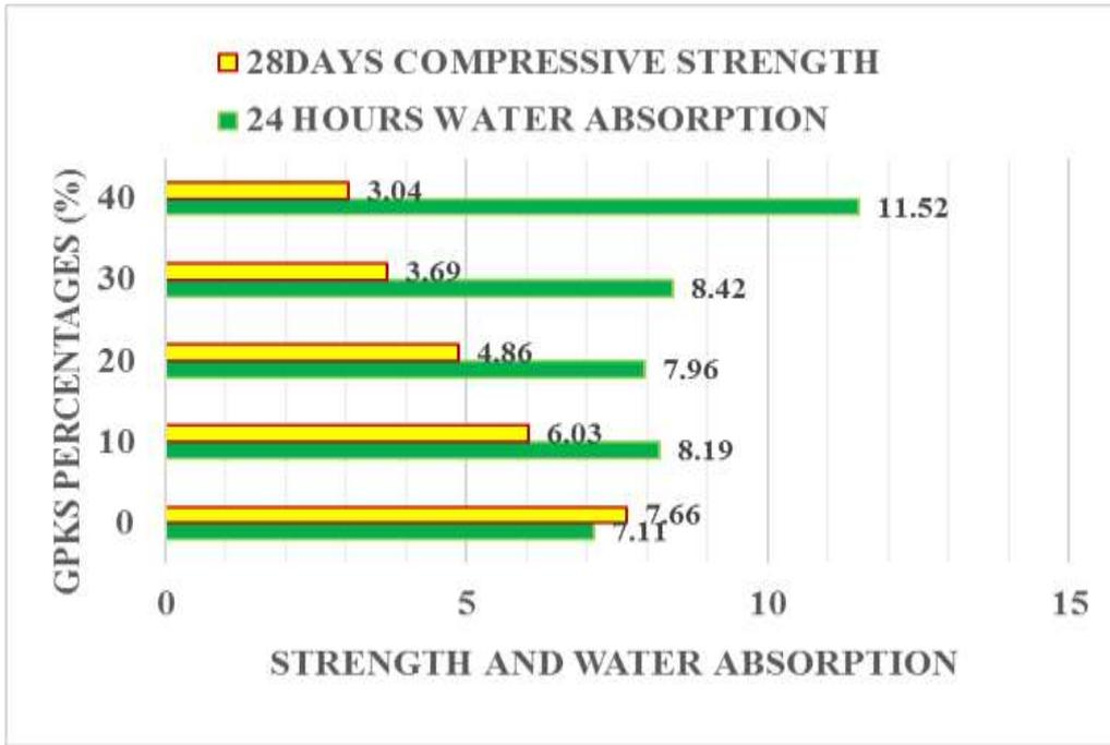
Figure 4.16b, Strength Verses Water absorption of 150mm solid block with GPKS aggregate Type B
