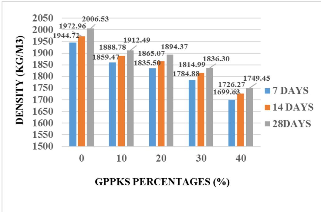
Figure 4.4a, Density of 125mm solid block with sand and GPKS aggregate Type A
