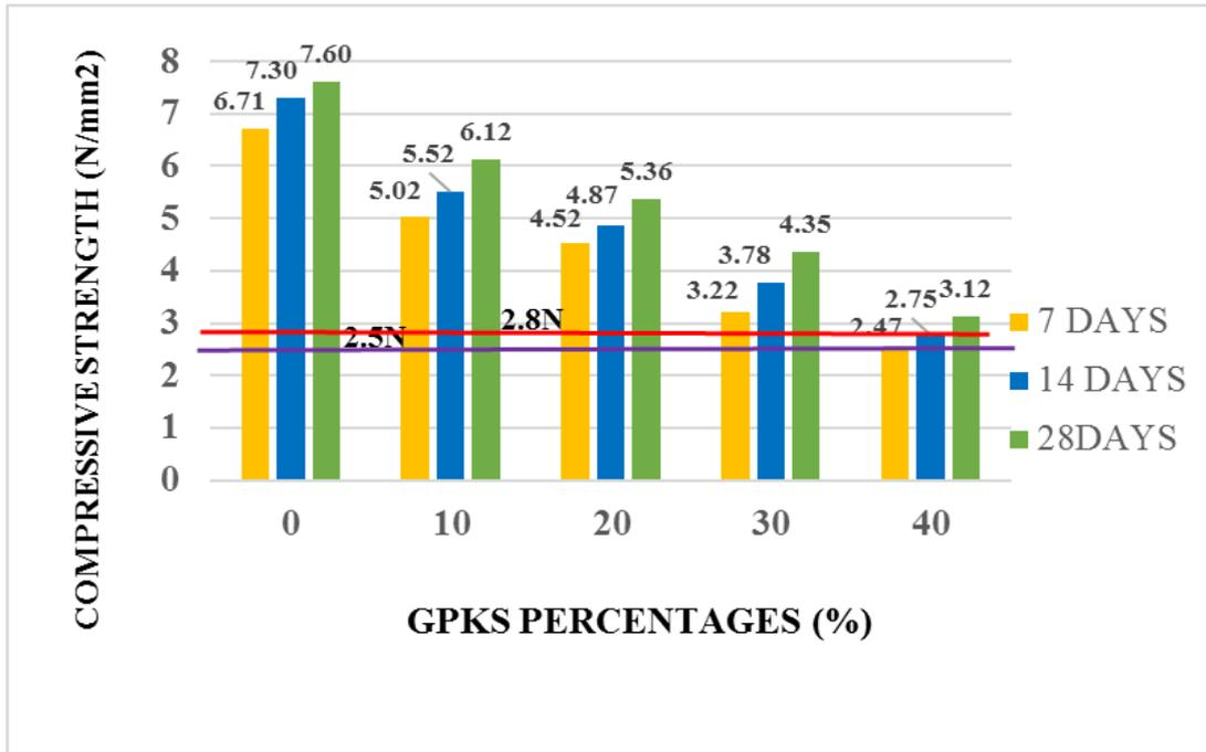
**Figure 4.9b, Compressive strength of 125mm solid block with (GPKS Type B)**
