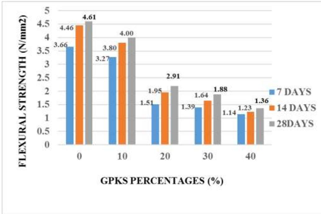
Figure 4.12a, Flexural strength of 150mm solid block with (GPKS Type A)
