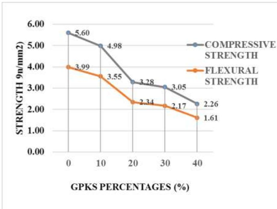
Figure 4.29a, Compressive versus Flexural Strengths (with GPKS aggregate Type A)
