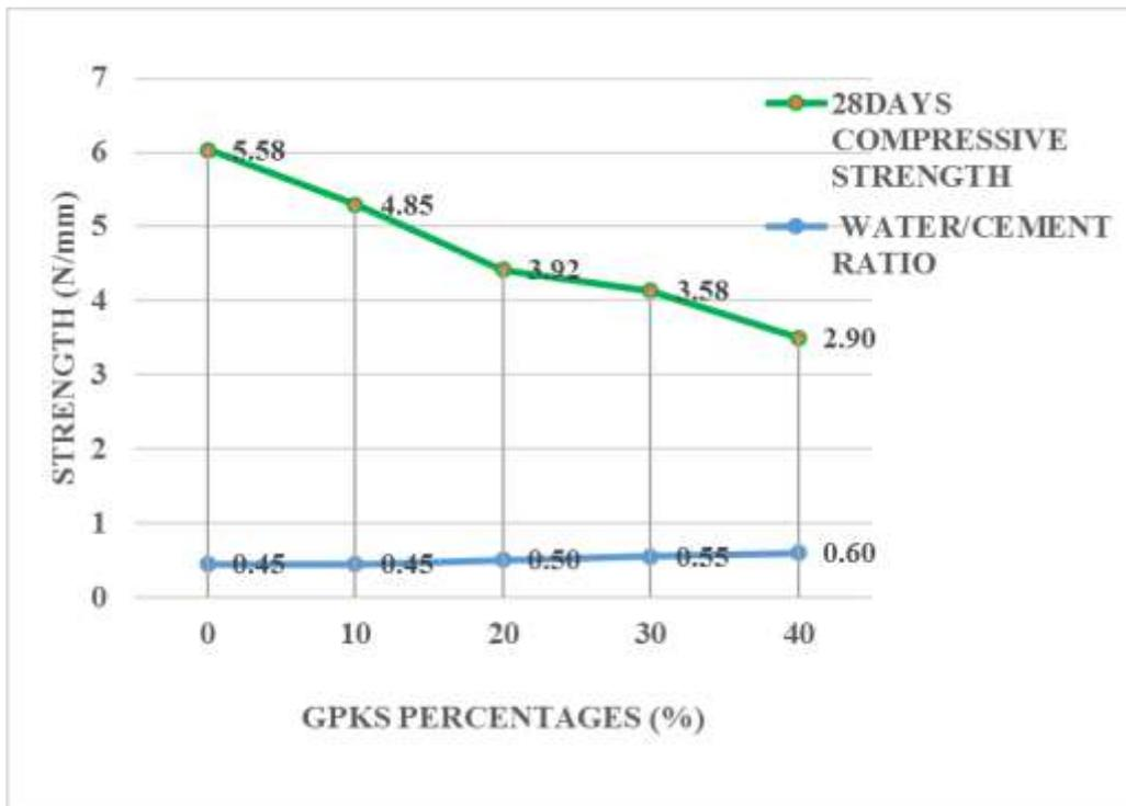
Figure 4.26b, Effect of Water on Strength (150mm cellular block with GPKS aggregate Type B)
