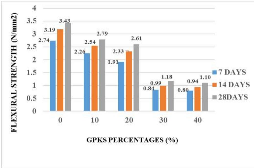
Figure 4.13a, Flexural strength of 125mm solid block with (GPKS Type A)
