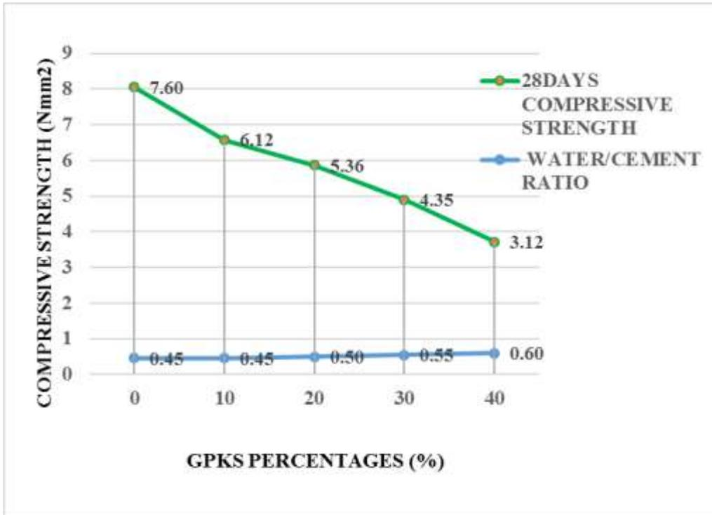
Figure 4.25b, Effect of Water on Strength (125mm solid block with GPKS aggregate Type B)
