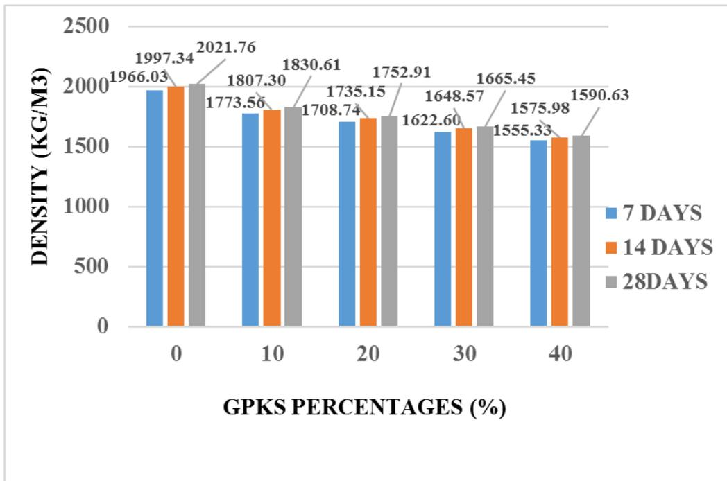
Figure 4.3a, Density of 150mm solid block with sand and GPKS aggregate Type A
