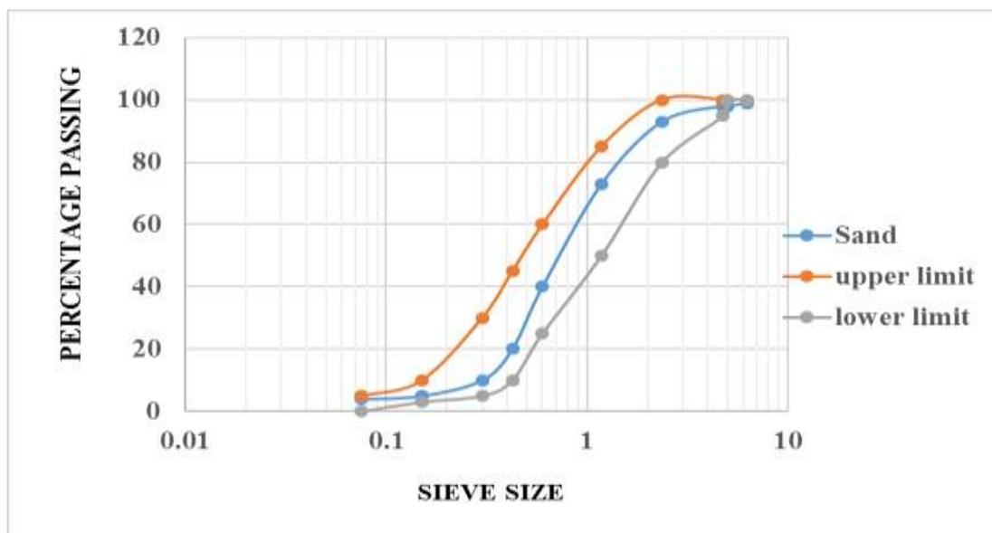
Figure 4.1 Graph of particle size distribution for sand
