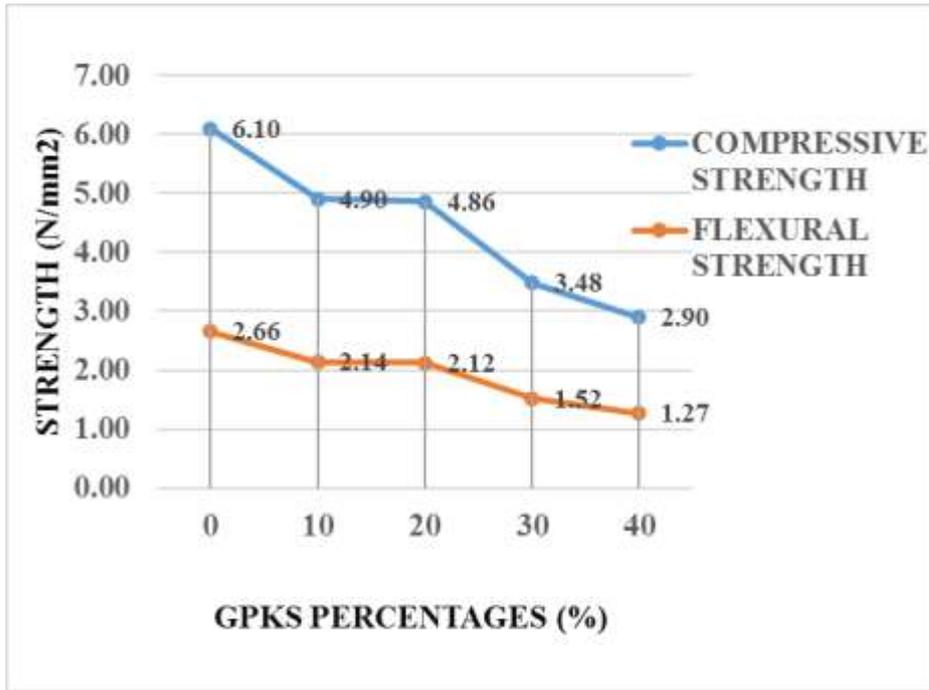
Figure 4.31b, Compressive versus Flexural Strengths (with GPKS aggregate Type B)
