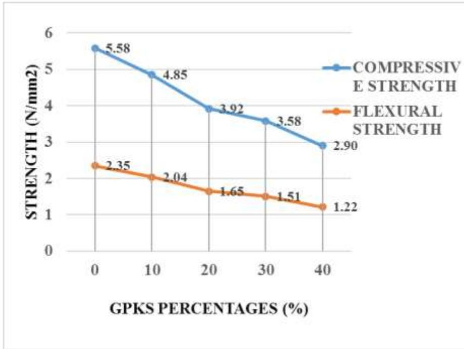
Figure 4.30b, Compressive versus Flexural Strengths (with GPKS aggregate Type B)
