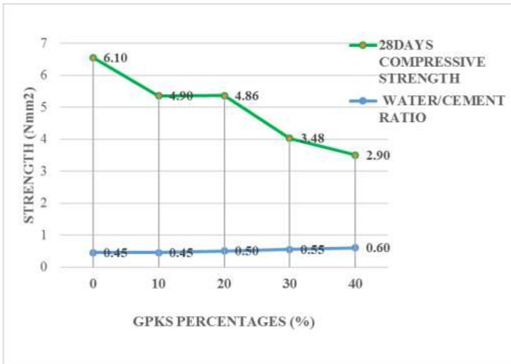
Figure 4.27b, Effect of Water on Strength (125mm cellular block with GPKS aggregate Type B)
