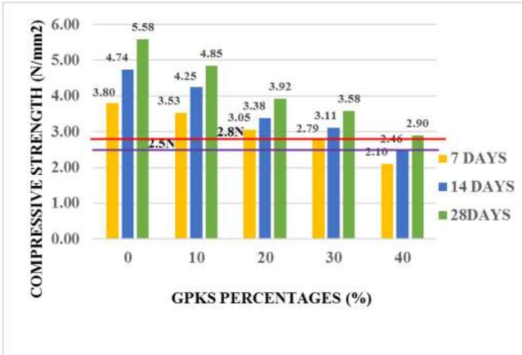
Figure 4.10b, Compressive strength of 150mm cellular block with (GPKS Type B)
