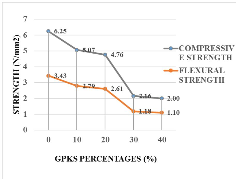
Figure 4.30a, Compressive versus Flexural Strengths (with GPKS aggregate Type A)
