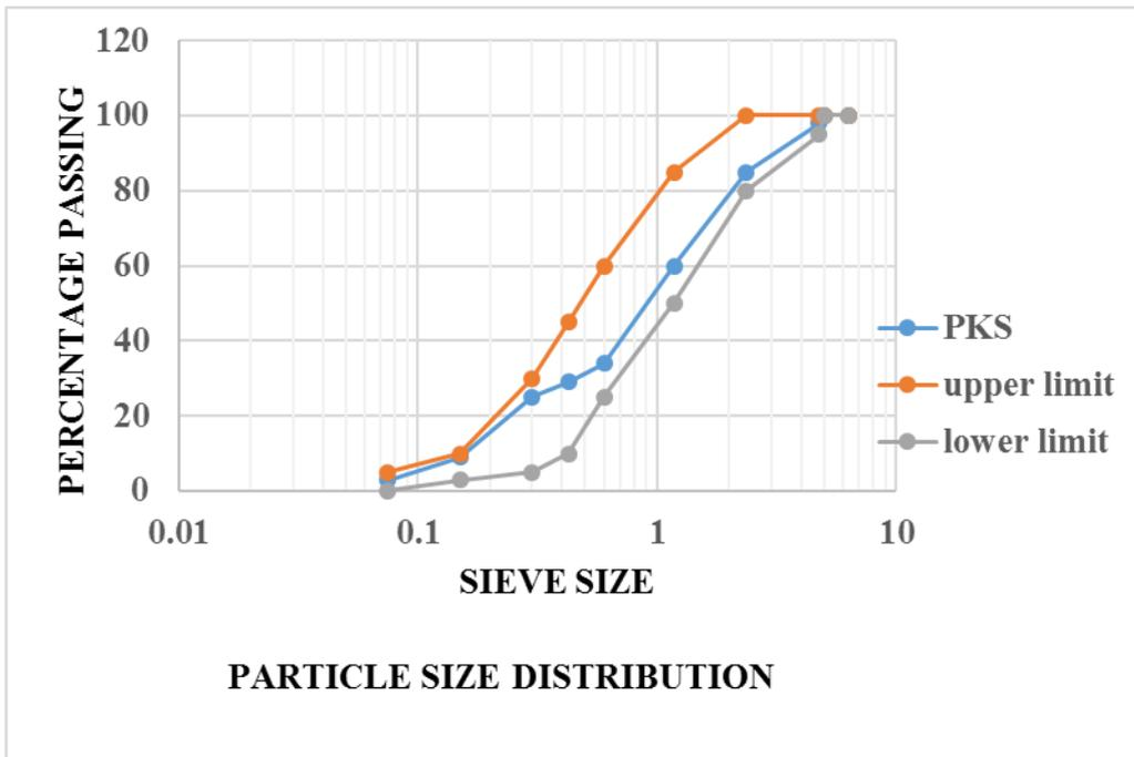
Figure 4.2b, Graph of particle size distribution for GPKS (type B)
