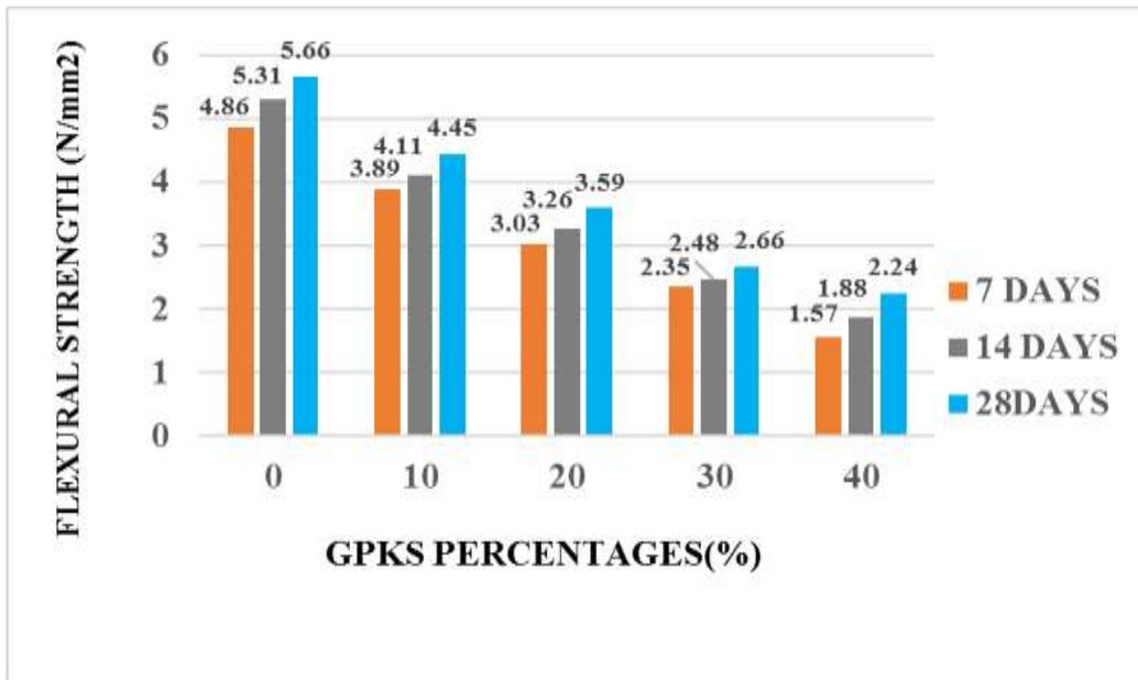
Figure 4.12b, Flexural strength of 150mm solid block with (GPKS Type B)
