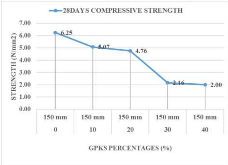
Figure 4.22a, Strength Verses Size of 150mm cellular block with GPKS aggregate Type A
