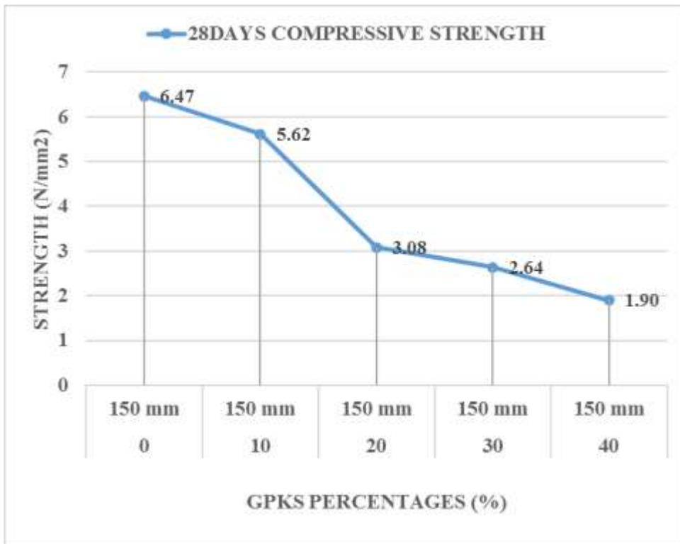
Figure 4.20a, Strength Verses Size of 150mm solid block with GPKS aggregate Type A
