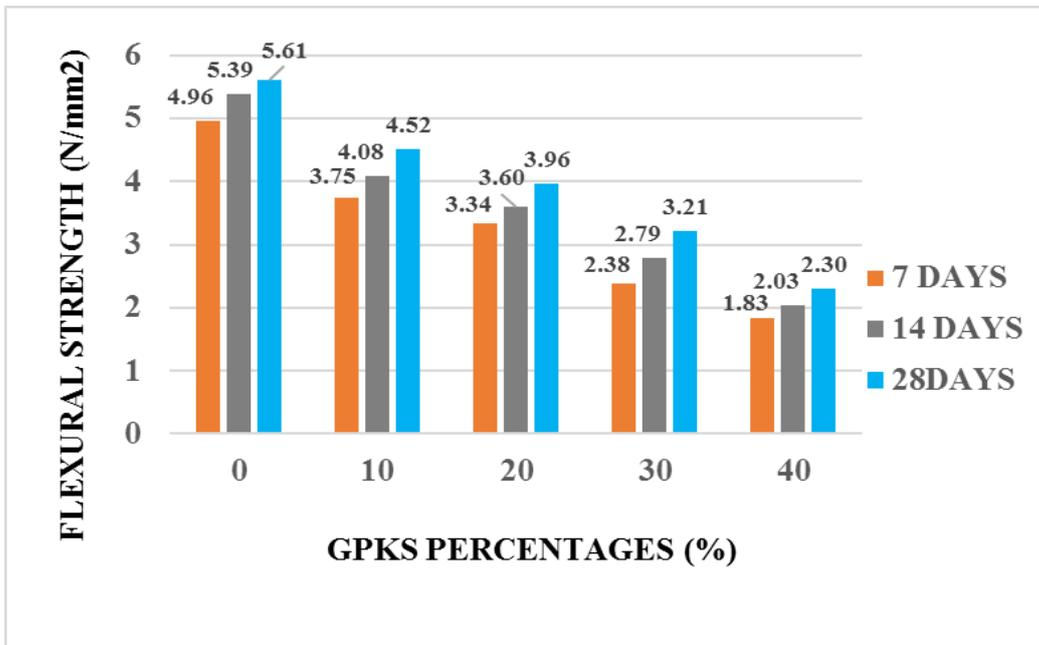
Figure 4.13b, Flexural strength of 125mm solid block with (GPKS Type B)
