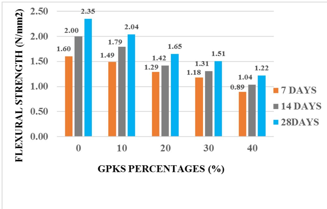
Figure 4.14b, Flexural strength of 150mm cellular block with (GPKS Type B)
