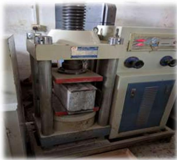
Figure 3.3 Crushing process of the masonry units
