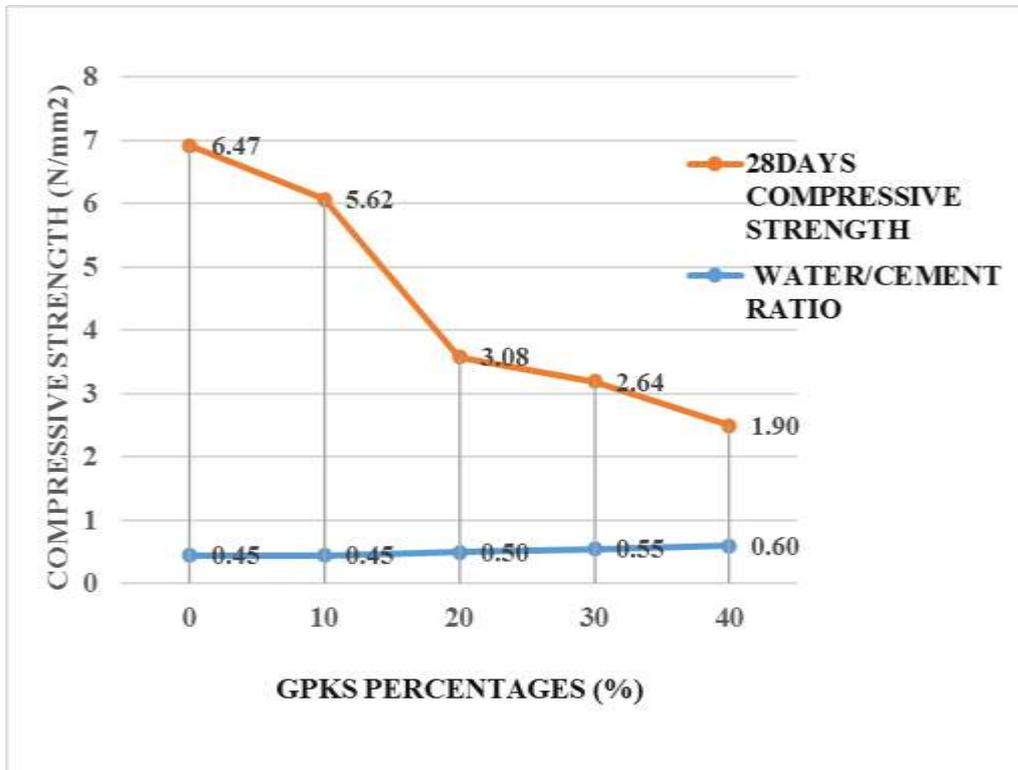
Figure 4.24a, Effect of Water on Strength (150mm solid block with GPKS aggregate Type A)
