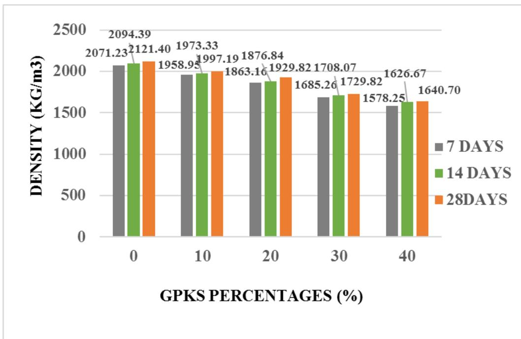
Figure 4.4b, Density of 125mm solid block with sand and GPKS aggregate Type B
