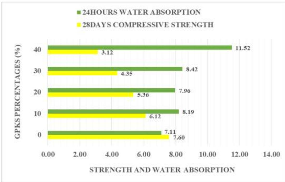
Figure 4.17b, Strength Verses Water absorption of 125mm solid block with GPKS aggregate Type B
