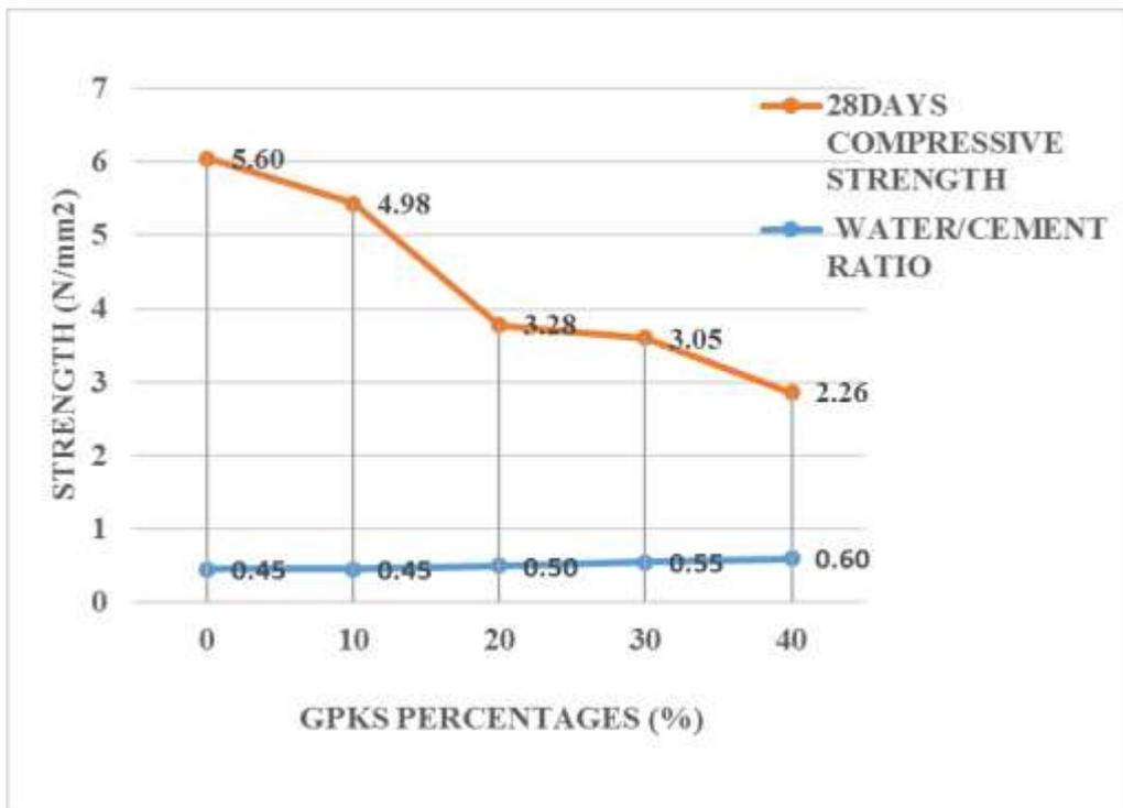
Figure 4.27a, Effect of Water on Strength (125mm cellular block with GPKS aggregate Type A)
