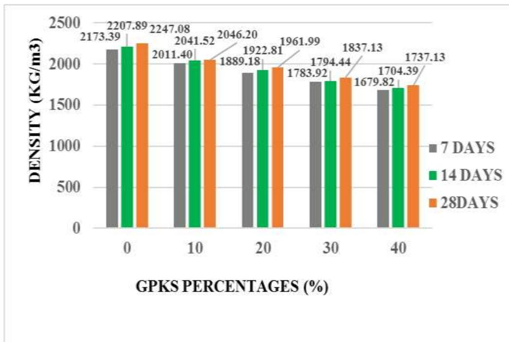
Figure 4.3b, Density of 150mm solid block with sand and GPKS aggregate Type B
