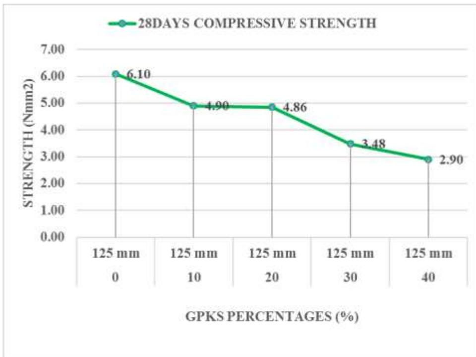
Figure 4.23b, Strength Verses Size of 125mm cellular block with GPKS aggregate Type B
