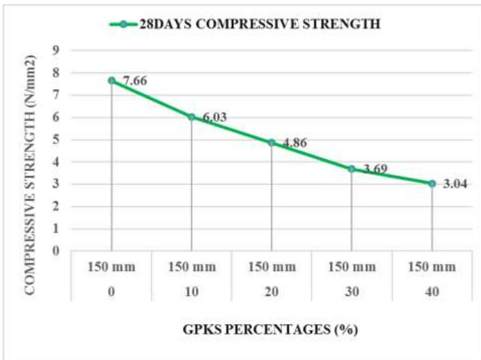
Figure 4.20b, Strength Verses Size of 150mm solid block with GPKS aggregate Type B
