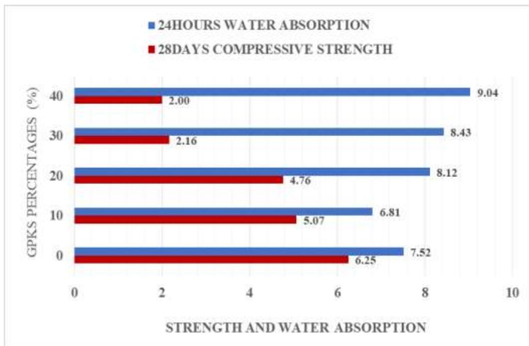
Figure 4.18a, Strength Verses Water absorption of 150mm cellular block with GPKS aggregate Type A
