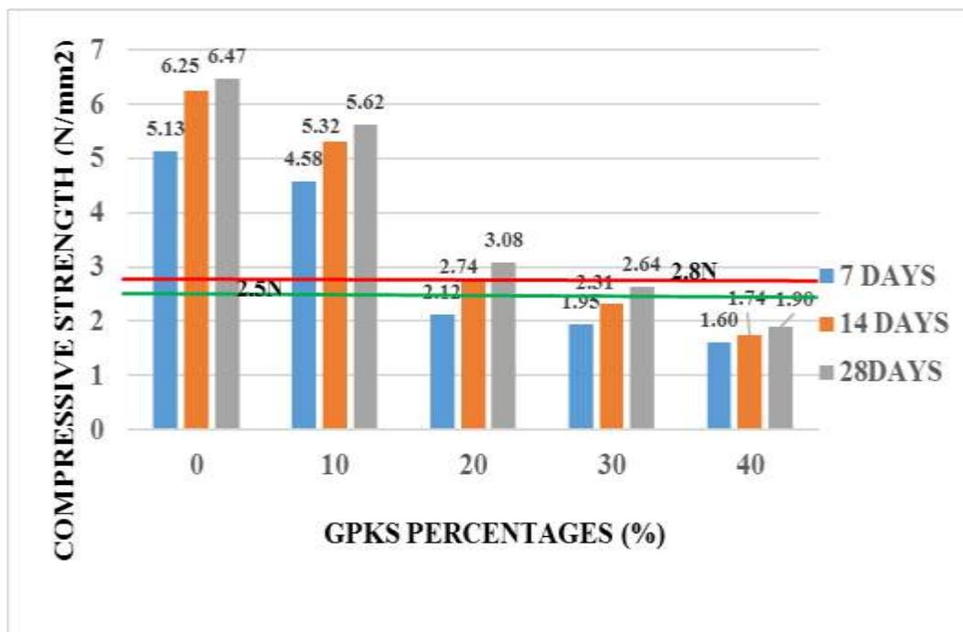
Figure 4.8a, Compressive strength of 150mm solid block with (GPKS Type A)
