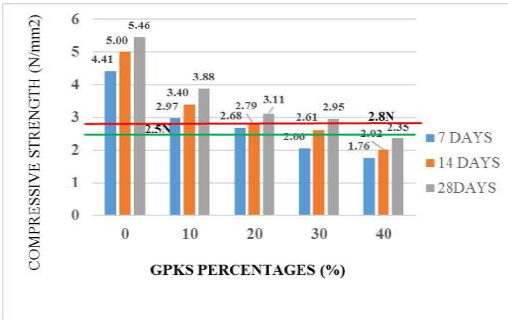
Figure 4.11a, Compressive strength of 125mm cellular block with (GPKS Type A)
