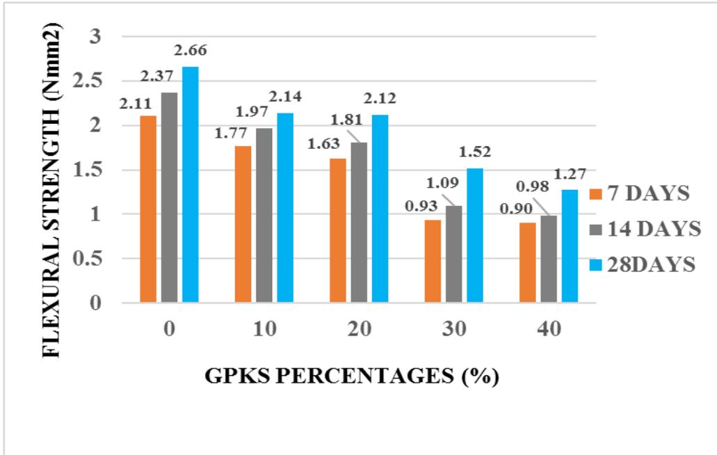
Figure 4.15b, Flexural strength of 125mm cellular block with (GPKS Type B)
