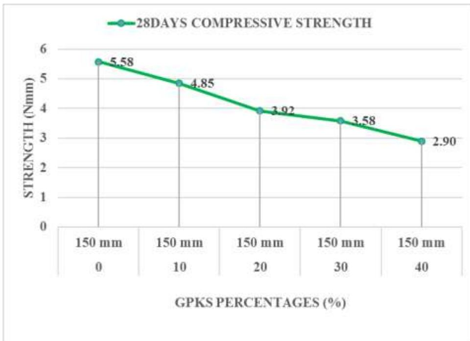
Figure 4.22b, Strength Verses Size of 150mm cellular block with GPKS aggregate Type B
