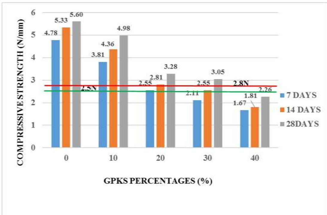
Figure 4.9a, Compressive strength of 125mm solid block with (GPKS Type A)
