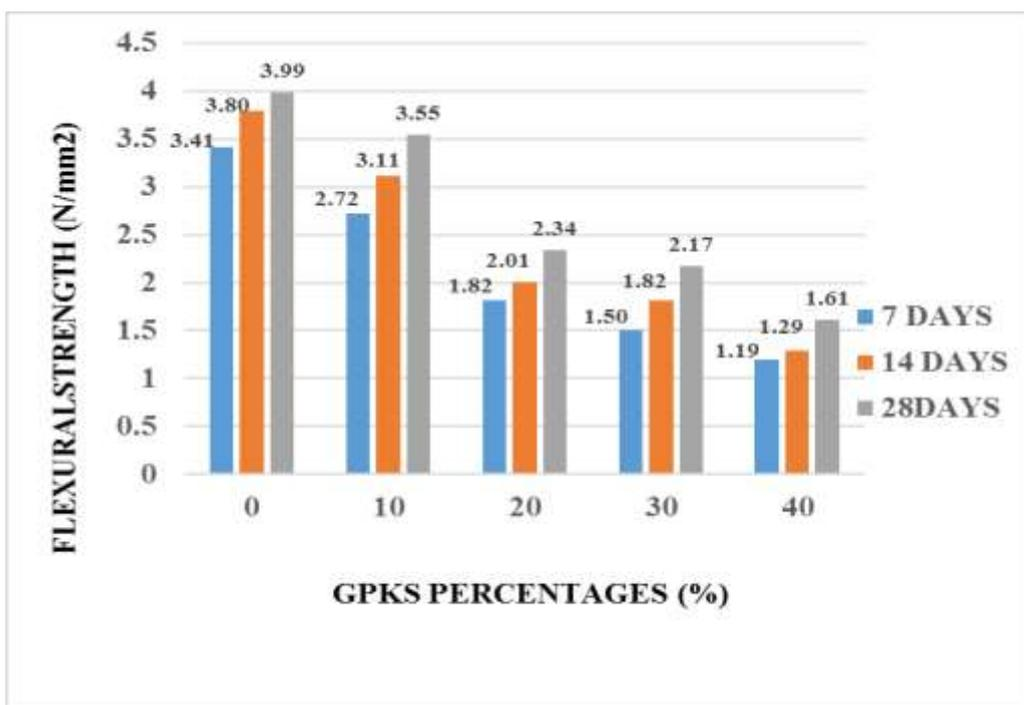
**Figure 4.14a, Flexural strength of 150mm cellular block with (GPKS Type A)**
