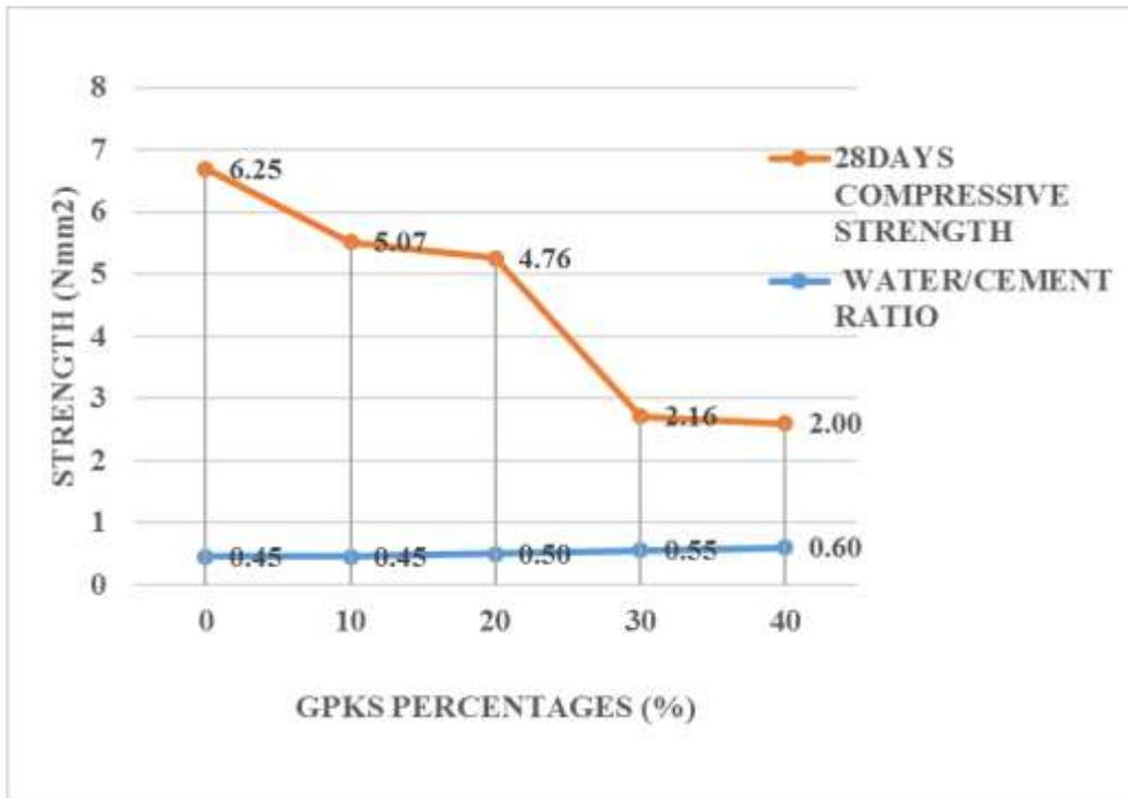
Figure 4.26a, Effect of Water on Strength (150mm cellular block with GPKS aggregate Type A)
