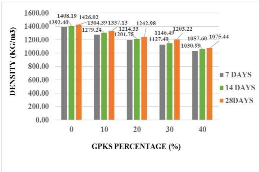
Figure 4.5b, Density of 150mm cellular block with sand and GPKS aggregate Type B
