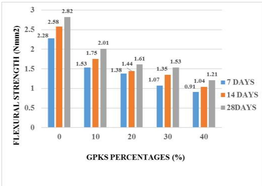
Figure 4.15a, Flexural strength of 125mm cellular block with (GPKS Type A)
