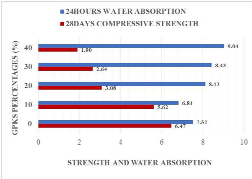
Figure 4.16a, Strength versus Water absorption of 150mm solid block with GPKS aggregate Type A
