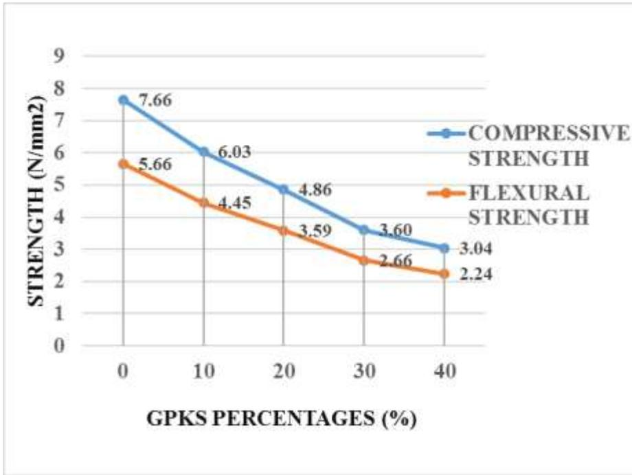
Figure 4.28b, Compressive versus Flexural Strengths (with GPKS aggregate Type B)
