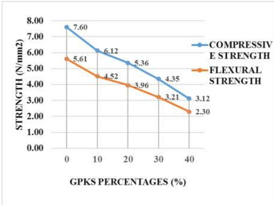
Figure 4.29b, Compressive versus Flexural Strengths (with GPKS aggregate Type B)
