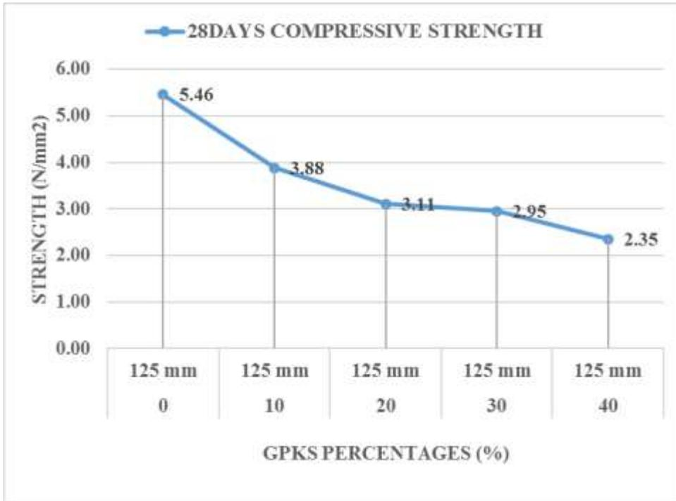
Figure 4.23a, Strength Verses Size of 125mm cellular block with GPKS aggregate Type A
