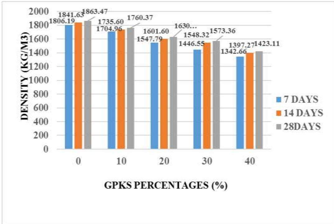
Figure 4.6a, Density of 125mm cellular block with sand and GPKS aggregate Type A
