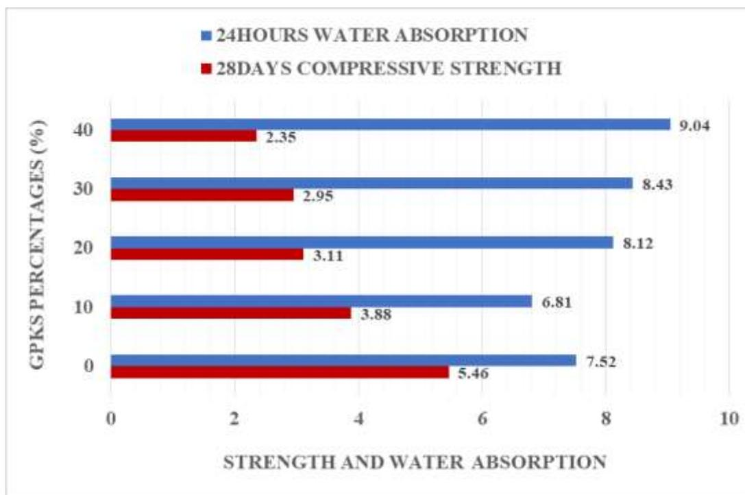
Figure 4.19a, Strength Verses Water absorption of 125mm cellular block with GPKS aggregate Type A
