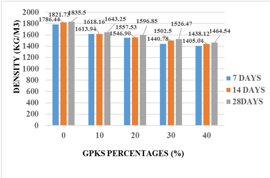
Figure 4.5a, Density of 150mm cellular block with sand and GPKS aggregate Type A
