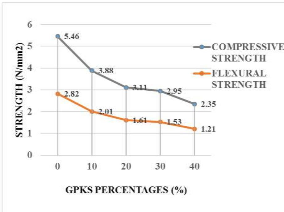
Figure 4.31a, Compressive versus Flexural Strengths (with GPKS aggregate Type A)
