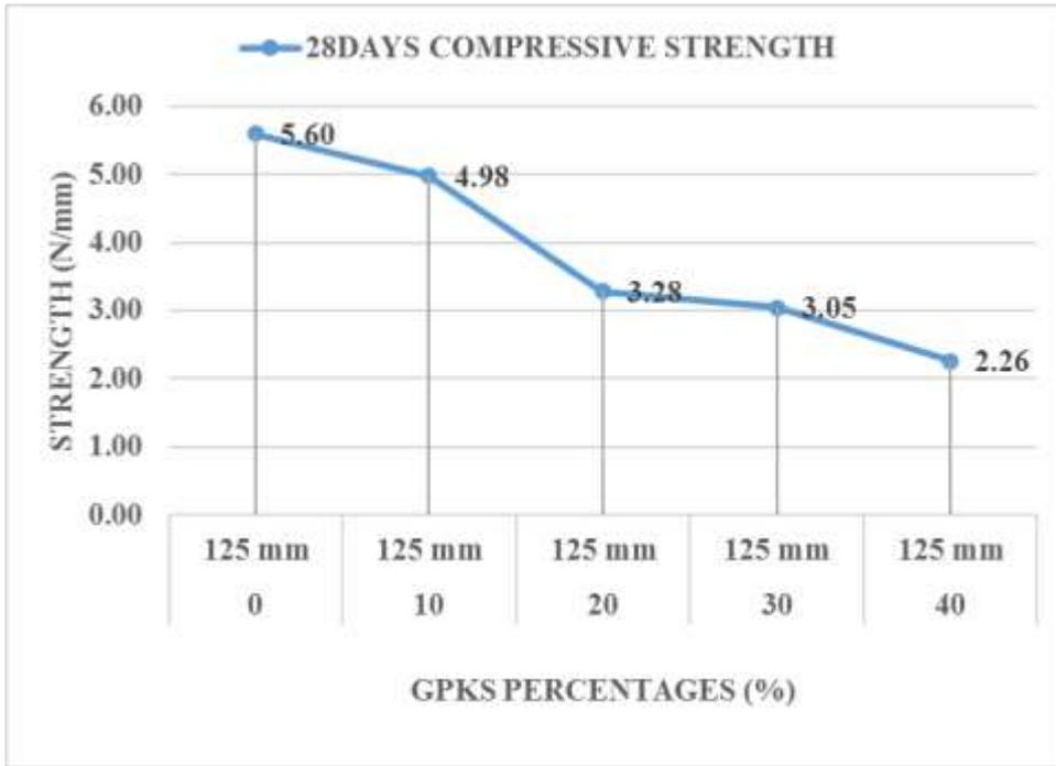
Figure 4.21a, Strength Verses Size of 125mm solid block with GPKS aggregate Type A
