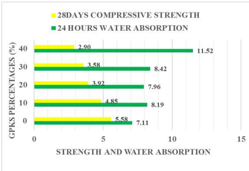
Figure 4.18b, Strength Verses Water absorption of 150mm cellular block with GPKS aggregate Type B
