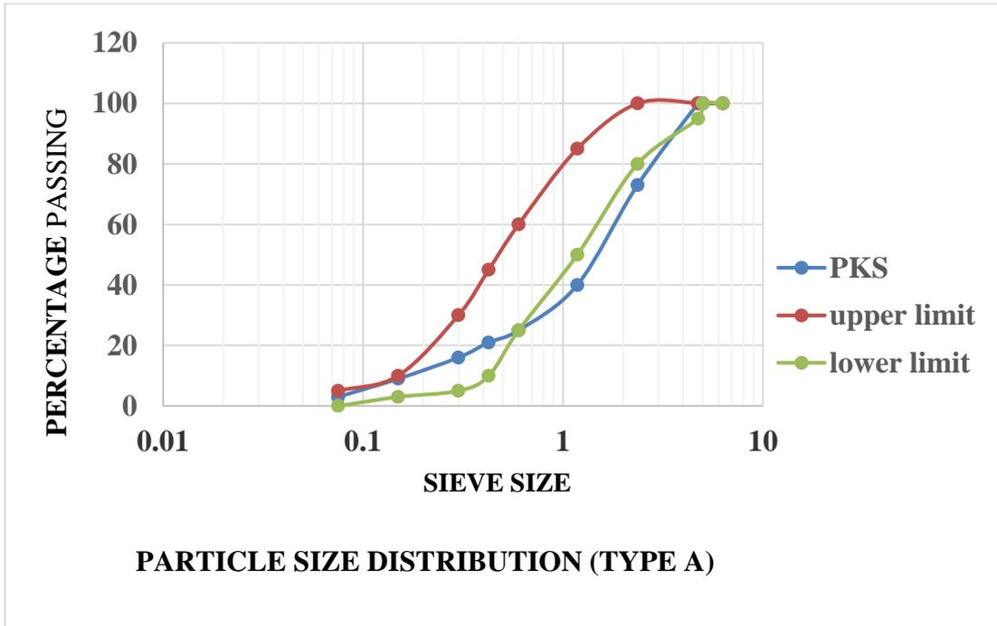
Figure 4.2a, Graph of particle size distribution for GPKS (type A)
