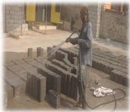
Figure 3.1 Curing and drying process of the masonry units
