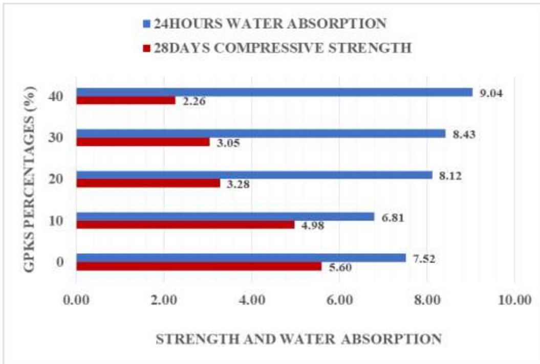
Figure 4.17a, Strength Verses Water absorption of 125mm solid block with GPKS aggregate Type A
