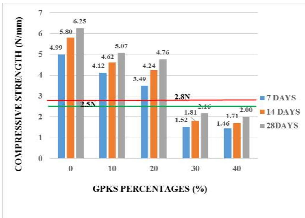
Figure 4.10a, Compressive strength of 150mm cellular block with (GPKS Type A)
