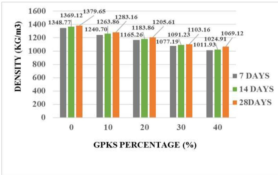
Figure 4.6b, Density of 125mm cellular block with sand and GPKS aggregate Type B
