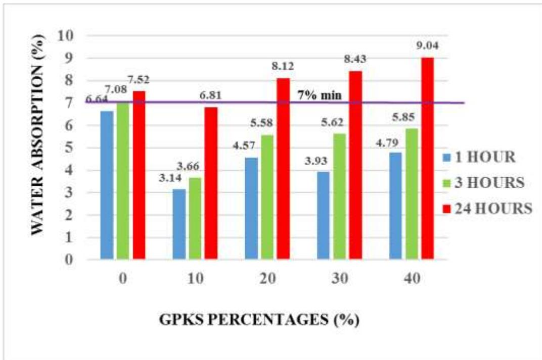
Figure 4.7a Water absorption of cubes produced with GPKS (Type A)
