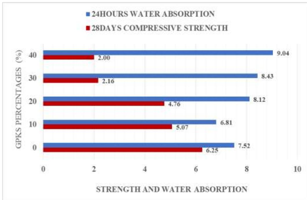
Figure 4.18a, Strength Verses Water absorption of 150mm cellular block with GPKS aggregate Type A
