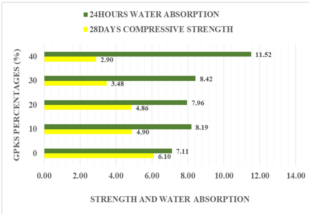
**Figure 4.19b, Strength Verses Water absorption of 125mm cellular block with GPKS aggregate Type B**
